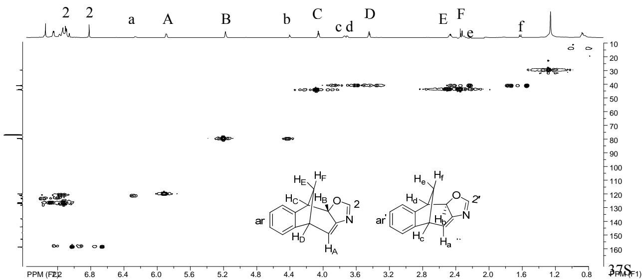
NOESY spectrum of crude mixture after irradiation ( $\text{CDCl}_3$ ) (**8a, 8b**)
