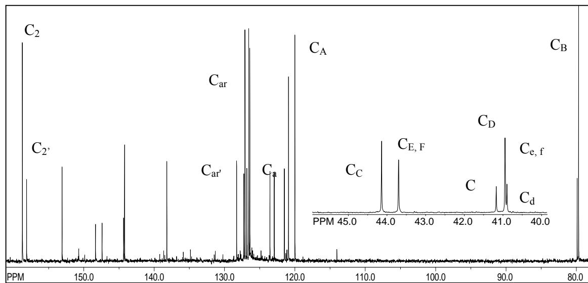
$^{13}\text{C}$  NMR entire range spectrum of crude mixture after irradiation (150 MHz, 3s, 9d, 1t) ( $\text{CDCl}_3$ ) (**8a, 8b**)
