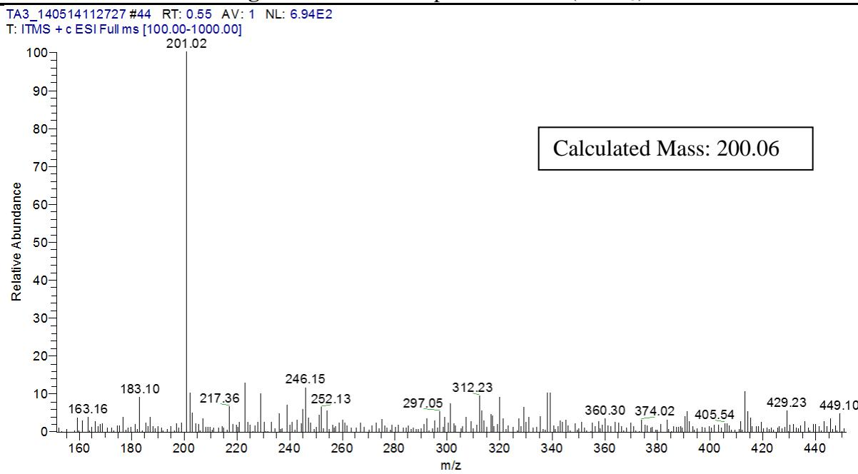
**Figure 84** ESI mass spectrum of Spectrum of **3u**
