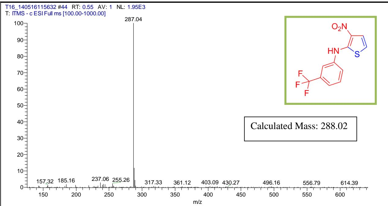
Figure 63 ESI mass spectrum of Spectrum of **3n**
