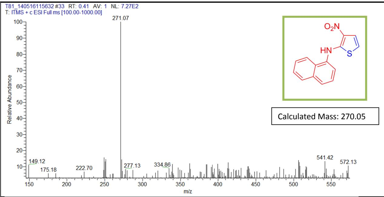
Figure 75 ESI mass spectrum of Spectrum of **3r**
