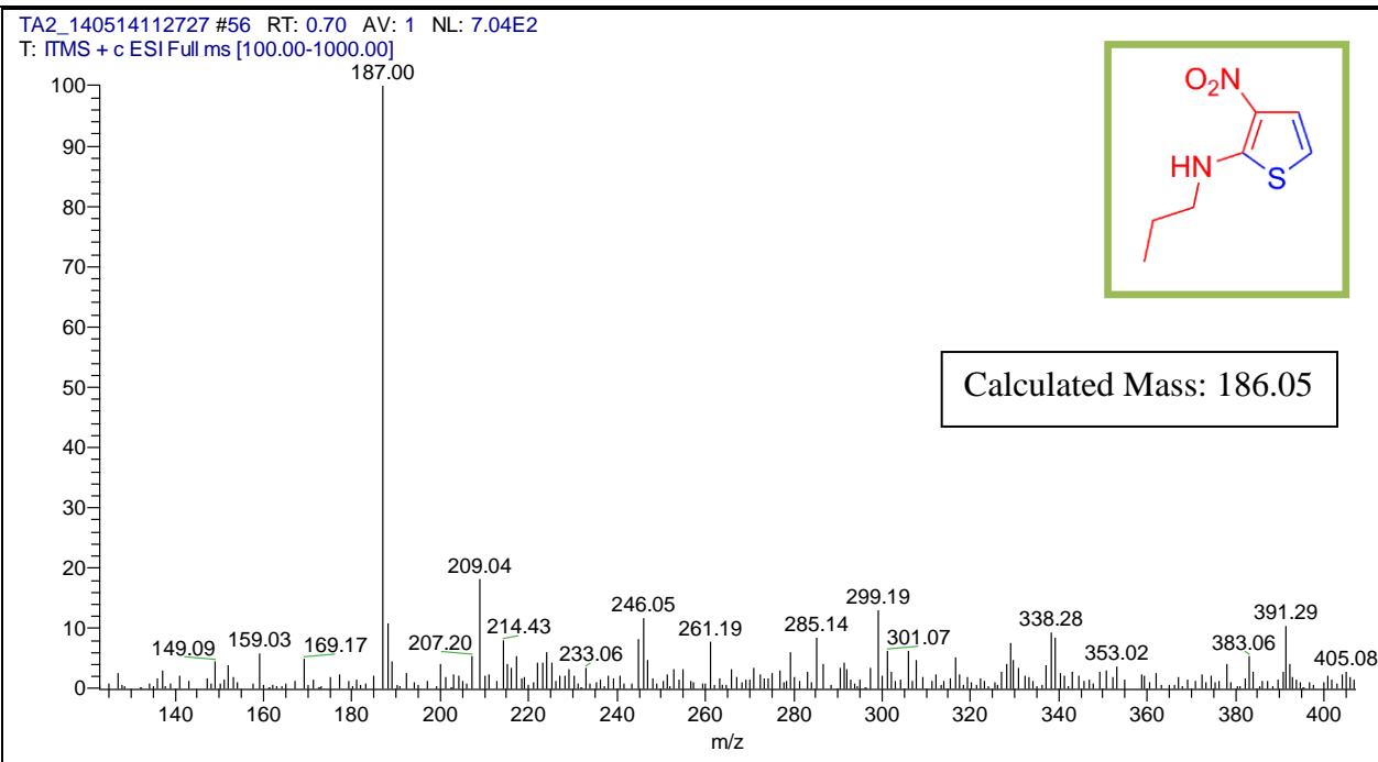
Figure 81 ESI mass spectrum of Spectrum of **3t**
