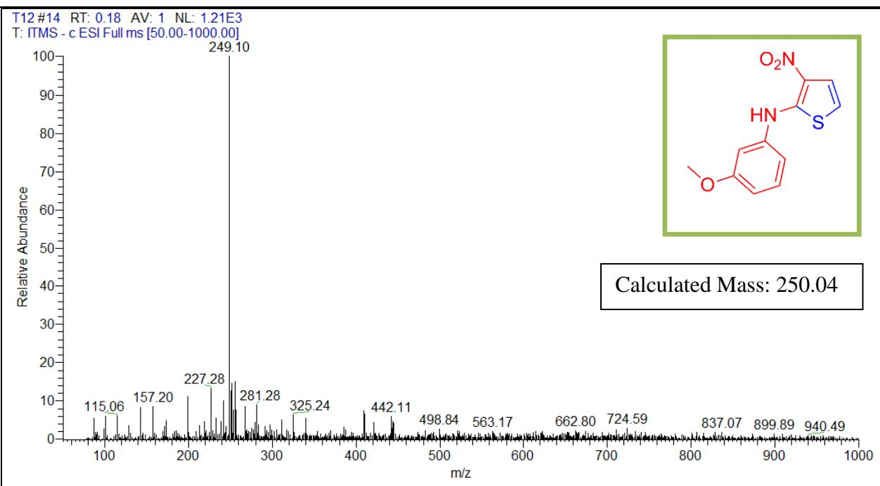
Figure 69 ESI mass spectrum of Spectrum of **3p**
