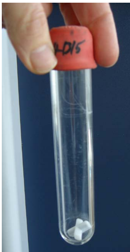
Figure 1: A polymerization tube consisting of a thick-walled test-tube with a septum cap, was used in the preparation of the RAFT copolymers.
