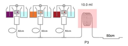
**Reactor setup:** A stock solution of isopropylidenemalononitrile (4) (3 M) in DCM was prepared for pump A (purple), a stock solution of DMF-DMA (4.2 M) and mesitylene (0.3 M) in DCM was prepared for pump B (orange), and a stock solution of acetic anhydride (0.6 M) in DCM was prepared for pump C (red). Each pump was connected to drop tubing (32 cm, 32 cm, and 50 cm respectively), which were connected together before
