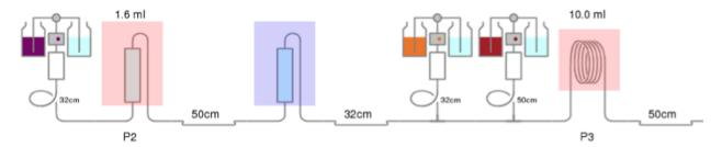
**Reactor setup:** Refer to reactor A setup in section 6 with the following modifications. For pump A, a stock solution of acetone (0.5 M) and malononitrile (0.5 M) was used. The  $Al_2O_3$  column was heated to 95 °C.
