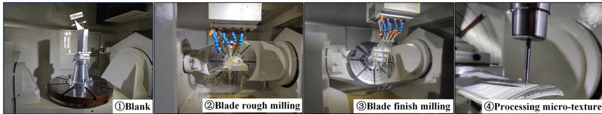
**Figure 7:** The manufacturing procedure of the microtextured blade.
