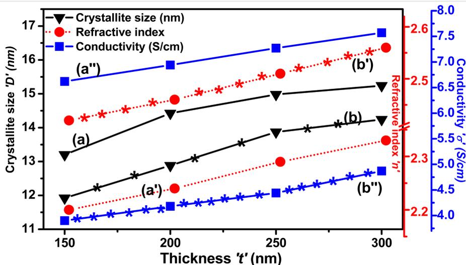
**Figure 12:** Mutual correlation between (a, b) crystallite size, (a', b') refractive index, and (a'', b'') conductivity and thickness of the Mo films. (a), (a') and (a'') stand for as-deposited and (b), (b)', and (b'') stand for  $N_2^+$ -implanted Mo thin films.
