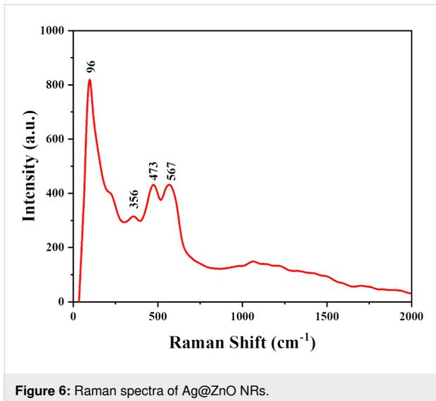
Figure 6: Raman spectra of Ag@ZnO NRs.
