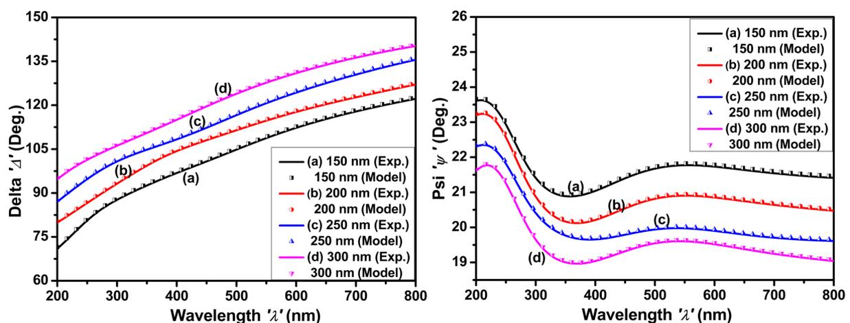
**Figure 6:** Measured SE data (solid line) and fit (symbols) of  $\psi$  and  $\Delta$  spectra as functions of the wavelength of  $N_2^+$ -implanted molybdenum thin films with thicknesses of (a) 150 nm, (b) 200 nm, (c) 250 nm, and (d) 300 nm.
