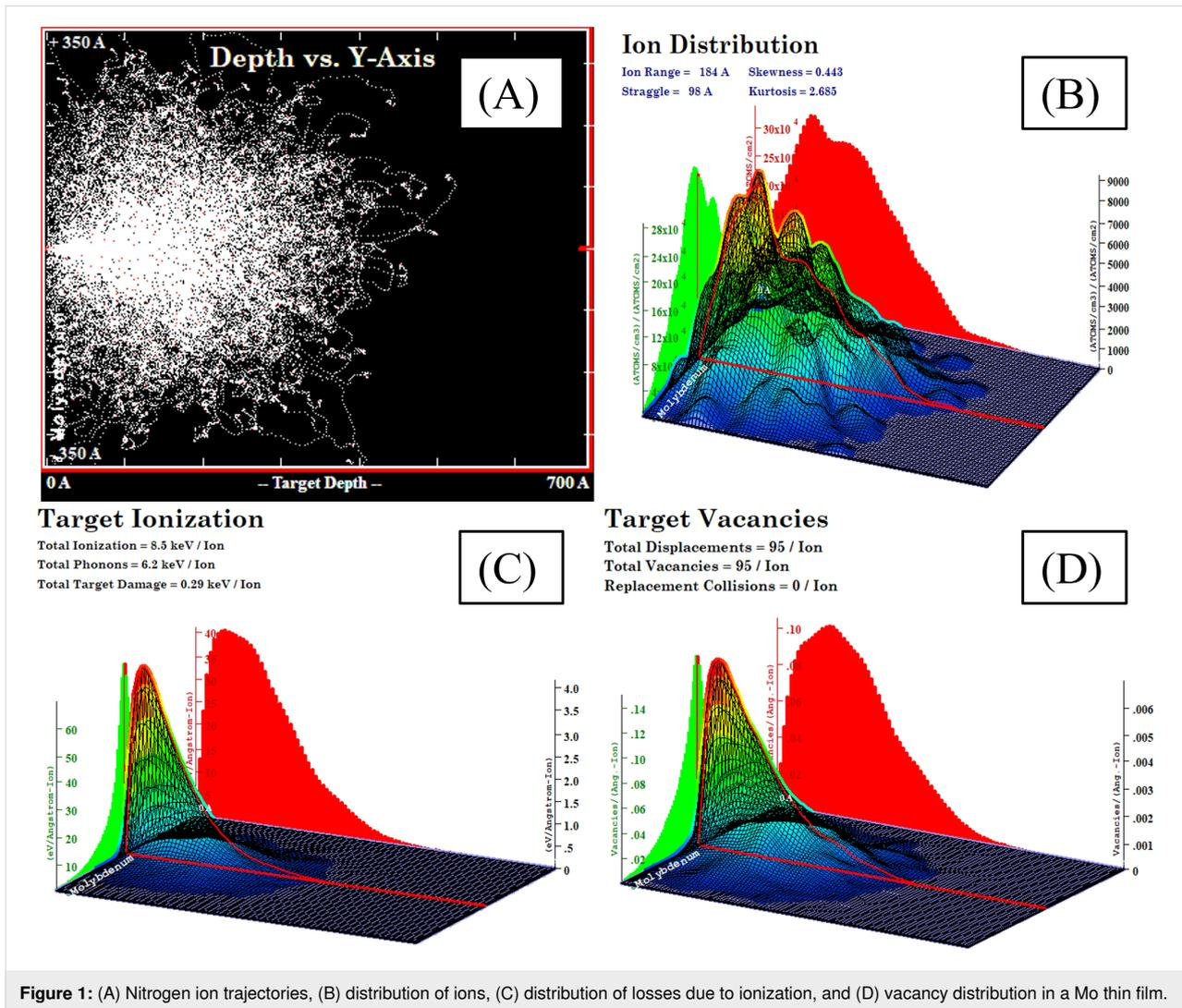
**Figure 1:** (A) Nitrogen ion trajectories, (B) distribution of ions, (C) distribution of losses due to ionization, and (D) vacancy distribution in a Mo thin film.
