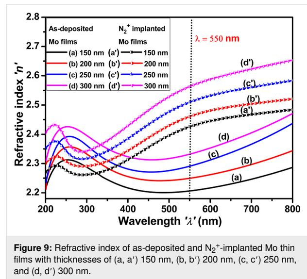
**Figure 9:** Refractive index of as-deposited and  $N_2^+$ -implanted Mo thin films with thicknesses of (a, a') 150 nm, (b, b') 200 nm, (c, c') 250 nm, and (d, d') 300 nm.
