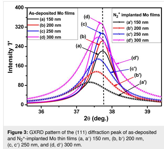
**Figure 3:** GXRD pattern of the (111) diffraction peak of as-deposited and  $\text{N}_2^+$ -implanted Mo thin films (a, a') 150 nm, (b, b') 200 nm, (c, c') 250 nm, and (d, d') 300 nm.
