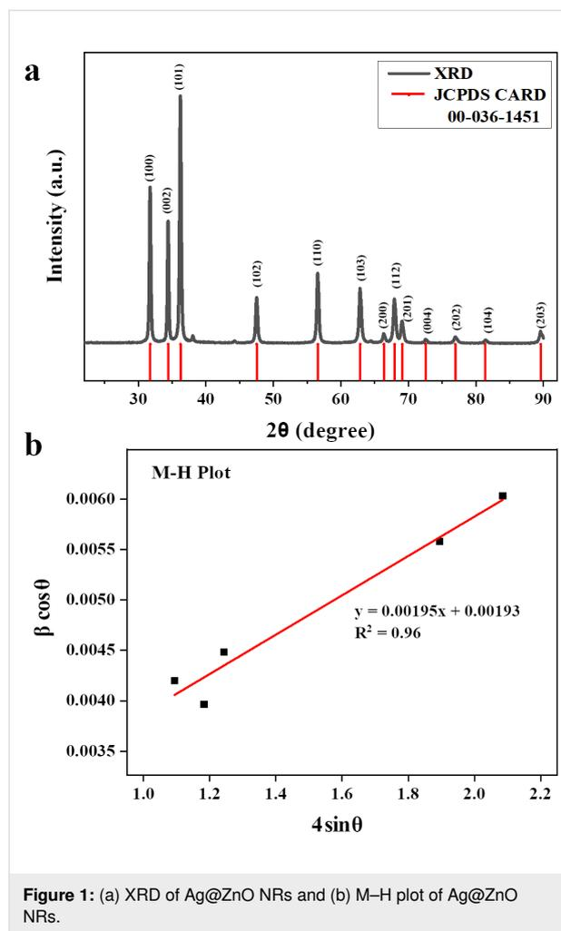
**Figure 1:** (a) XRD of Ag@ZnO NRs and (b) M–H plot of Ag@ZnO NRs.
