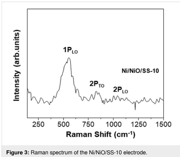
Figure 3: Raman spectrum of the Ni/NiO/SS-10 electrode.
