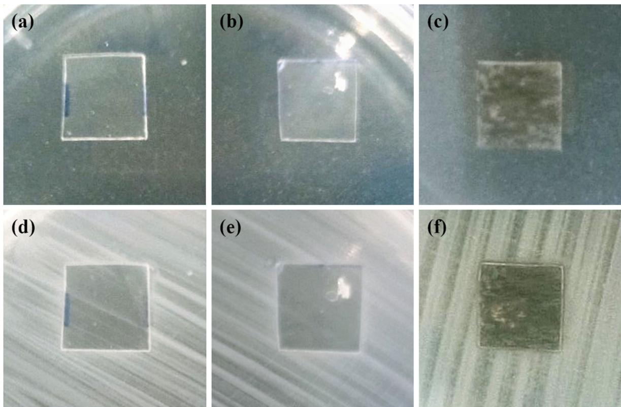
**Figure 10:** Antibacterial test of uncoated and coated PLA films against the growth of *E. coli* biofilm. (a, b, c) Pictures of a PLA film (a), an SG/PLA film (b), and a GO-SG-ZH/PLA film (c) on agar plates inoculated with *E. coli* bacteria (before incubation). (d, e, f) Pictures of the PLA film (d), SG/PLA film (e), and GO-SG-ZH/PLA film (f) on the agar/biofilm plates after incubation at 37 °C for 24 h.
