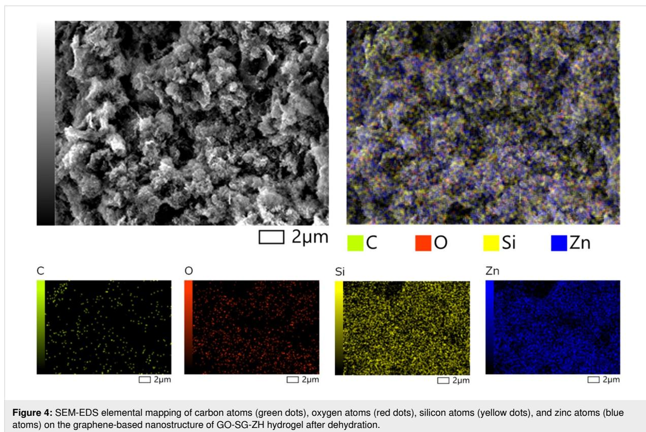
**Figure 4:** SEM-EDS elemental mapping of carbon atoms (green dots), oxygen atoms (red dots), silicon atoms (yellow dots), and zinc atoms (blue atoms) on the graphene-based nanostructure of GO-SG-ZH hydrogel after dehydration.
