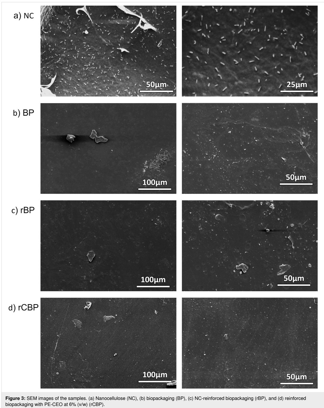
**Figure 3:** SEM images of the samples. (a) Nanocellulose (NC), (b) biopackaging (BP), (c) NC-reinforced biopackaging (rBP), and (d) reinforced biopackaging with PE-CEO at 6% (v/w) (rCBP).
