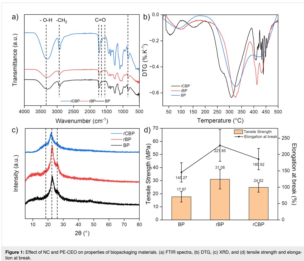
**Figure 1:** Effect of NC and PE-CEO on properties of biopackaging materials. (a) FTIR spectra, (b) DTG, (c) XRD, and (d) tensile strength and elongation at break.
