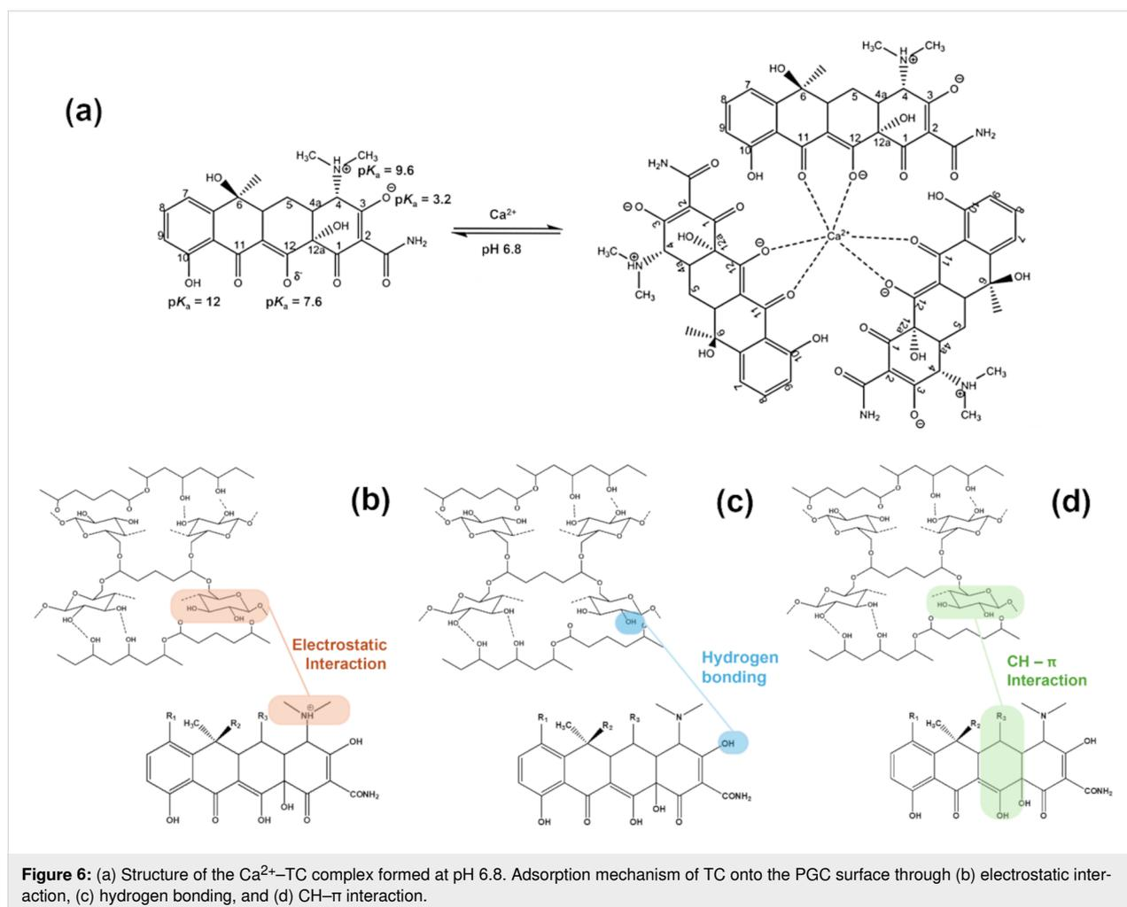
**Figure 6:** (a) Structure of the  $\text{Ca}^{2+}$ -TC complex formed at pH 6.8. Adsorption mechanism of TC onto the PGC surface through (b) electrostatic interaction, (c) hydrogen bonding, and (d) CH- $\pi$  interaction.
