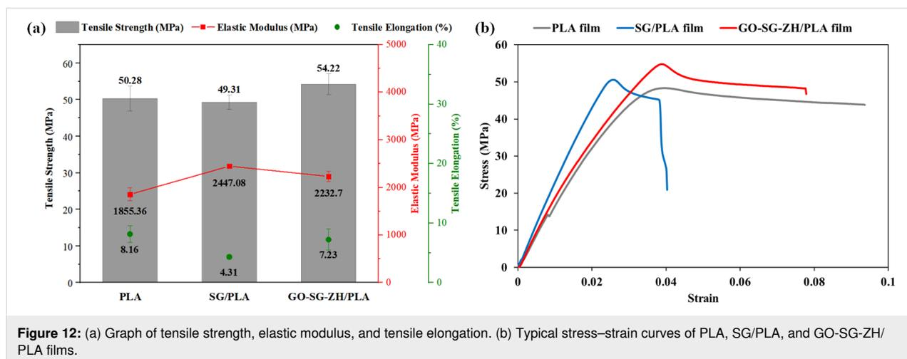
**Figure 12:** (a) Graph of tensile strength, elastic modulus, and tensile elongation. (b) Typical stress–strain curves of PLA, SG/PLA, and GO-SG-ZH/PLA films.
