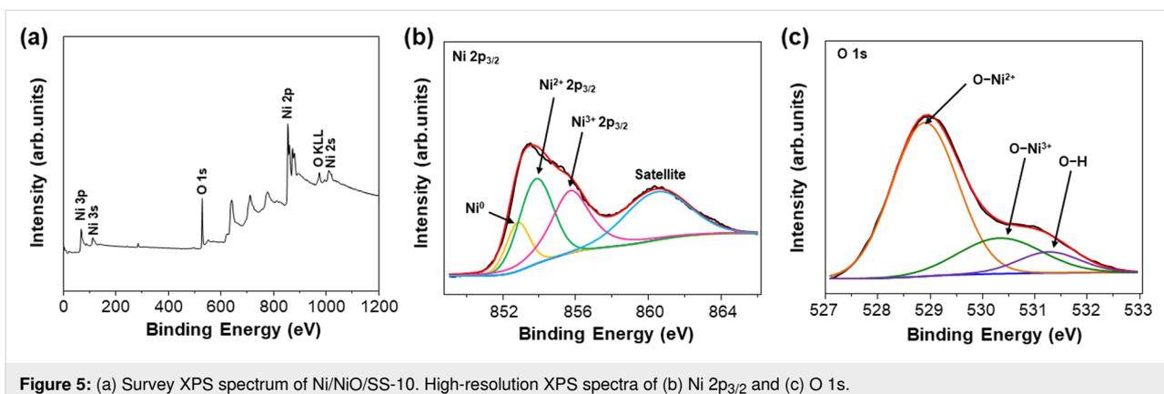
Figure 5: (a) Survey XPS spectrum of Ni/NiO/SS-10. High-resolution XPS spectra of (b) Ni  $2p_{3/2}$  and (c) O 1s.
