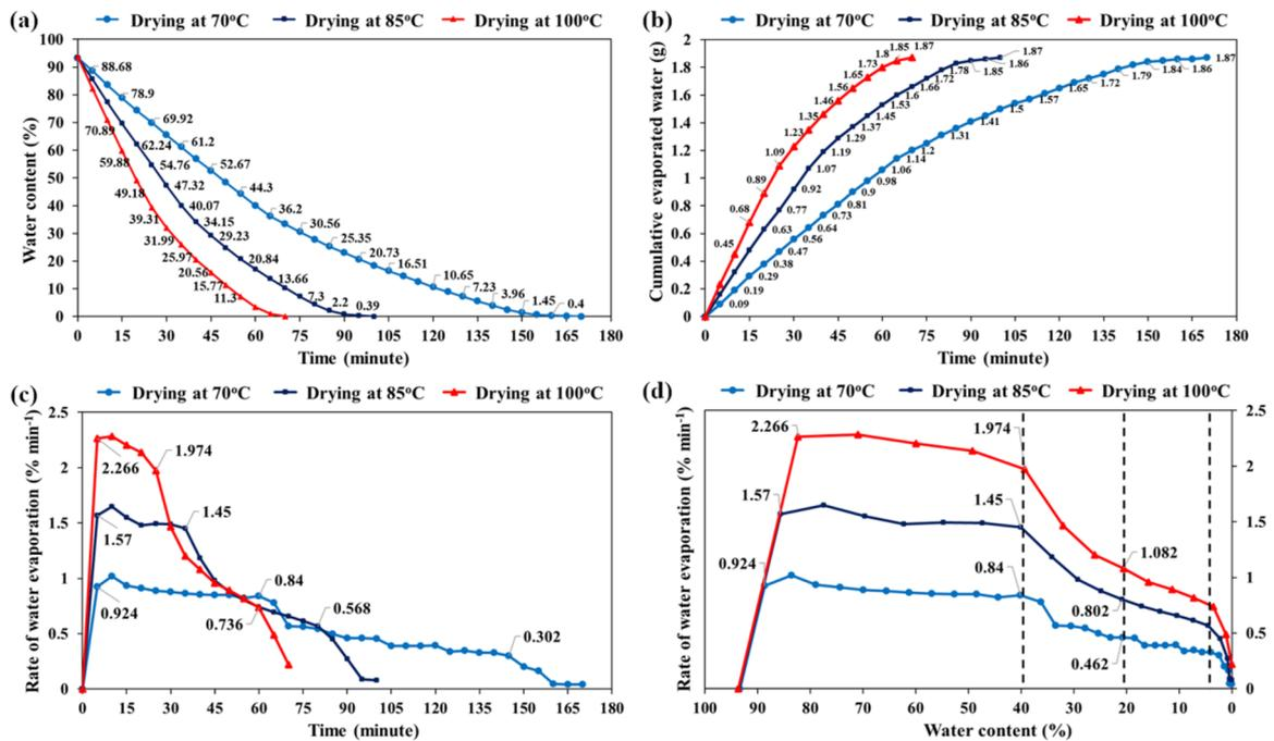
**Figure 5:** Analysis of moisture content and water evaporation of GO-SG-ZH hydrogel. (a) Curves of changing moistures of GO-SG-ZH hydrogel at different drying temperatures (70, 85, and 100 °C). (b) Curves of cumulative amount of evaporated water during drying at 70, 85, and 100 °C. (c) Plot of water evaporation rates with respect to drying time. (d) Plot of water evaporation rates with respect to water content in GO-SG-ZH hydrogel.
