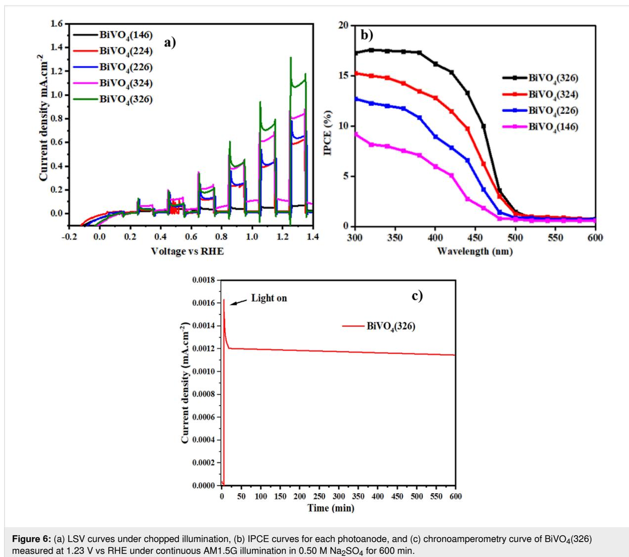
**Figure 6:** (a) LSV curves under chopped illumination, (b) IPCE curves for each photoanode, and (c) chronoamperometry curve of  $\text{BiVO}_4(326)$  measured at 1.23 V vs RHE under continuous AM1.5G illumination in 0.50 M  $\text{Na}_2\text{SO}_4$  for 600 min.
