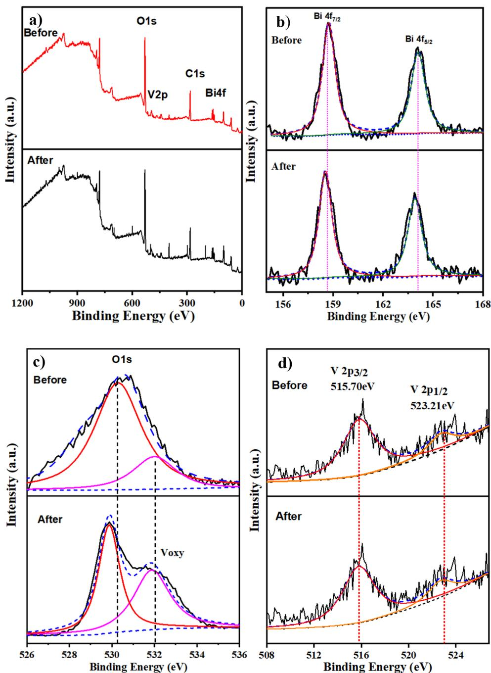
**Figure 7:** X-ray photoelectron spectroscopy (XPS) analysis of the  $\text{BiVO}_4(326)$  photoanode before and after PEC stability testing in 30 min (0.5 M  $\text{Na}_2\text{SO}_4$ ). (a) XPS view scans of survey spectrum and high-resolution spectra of (b) Bi 4f, (c) O 1s, and (d) V 2p.
