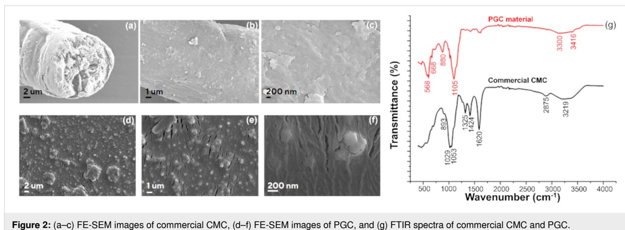
**Figure 2:** (a–c) FE-SEM images of commercial CMC, (d–f) FE-SEM images of PGC, and (g) FTIR spectra of commercial CMC and PGC.
