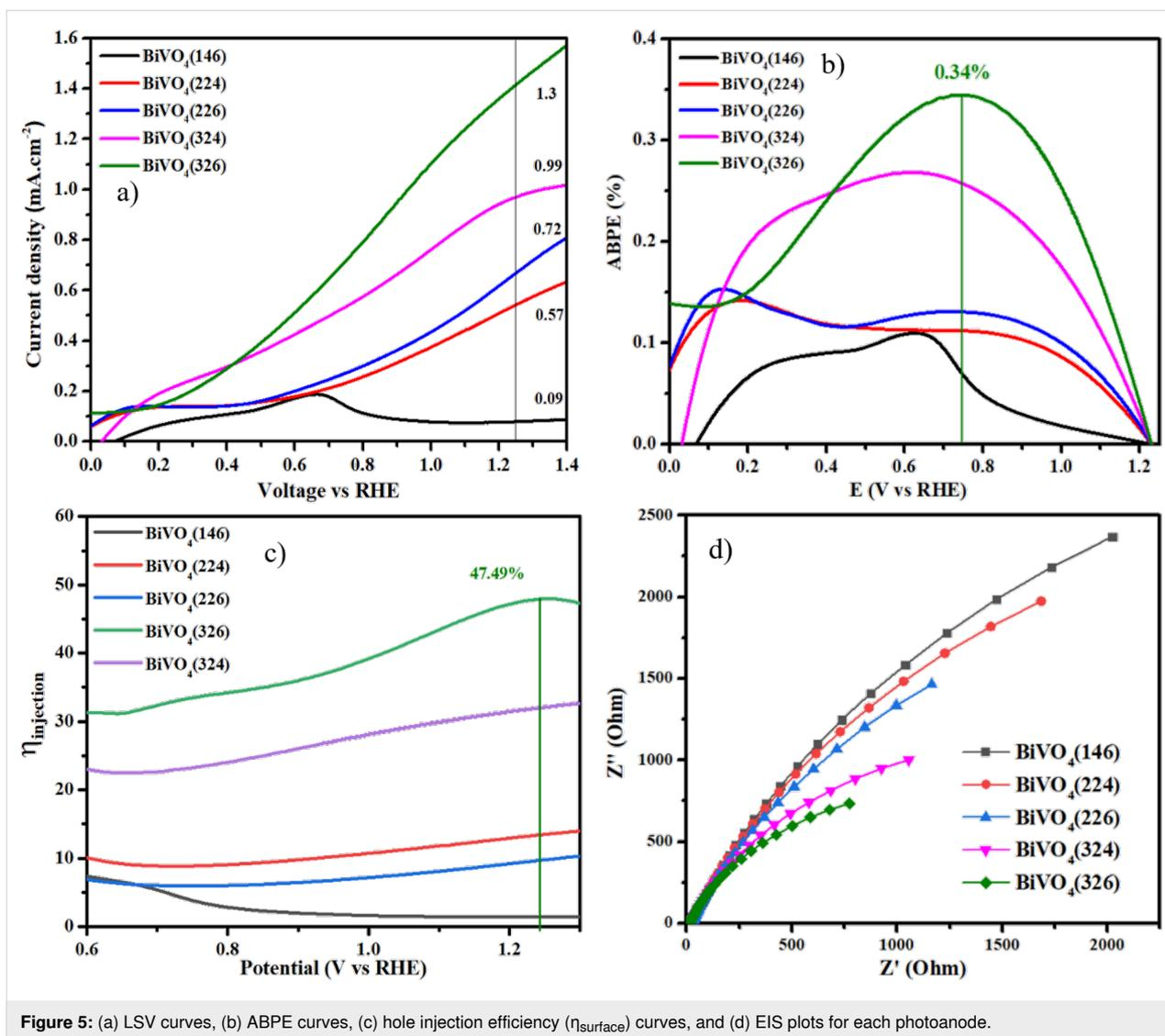
**Figure 5:** (a) LSV curves, (b) ABPE curves, (c) hole injection efficiency ( $\eta_{\text{surface}}$ ) curves, and (d) EIS plots for each photoanode.
