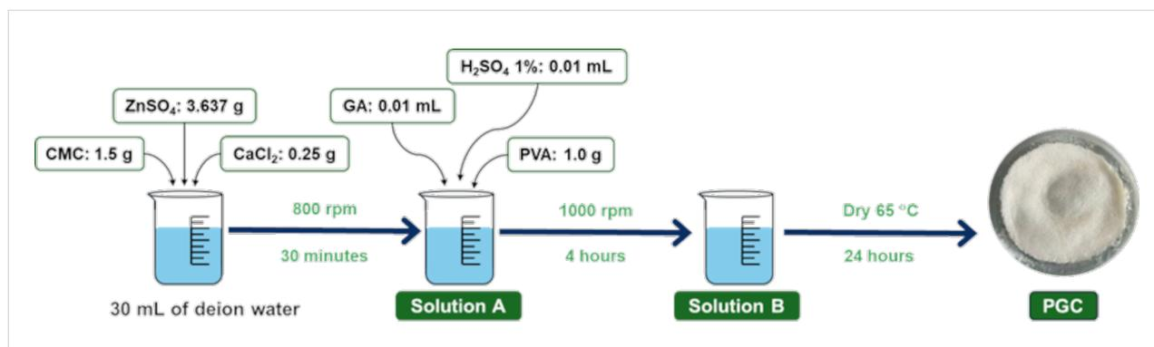
**Figure 7:** Synthesis procedure for PGC.
