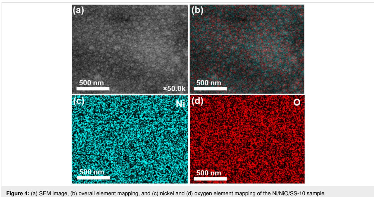
Figure 4: (a) SEM image, (b) overall element mapping, and (c) nickel and (d) oxygen element mapping of the Ni/NiO/SS-10 sample.
