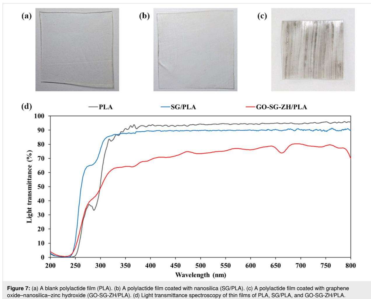
**Figure 7:** (a) A blank poly(lactide) film (PLA). (b) A poly(lactide) film coated with nanosilica (SG/PLA). (c) A poly(lactide) film coated with graphene oxide–nanosilica–zinc hydroxide (GO-SG-ZH/PLA). (d) Light transmittance spectroscopy of thin films of PLA, SG/PLA, and GO-SG-ZH/PLA.
