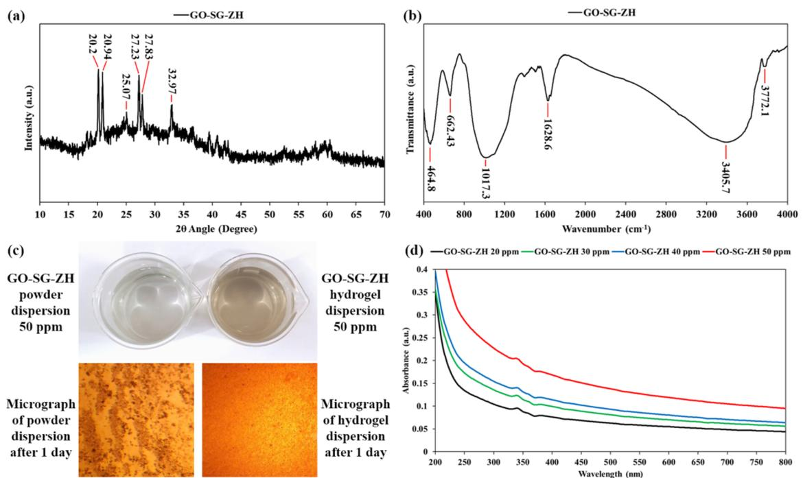
**Figure 6:** (a) XRD pattern of GO-SG-ZH powder. (b) FTIR spectrum of GO-SG-ZH powder. (c) Aqueous dispersions of GO-SG-ZH powder and hydrogel (concentrations of 50 ppm) and their sedimented particles after 1 day (visualized by the optical microscope). (d) UV-vis spectra of aqueous dispersions of GO-SG-ZH hydrogel.
