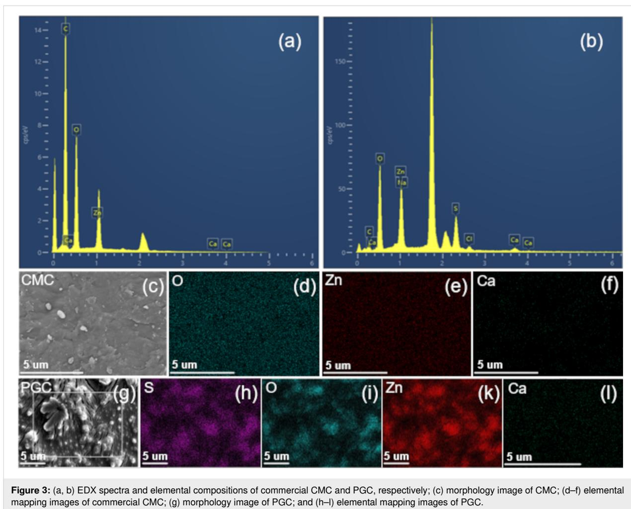
**Figure 3:** (a, b) EDX spectra and elemental compositions of commercial CMC and PGC, respectively; (c) morphology image of CMC; (d–f) elemental mapping images of commercial CMC; (g) morphology image of PGC; and (h–l) elemental mapping images of PGC.
