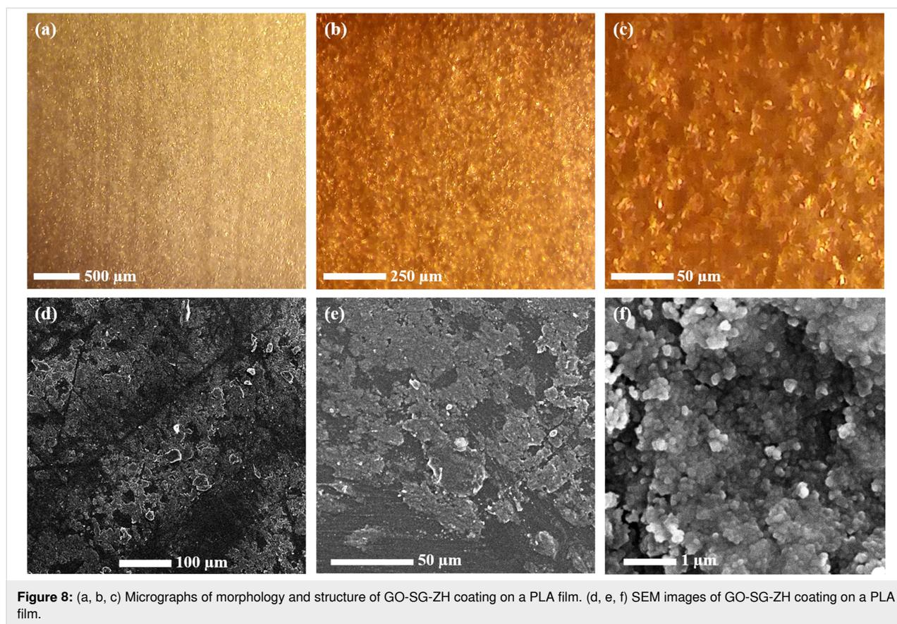
**Figure 8:** (a, b, c) Micrographs of morphology and structure of GO-SG-ZH coating on a PLA film. (d, e, f) SEM images of GO-SG-ZH coating on a PLA film.
