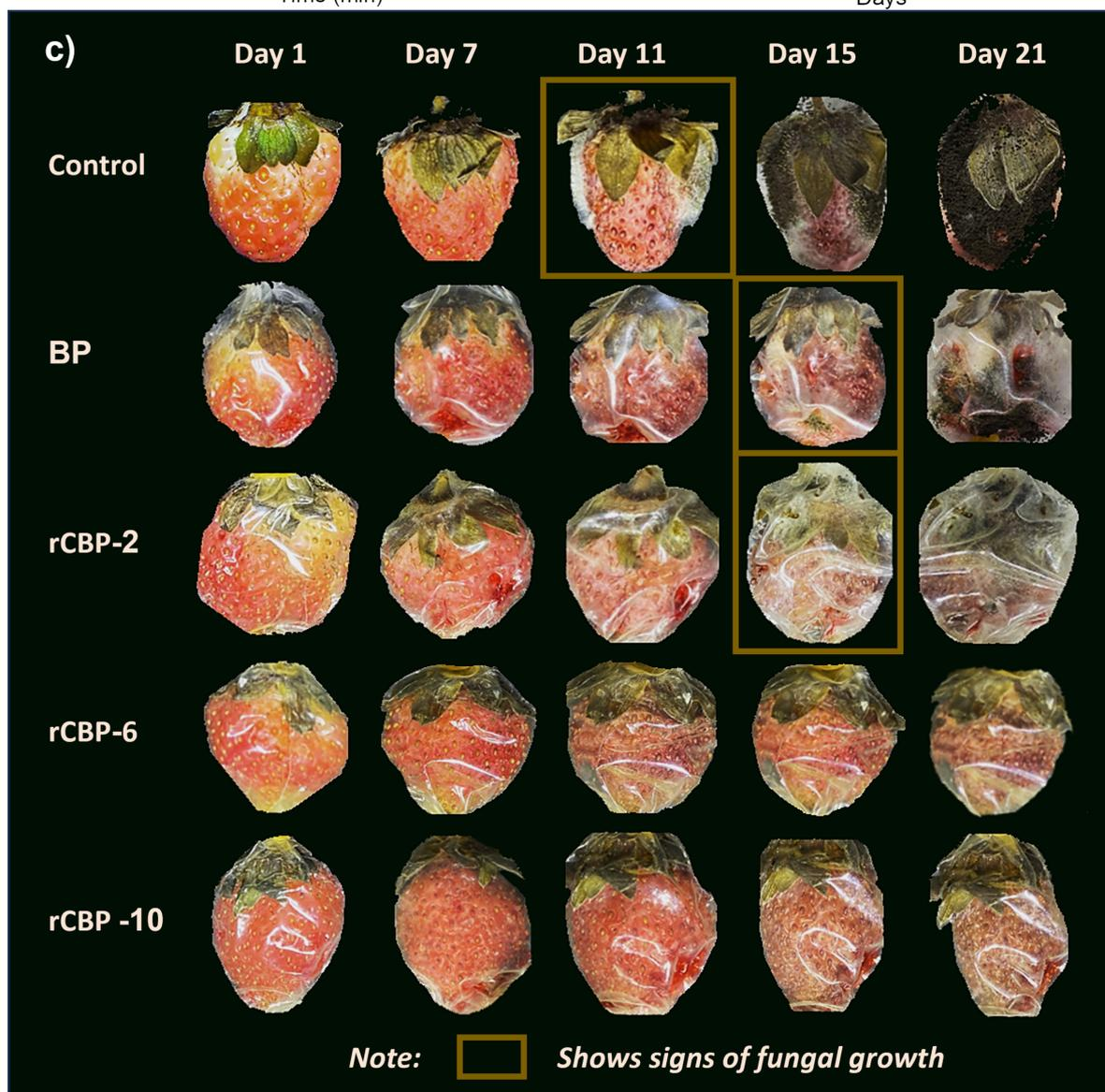
**Figure 5:** Results on strawberry preservation. (a) Release profile of CEO from rCBP-10, (b) mass loss record by days, and (c) appearance of the fruits after 1, 7, 11, 15, and 21 days of preservation for control (commercial PVC), BP, and reinforced biopackaging with PE-CEO (rCBP) at different concentrations (2%, 6%, and 10% (v/w)).
