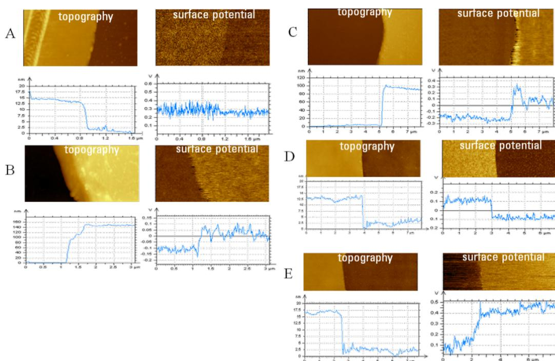
**Figure 7:** Topography and surface potential images, which were recorded at the scratch location in PS films of different thicknesses on a Si substrate, are presented in A and B. Similar images at the scratch location in PMMA films on Si are shown in C–E. The cross-section profiles, which were taken in the images, in the horizontal direction are shown under the images. The images in A–D were recorded with the sample in air and the image in E was recorded with the PMMA film in methanol vapor.
