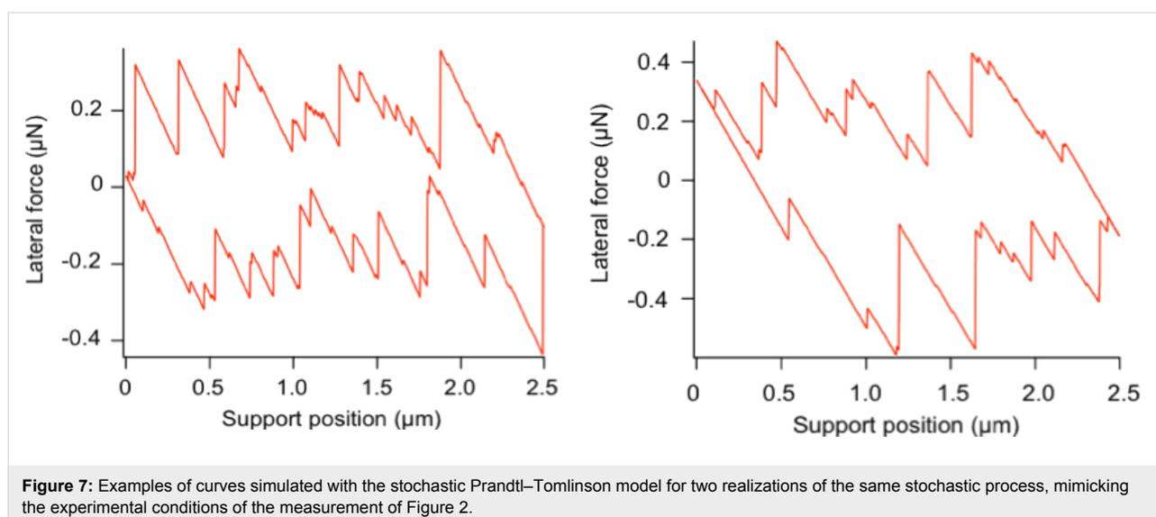
**Figure 7:** Examples of curves simulated with the stochastic Prandtl–Tomlinson model for two realizations of the same stochastic process, mimicking the experimental conditions of the measurement of Figure 2.
