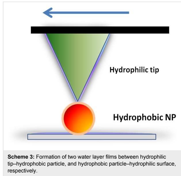
related to the intrinsic wetting properties of the interfacial system. As a consequence, the resulting water meniscus (or layer) can either increase friction through increased adhesion in the contact zone (hydrophilic interfaces) or reduce it through the lubricating effect of a water layer.
