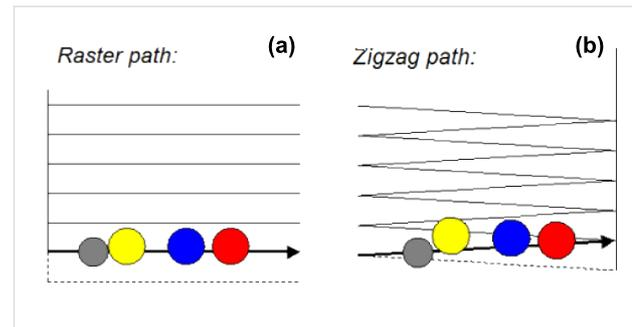
**Figure 3:** Typical scan patterns used in AFM: (a) raster scan path used by Nanosurf (b) zigzag scan path used by Veeco. *Top view:* the grey disk corresponds to the position of the tip on the surface and the yellow, blue and red disks are the positions of spherical particles pushed by the tip along its scan path.
