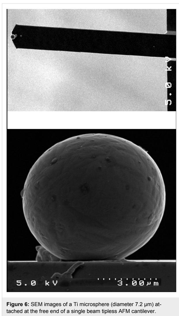
**Figure 6:** SEM images of a Ti microsphere (diameter 7.2  $\mu\text{m}$ ) attached at the free end of a single beam tipless AFM cantilever.
