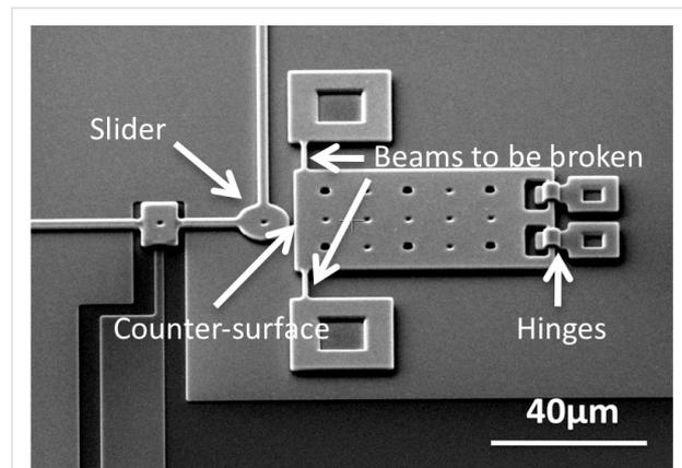
**Figure 5:** The counter-surface is held by two small beams. After the experiments, the beams can be broken and the counter-surface flipped upright in its hinges with a probe needle, allowing easy access with an AFM cantilever tip. The AFM has been used to measure the surface roughness (Figure 6) on the sidewall at the position where the arrow indicating ‘Counter-surface’ is pointing.
