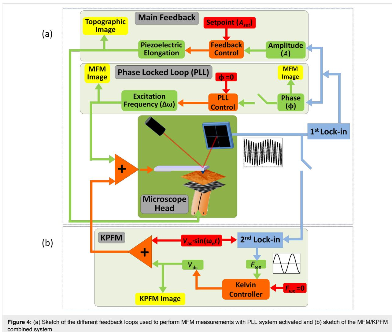
**Figure 4:** (a) Sketch of the different feedback loops used to perform MFM measurements with PLL system activated and (b) sketch of the MFM/KPFM combined system.
