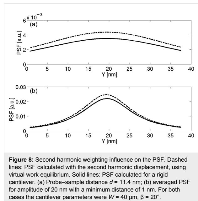
**Figure 8:** Second harmonic weighting influence on the PSF. Dashed lines: PSF calculated with the second harmonic displacement, using virtual work equilibrium. Solid lines: PSF calculated for a rigid cantilever. (a) Probe–sample distance  $d = 11.4$  nm; (b) averaged PSF for amplitude of 20 nm with a minimum distance of 1 nm. For both cases the cantilever parameters were  $W = 40 \mu\text{m}$ ,  $\beta = 20^\circ$ .
