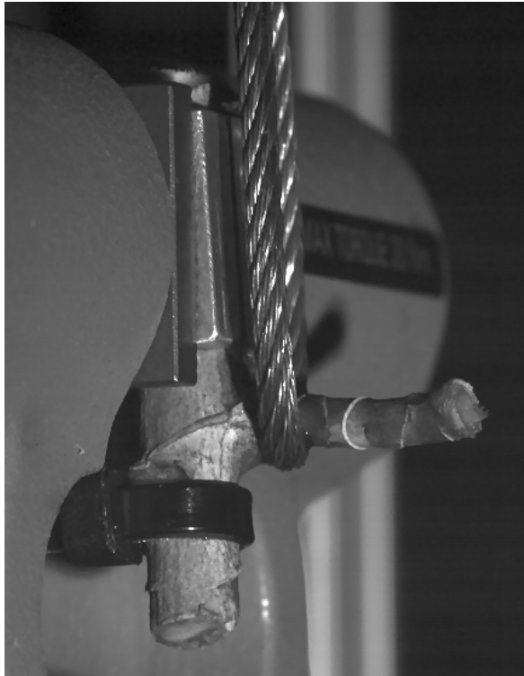
Figure 9: Breaking experiments. A critical force F_{crit} is applied to a branch of Dracaena reflexa by means of a steel cable connected to an Instron testing device. For technical reasons (direction of movement of the cross-head) the branch–stem-junctions are oriented ‘upside-down’ with regard to the original orientation in the plant.
