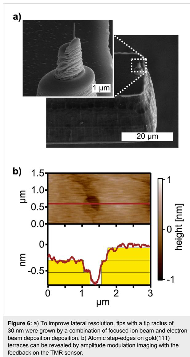
**Figure 6:** a) To improve lateral resolution, tips with a tip radius of 30 nm were grown by a combination of focused ion beam and electron beam deposition. b) Atomic step-edges on gold(111) terraces can be revealed by amplitude modulation imaging with the feedback on the TMR sensor.
