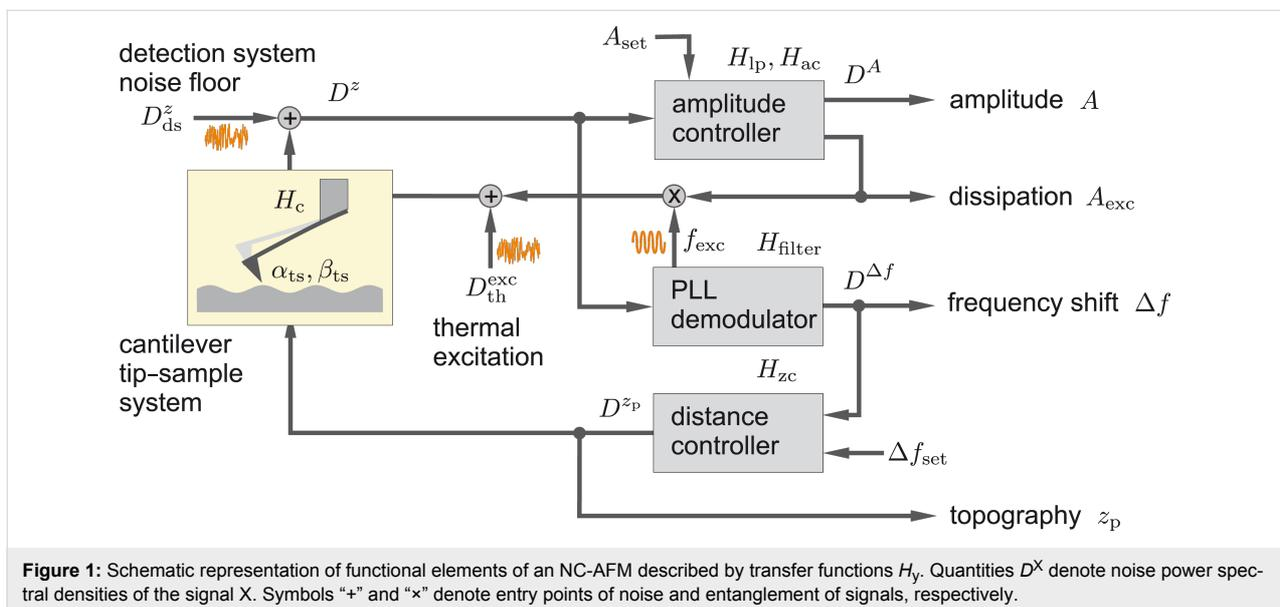
**Figure 1:** Schematic representation of functional elements of an NC-AFM described by transfer functions  $H_i$ . Quantities  $D^X$  denote noise power spectral densities of the signal X. Symbols “+” and “x” denote entry points of noise and entanglement of signals, respectively.
