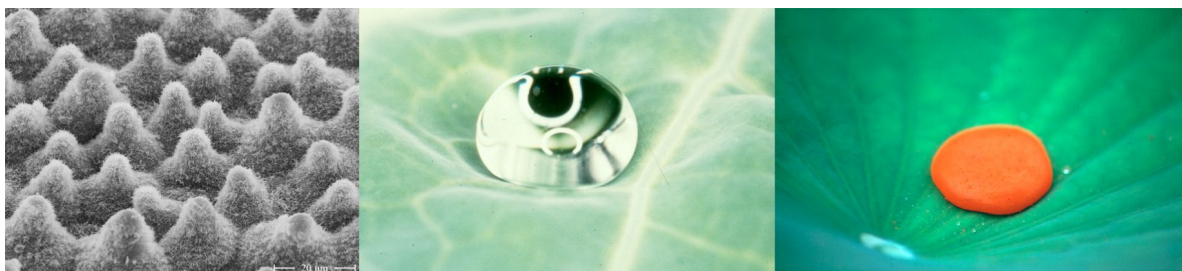
Figure 7: Fundamentals of self-cleaning in plants: a rough, hydrophobic surface (left) causes water to form spheres not adhering to the leaf (middle) removing particles while running off the leaf (right).
