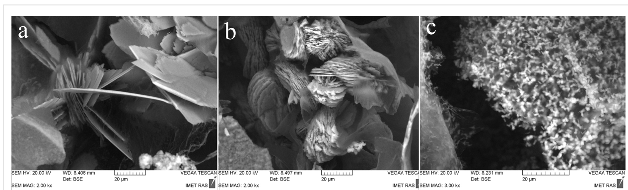
Figure 4: SEM micrographs of the microstructure of 3D printed samples on the basis of alginate with concentration of (a) 0.25, (b) 1.0 and (c) 2.0 wt %.
