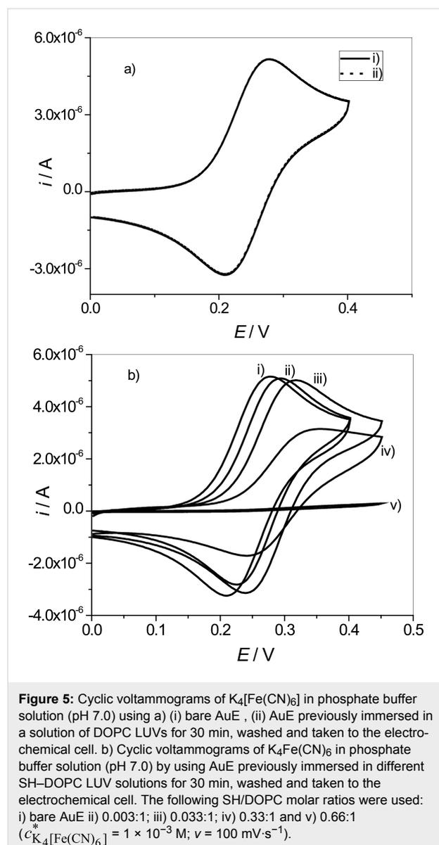
As the SH/DOPC ratio was increased, a decrease of the  $[Fe(CN)_6]^{4-}$  peak intensity of the current (oxidation and reduction) was observed. Moreover, at a ratio of SH/DOPC = 0.66:1, the  $[Fe(CN)_6]^{4-}$  couple redox peak intensity of the current decreases drastically indicating that the AuE surface was
