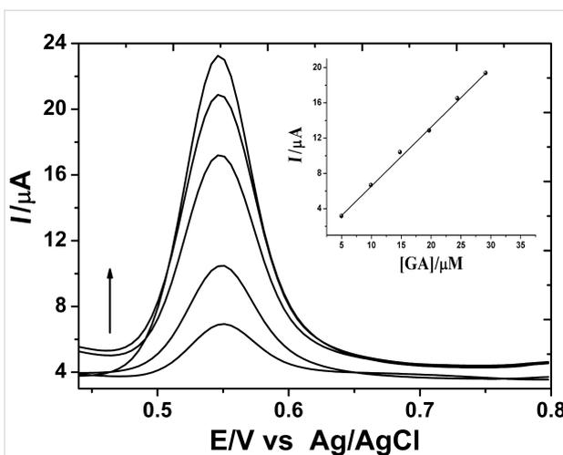
**Figure 6:** SW voltammograms obtained at optimal conditions in 0.2 M H<sub>3</sub>PO<sub>4</sub> solution containing different GA concentrations. Inset: analytical curve.
