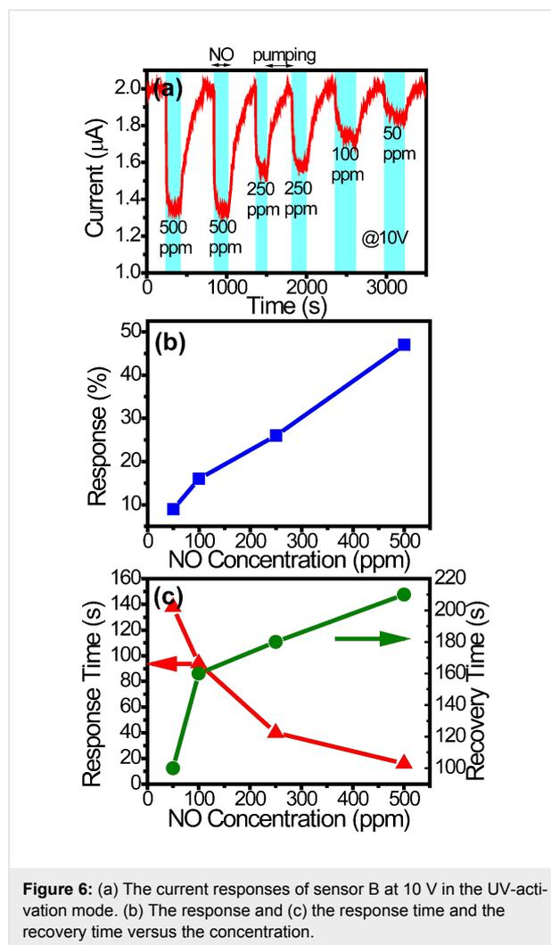
**Figure 6:** (a) The current responses of sensor B at 10 V in the UV-activation mode. (b) The response and (c) the response time and the recovery time versus the concentration.
