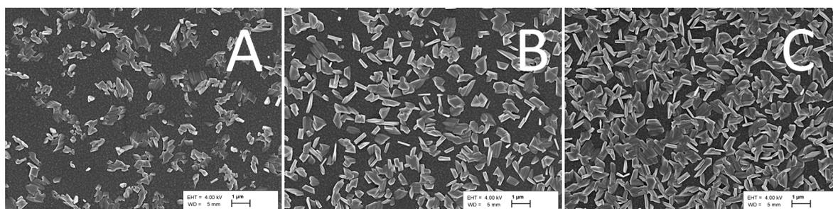
**Figure 2:** SEM images of  $\text{Sb}_2\text{S}_3$  crystalline flakes grown by spraying solutions with a precursor ratio of 1:6 onto a  $\text{TiO}_2$  substrate kept at 250 °C using 3, 7 and 11 deposition cycles, depicted in images A, B and C, respectively. The linear dimensions of the flakes, or coalesced flakes, are in the range of 200–800 nm, 500–1200 nm and 800–1500 nm in panels A, B and C, respectively.
