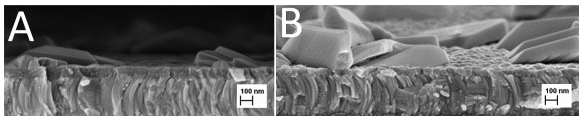
**Figure 3:** Cross-sectional SEM image of the glass/ITO/ $\text{TiO}_2$ / $\text{Sb}_2\text{S}_3$  structure, the topmost  $\text{Sb}_2\text{S}_3$  layer consists of nanoparticles grown by ultrasonic CSP using three spray cycles (A) or nine spray cycles (B).
