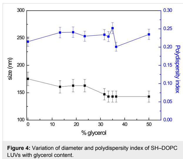
chemical measurements, employing different molar ratios of SH and DOPC as it is described in subsection “Vesicles preparation” of the Experimental section. All diameters of these organized systems were around 175 nm with a polydispersity of 0.2 determined by DLS indicating that the size of the LUVs does not change significantly by the incorporation of SH to the bilayer.
