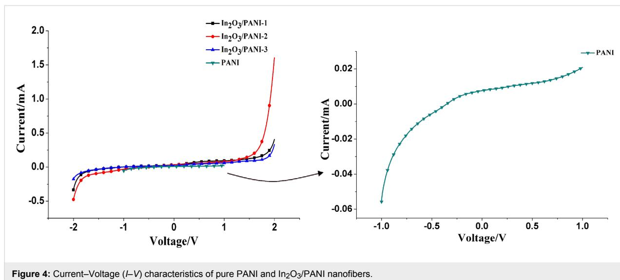
Figure 4: Current–Voltage ( $I$ – $V$ ) characteristics of pure PANI and  $\text{In}_2\text{O}_3$ /PANI nanofibers.
