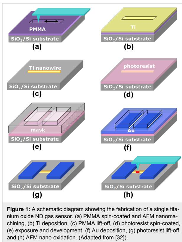
**Figure 1:** A schematic diagram showing the fabrication of a single titanium oxide ND gas sensor. (a) PMMA spin-coated and AFM nanomachining, (b) Ti deposition, (c) PMMA lift-off, (d) photoresist spin-coated, (e) exposure and development, (f) Au deposition, (g) photoresist lift-off, and (h) AFM nano-oxidation. (Adapted from [32]).
