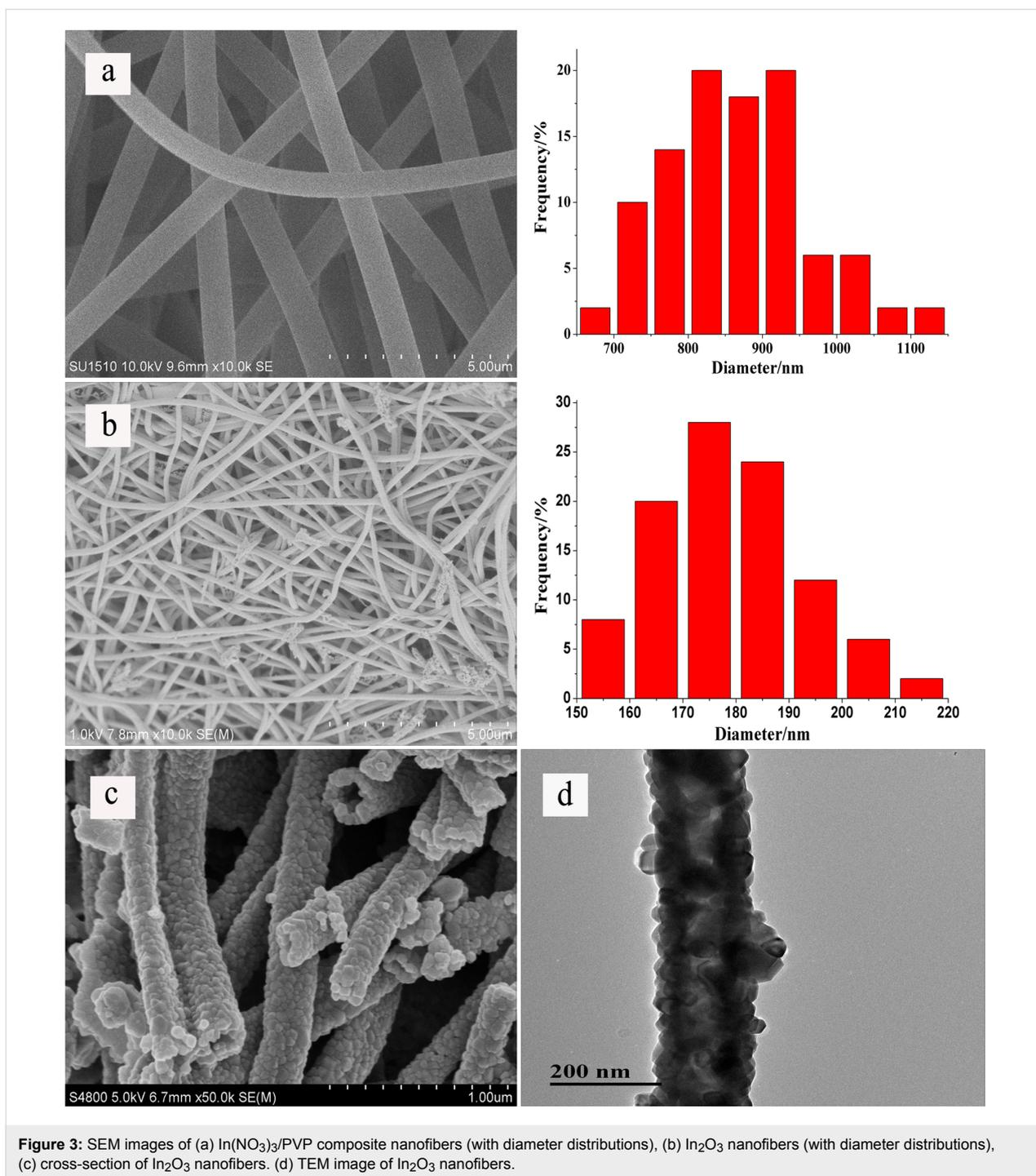
**Figure 3:** SEM images of (a) In(NO<sub>3</sub>)<sub>3</sub>/PVP composite nanofibers (with diameter distributions), (b) In<sub>2</sub>O<sub>3</sub> nanofibers (with diameter distributions), (c) cross-section of In<sub>2</sub>O<sub>3</sub> nanofibers. (d) TEM image of In<sub>2</sub>O<sub>3</sub> nanofibers.
