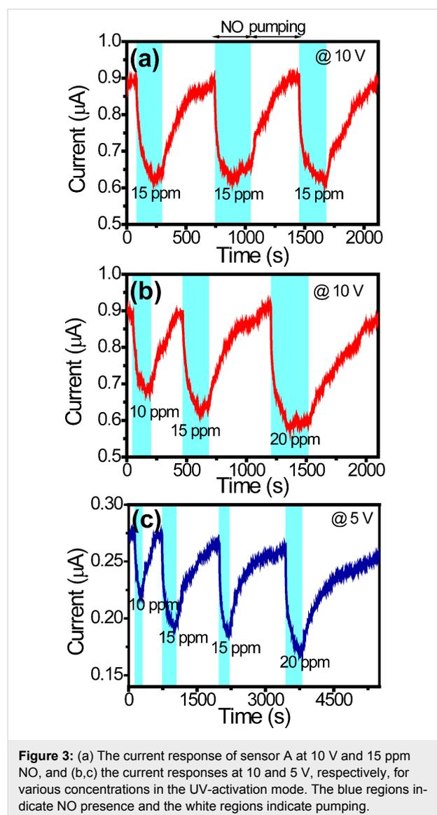
**Figure 3:** (a) The current response of sensor A at 10 V and 15 ppm NO, and (b,c) the current responses at 10 and 5 V, respectively, for various concentrations in the UV-activation mode. The blue regions indicate NO presence and the white regions indicate pumping.
