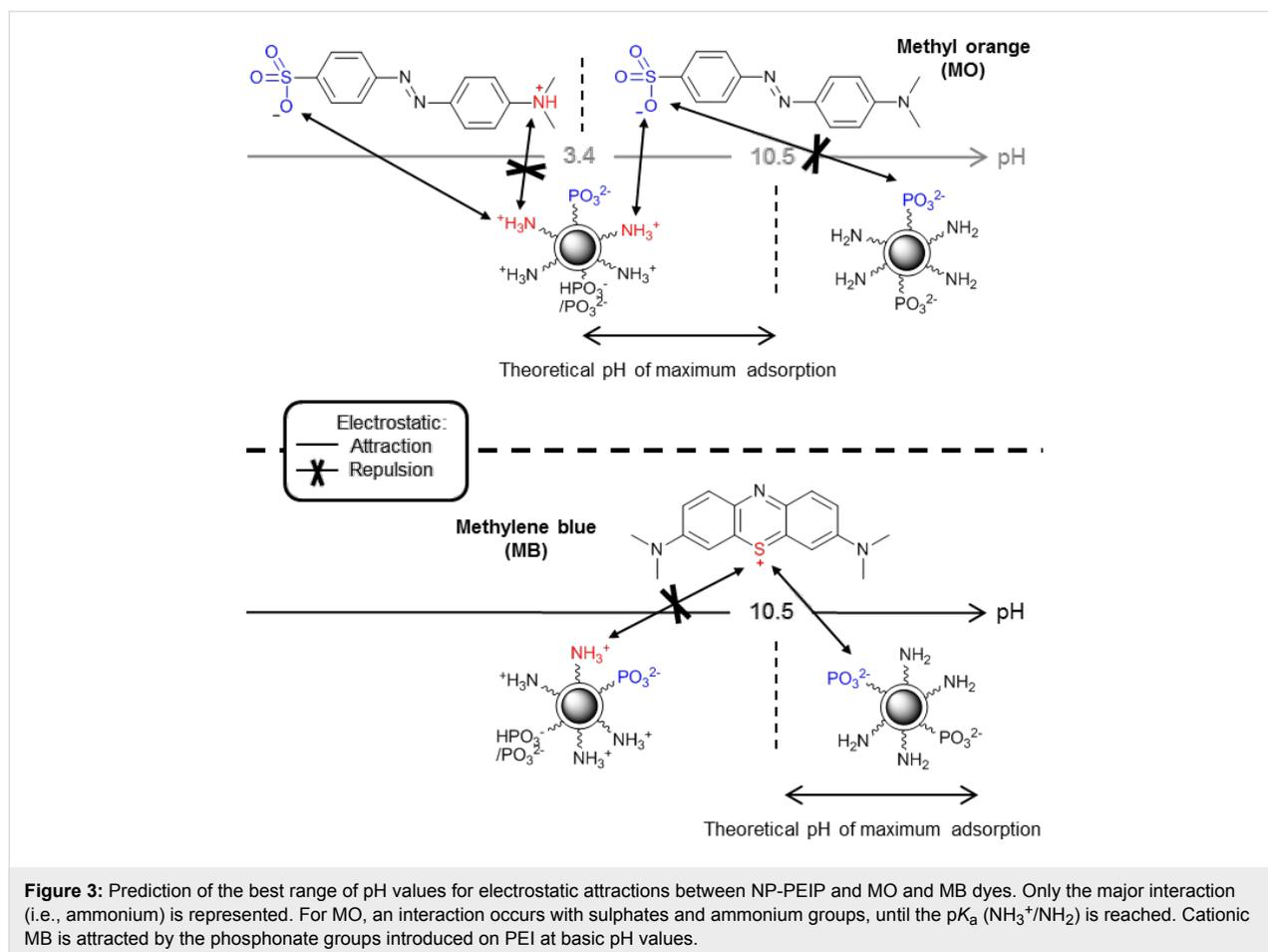
the sulfur atom is always positively charged. The adsorption therefore increases after the second deprotonation of phosphonate, and is maximized above  $pK_a$  of the ammonium/amine deprotonation, where repulsive forces are negligible. All of these results show that, in the case of maghemite coated with phosphonated PEI adsorbing MO and MB, electrostatic interactions are predominant.
