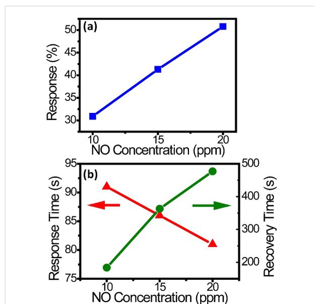
**Figure 4:** (a) Response and (b) response time and recovery time as a function of the concentration for sensor A at 10 V in the UV-activation mode calculated from Figure 3b.
