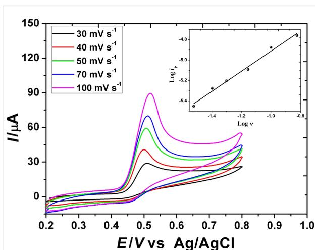
**Figure 5:** Effect of scan rate on the cyclic voltammograms recorded for the first wave of 1.0 mM GA on the PGA/MWCNT/GCE modified electrode in 0.2 M H<sub>3</sub>PO<sub>4</sub> (pH 2.0). Inset:  $\log i_p^a$ – $\log v$  relationship.
