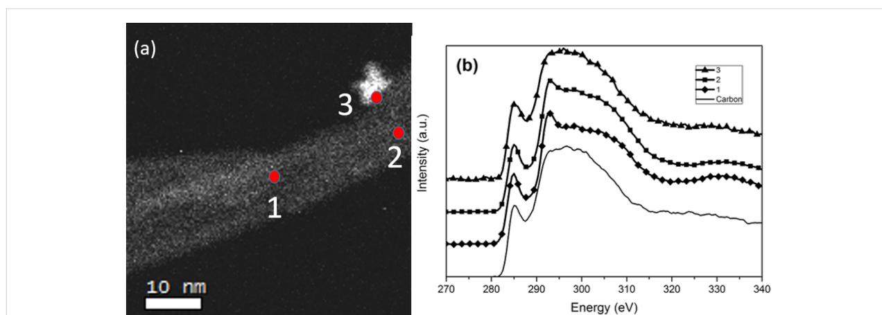
**Figure 4:** (a) HAADF-STEM image of the area of interest where EELS was performed, (b) C K-edge core loss EELS spectra on the area of interest indicated in Figure 2a.
