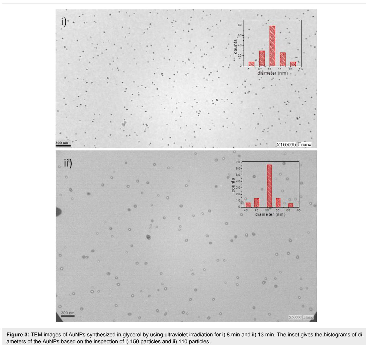
**Figure 3:** TEM images of AuNPs synthesized in glycerol by using ultraviolet irradiation for i) 8 min and ii) 13 min. The inset gives the histograms of diameters of the AuNPs based on the inspection of i) 150 particles and ii) 110 particles.
