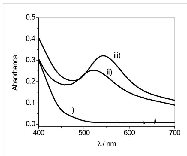
**Figure 2:** UV–vis spectra in glycerol: i) the HClAu<sub>4</sub> precursor; ii) the AuNPs synthesized with 8 min of irradiation time; iii) the AuNPs synthesized with 13 min of irradiation time ( $\lambda_{\text{irradiation}} = 300 \text{ nm}$ ).
