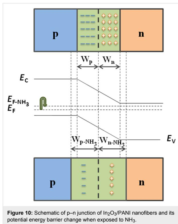
**Figure 10:** Schematic of p–n junction of  $\text{In}_2\text{O}_3/\text{PANI}$  nanofibers and its potential energy barrier change when exposed to  $\text{NH}_3$ .
