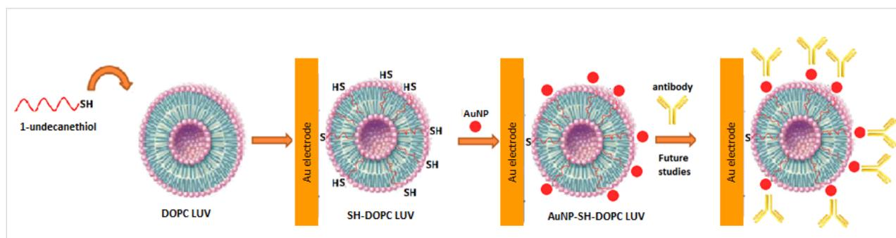
**Figure 1:** Platform to design a possible immunosensor.
