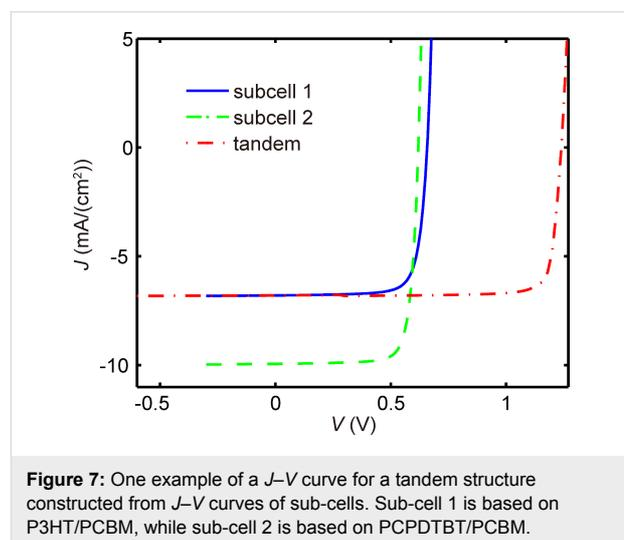
**Figure 7:** One example of a  $J$ – $V$  curve for a tandem structure constructed from  $J$ – $V$  curves of sub-cells. Sub-cell 1 is based on P3HT/PCBM, while sub-cell 2 is based on PCPDTBT/PCBM.
