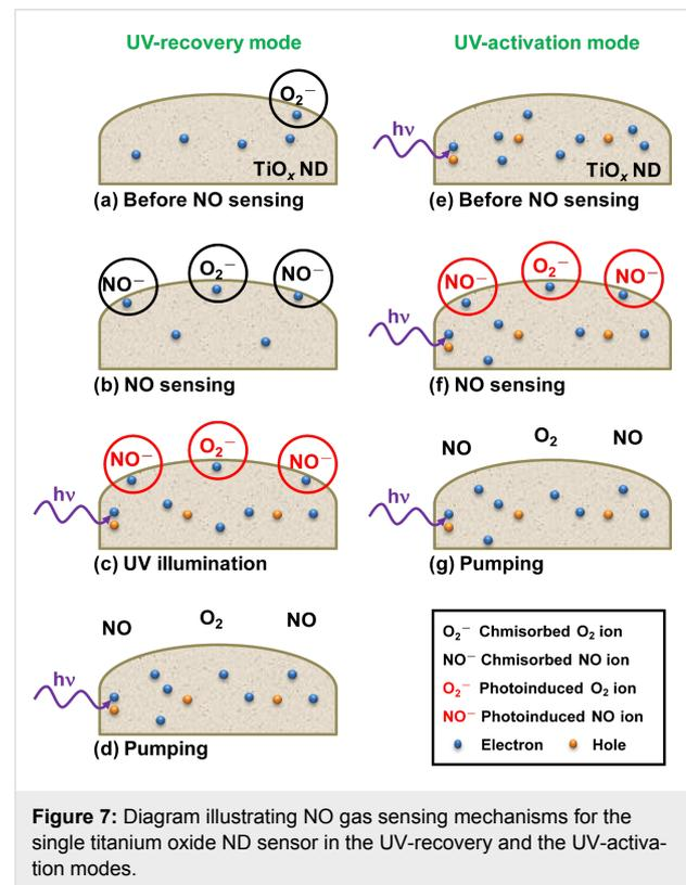
**Figure 7:** Diagram illustrating NO gas sensing mechanisms for the single titanium oxide ND sensor in the UV-recovery and the UV-activation modes.
