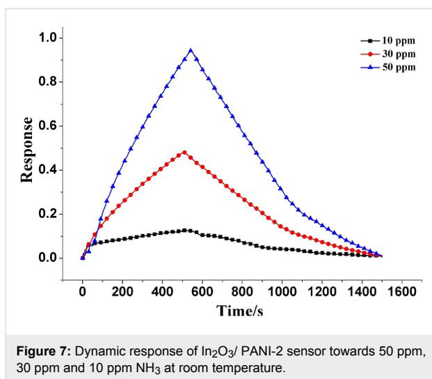
resistance [37,38]. When this reaction reached equilibrium in  $\text{NH}_3$  atmosphere, the resistance of the PANI-based sensor maintained a constant value. When the sensor was exposed to air,  $\text{NH}_3$  is volatilized and the resistance of the PANI composite nanofibers is reduced. Therefore, due to the unique mechanism,
