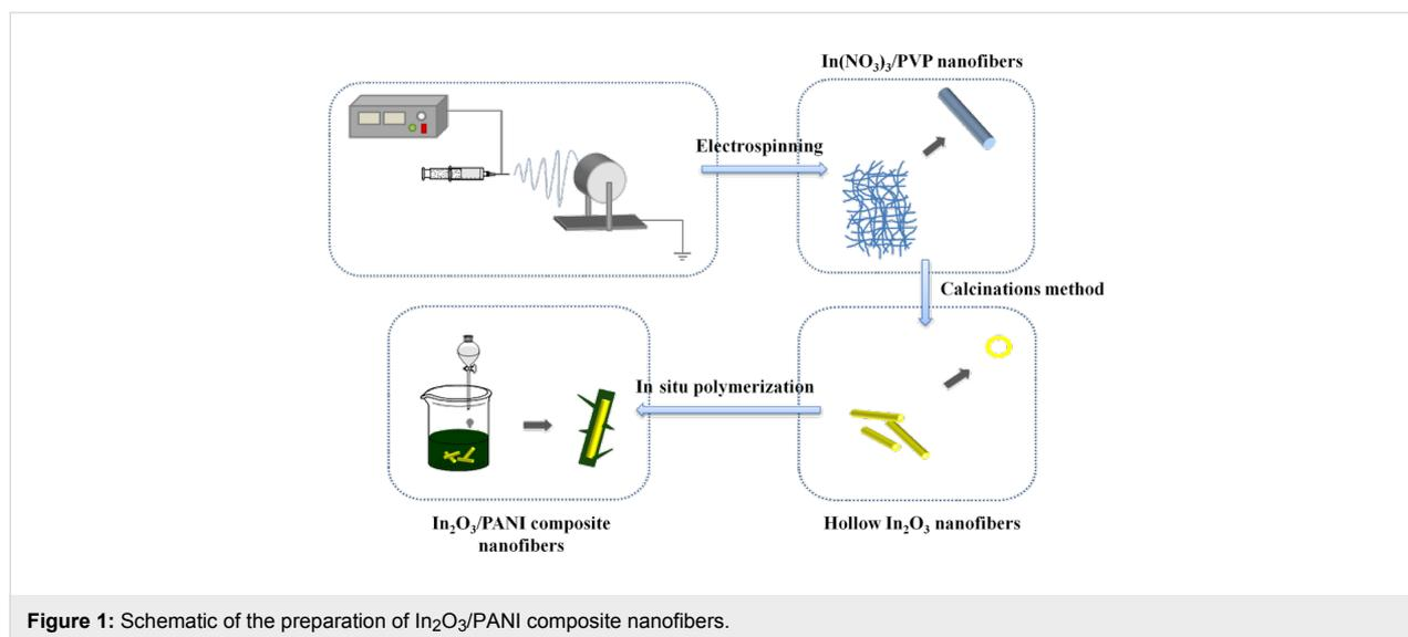
**Figure 1:** Schematic of the preparation of In<sub>2</sub>O<sub>3</sub>/PANI composite nanofibers.
