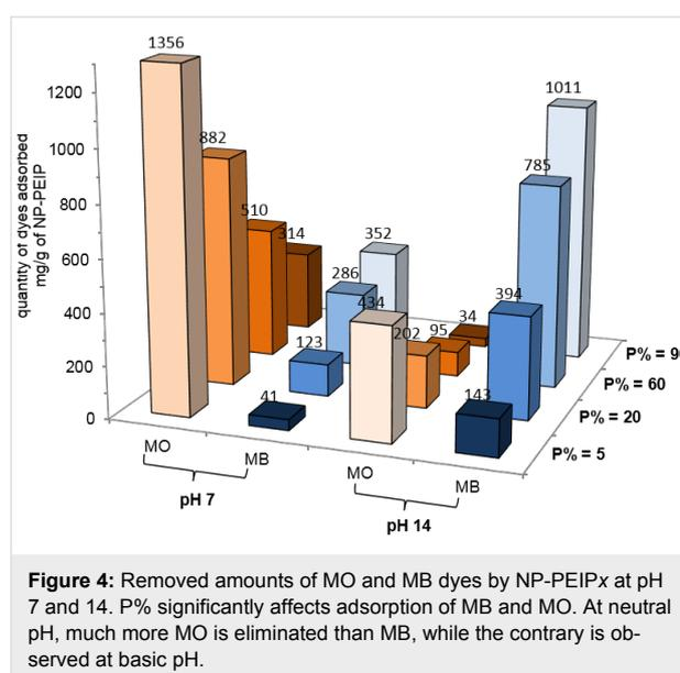
The phosphonation rate also strongly influences the adsorption of MB. The value of  $q_{\text{max}}$  is increased to the seven-fold between  $P\% = 5$  and  $P\% = 90$  at pH 14 with a maximum of
