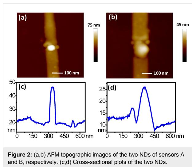
**Figure 2:** (a,b) AFM topographic images of the two NDs of sensors A and B, respectively. (c,d) Cross-sectional plots of the two NDs.
