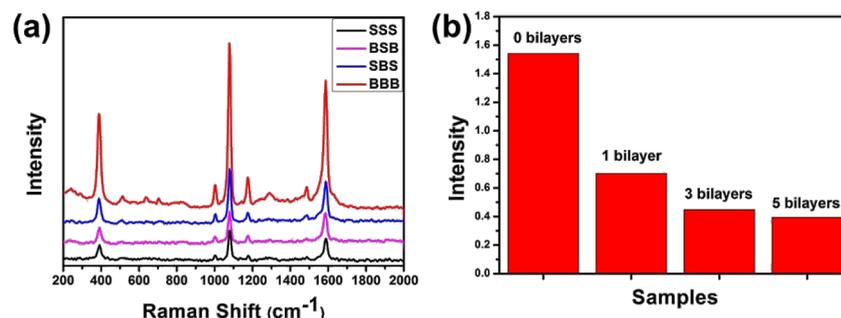
**Figure 3:** (a) SERS spectra of the sandwich-like multilayer thin films; (b) SERS intensity variations at  $1078\text{ cm}^{-1}$  for LbL thin films inserted with different numbers of PDDA/PSS bilayers.
