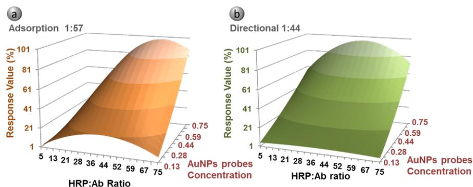
**Figure 2:** DOE experimental results for adsorption (a) and directional (b) methods. Estimation of the effect on response of HRP/Ab ratio and AuNP probe concentration. The layout displays the response value as percent of the maximal HRP signal at 450 nm. Coefficient of determination of DOE results  $R^2 = 0.9485$  (a) and  $R^2 = 0.9768$  (b).
