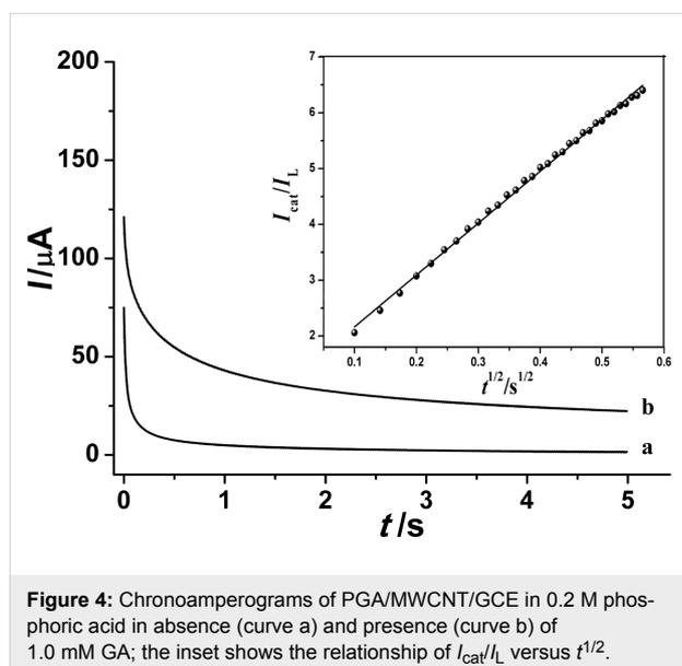
**Figure 4:** Chronoamperograms of PGA/MWCNT/GCE in 0.2 M phosphoric acid in absence (curve a) and presence (curve b) of 1.0 mM GA; the inset shows the relationship of  $i_{cat}/i_L$  versus  $t^{1/2}$ .
