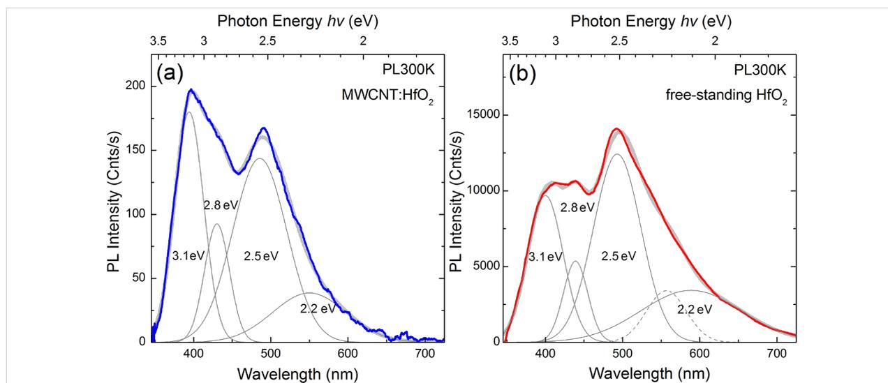
**Figure 3:** (a) Room temperature photoluminescence spectra of MWCNTs decorated with cubic HfO<sub>2</sub> nanoparticles (from a colloidal suspension in ethanol) compared to (b) free-standing HfO<sub>2</sub> nanoparticles. Grey curves represent the Gaussian deconvolution components. Note different the photoluminescence intensity scales in (a) and (b).
