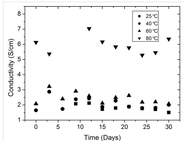
**Figure 6:** Time dependence of the electrical conductivity of PANI thin films annealed at different temperatures. The decrease in the conductivity after 30 days was less than 2% and did not depend on the annealing temperature.
