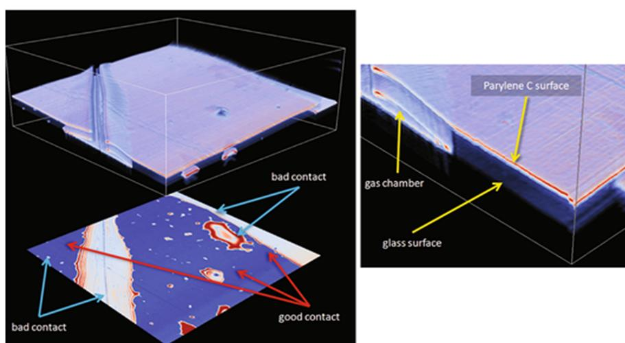
**Figure 11:** Volumetric reconstruction of the Parylene C-coated microscopy glass (left, atop) and calculated amplitude map of the Parylene C/glass interface (left, bottom). Boundary box indicates the size of the volume  $2000 \times 2000 \times 208 \mu\text{m}$ . Zoom-in image (right). Coating defects and gas chambers are clearly visible. Reprinted with the permission from [68], copyright 2011 Springer.
