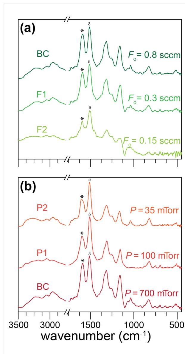
**Figure 4:** FTIR of washed oCVD PANI films based on the experimental conditions in Table 1. Effect of (a) reactor pressure, and (b) oxidant flow rate on oCVD PANI chemistry after washing. The quinoid and benzenoid groups are labeled by \* and  $\delta$ , respectively.
