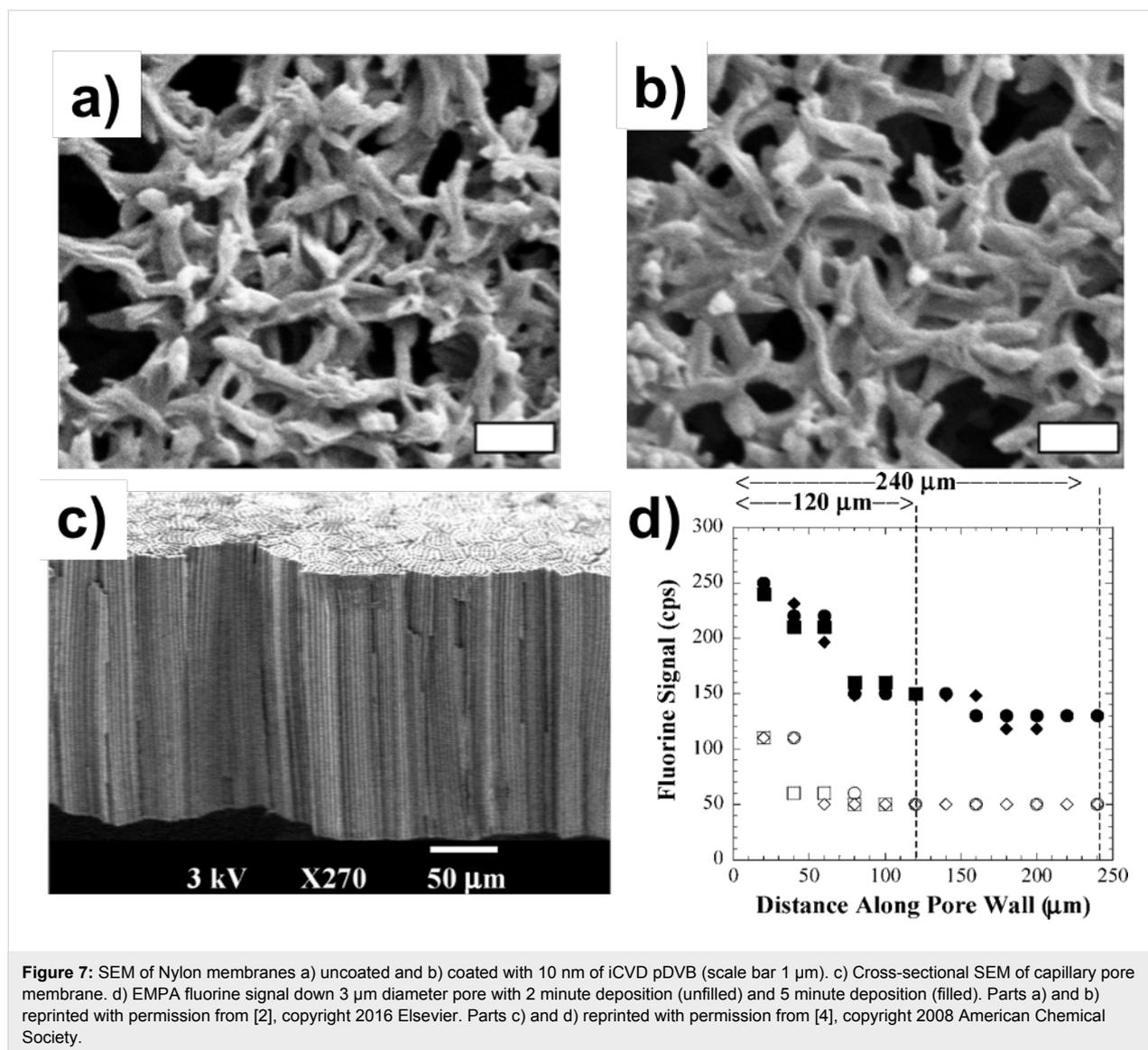
**Figure 7:** SEM of Nylon membranes a) uncoated and b) coated with 10 nm of iCVD pDVB (scale bar 1 μm). c) Cross-sectional SEM of capillary pore membrane. d) EMPA fluorine signal down 3 μm diameter pore with 2 minute deposition (unfilled) and 5 minute deposition (filled). Parts a) and b) reprinted with permission from [2], copyright 2016 Elsevier. Parts c) and d) reprinted with permission from [4], copyright 2008 American Chemical Society.
