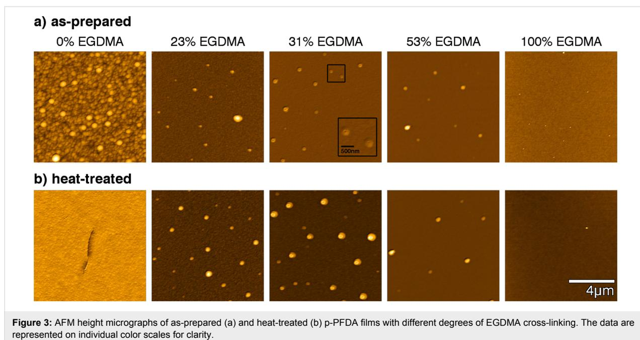
**Figure 3:** AFM height micrographs of as-prepared (a) and heat-treated (b) p-PFDA films with different degrees of EGDMA cross-linking. The data are represented on individual color scales for clarity.
