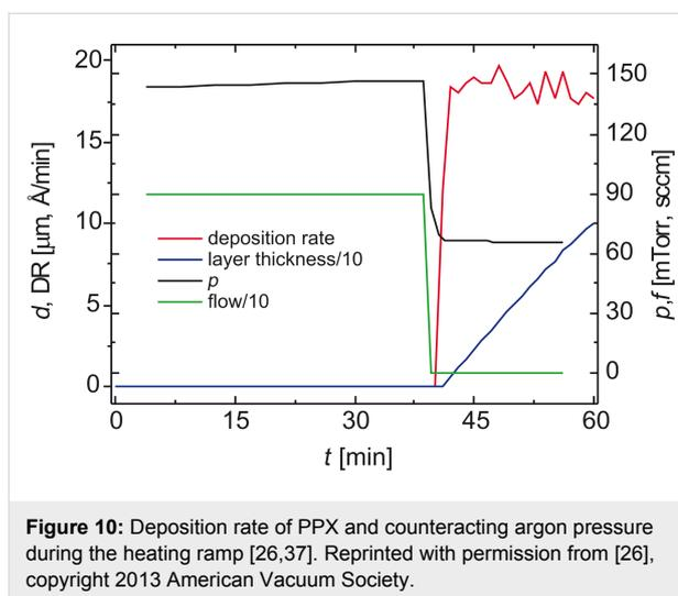
**Figure 10:** Deposition rate of PPX and counteracting argon pressure during the heating ramp [26,37]. Reprinted with permission from [26], copyright 2013 American Vacuum Society.
