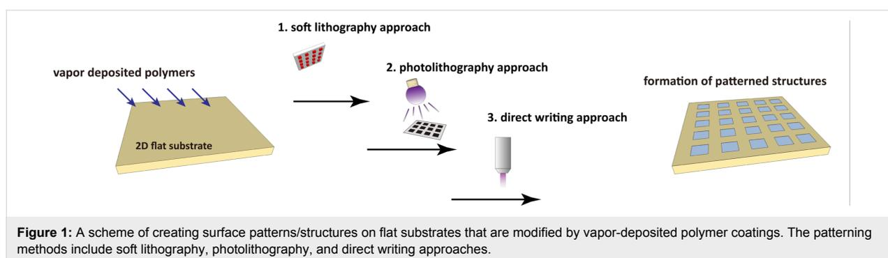
**Figure 1:** A scheme of creating surface patterns/structures on flat substrates that are modified by vapor-deposited polymer coatings. The patterning methods include soft lithography, photolithography, and direct writing approaches.
