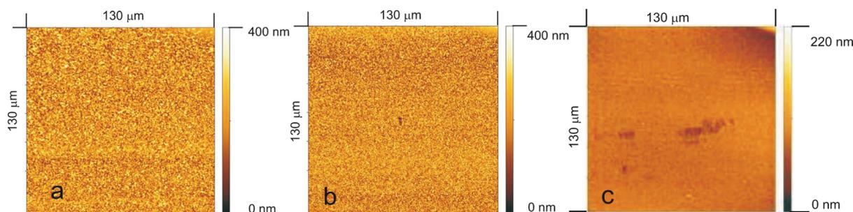
**Figure 18:** Surface morphology of parylene films deposited at various deposition pressures. Flow of the monomeric species was fixed to 9 sccm. Process pressure was established by adding argon to the ambient. (a) Without diluent, 6 mTorr (0.8 Pa), (b) 37.5 mTorr (5 Pa), (c) 75 mTorr (10 Pa). Reprinted from [60], copyright 2015 the authors.
