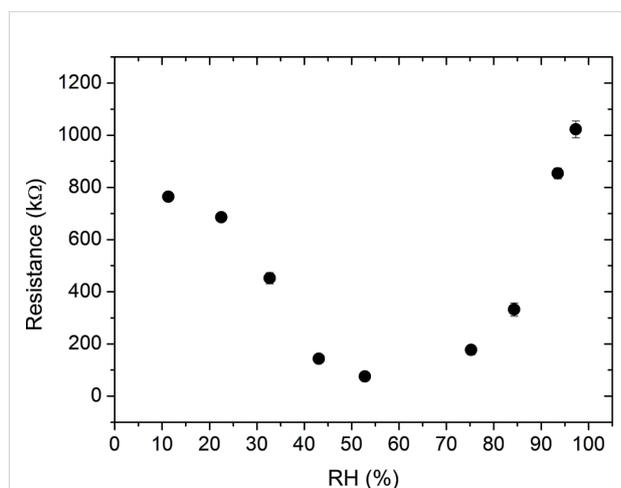
**Figure 9:** Resistance of single-component PANI nanotubes as a function of the relative humidity. The competing effects of doping and swelling lead to the parabolic behavior, which is similar to the observed behavior in PANI thin films.
