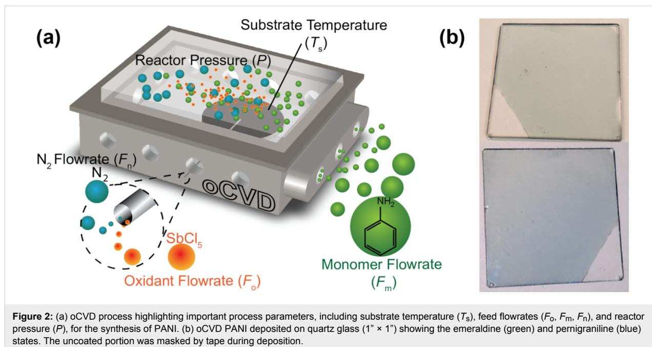
**Figure 2:** (a) oCVD process highlighting important process parameters, including substrate temperature ( $T_s$ ), feed flowrates ( $F_o$ ,  $F_m$ ,  $F_n$ ), and reactor pressure ( $P$ ), for the synthesis of PANI. (b) oCVD PANI deposited on quartz glass ( $1'' \times 1''$ ) showing the emeraldine (green) and pernigraniline (blue) states. The uncoated portion was masked by tape during deposition.
