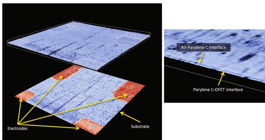
**Figure 12:** Volumetric reconstruction of the Parylene C-coated OFET structure (left, atop) and calculated amplitude map of the Parylene C/substrate interface (left, bottom). Boundary box indicates the size of the volume  $2000 \times 2000 \times 73 \mu\text{m}$ . Zoom-in image showing interfaces of 2  $\mu\text{m}$  thin polymer layer (right). Reprinted with the permission from [68], copyright 2011 Springer.
