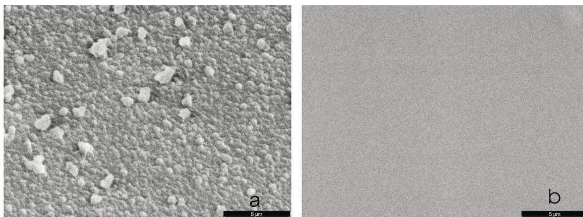
**Figure 17:** (a) Parylene N deposited in pure atmosphere of *p*-xylylene at a total pressure of 6 mTorr; (b) parylene N deposited in *p*-xylylene diluted with at a total pressure of 50 mTorr. At constant partial pressure of the monomer, the volume polymerization at low pressure is effectively suppressed. Reprinted from [60], copyright 2015 the authors.
