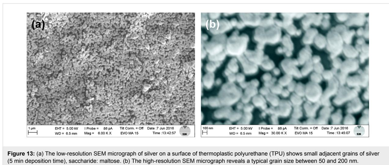
**Figure 13:** (a) The low-resolution SEM micrograph of silver on a surface of thermoplastic polyurethane (TPU) shows small adjacent grains of silver (5 min deposition time), saccharide: maltose. (b) The high-resolution SEM micrograph reveals a typical grain size between 50 and 200 nm.
