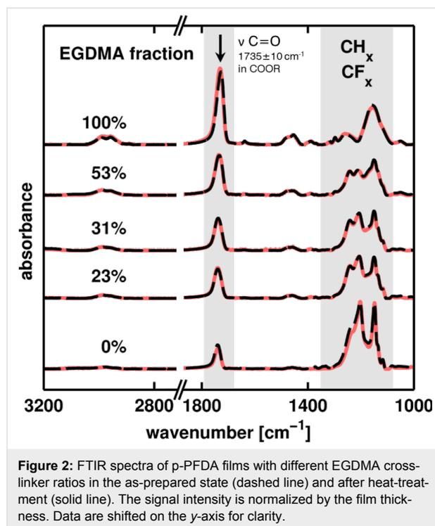
**Figure 2:** FTIR spectra of p-PFDA films with different EGDMA cross-linker ratios in the as-prepared state (dashed line) and after heat-treatment (solid line). The signal intensity is normalized by the film thickness. Data are shifted on the y-axis for clarity.
