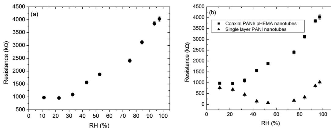
**Figure 10:** (a) Change in the resistance of coaxial PANI/pHEMA nanotubes with relative humidity. (b) Comparison of the single component and coaxial nanotubes in terms of humidity effect on resistance. The parabolic behavior observed in single-component nanotubes is not observed in the coaxial nanotubes, suggesting the dominance of the swelling effect in the presence of pHEMA hydrogel inner layer.
