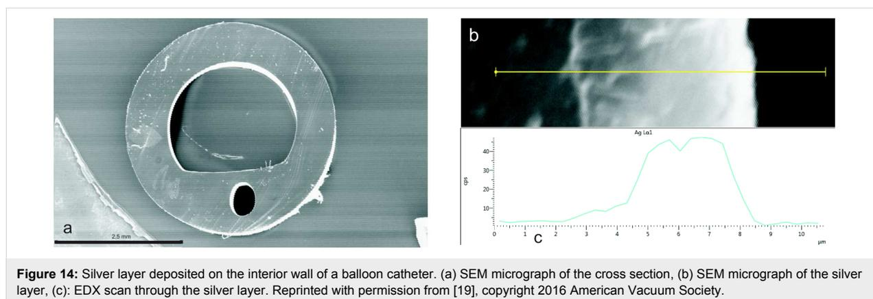
**Figure 14:** Silver layer deposited on the interior wall of a balloon catheter. (a) SEM micrograph of the cross section, (b) SEM micrograph of the silver layer, (c): EDX scan through the silver layer. Reprinted with permission from [19], copyright 2016 American Vacuum Society.
