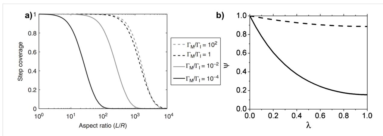
**Figure 5:** a) Step coverage as function of aspect ratio and ratio of sticking coefficients from numerical solutions of Equation 6. b) Concentration profile of perfluorodecyl acrylate (solid line) and divinyl benzene (dashed line) down a pore. a) Reprinted with permission from [1], copyright 2015 John Wiley and Sons. b) Reprinted with permission from [3], copyright 2011 American Chemical Society.
