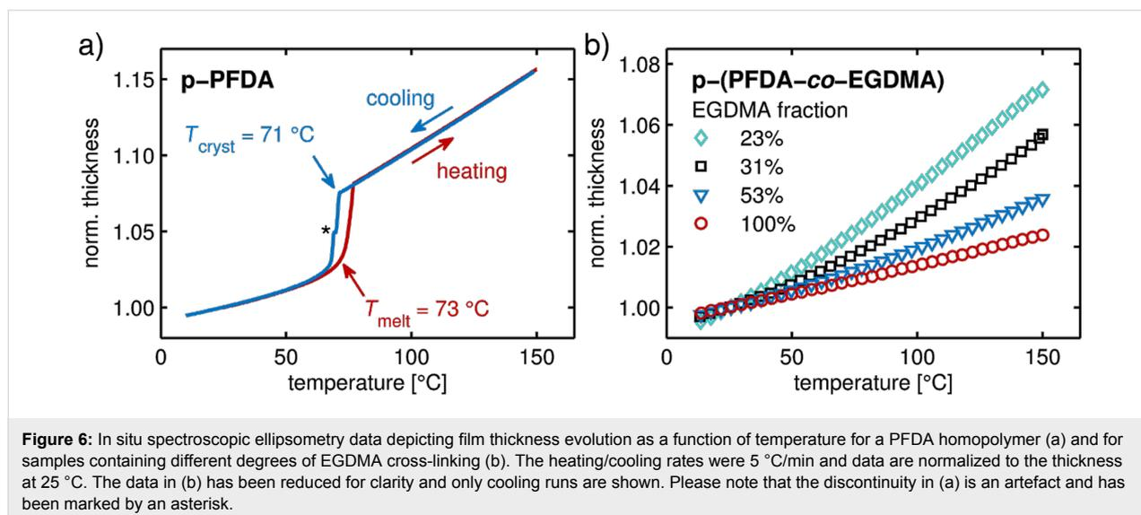
**Figure 6:** In situ spectroscopic ellipsometry data depicting film thickness evolution as a function of temperature for a PFDA homopolymer (a) and for samples containing different degrees of EGDMA cross-linking (b). The heating/cooling rates were 5 °C/min and data are normalized to the thickness at 25 °C. The data in (b) has been reduced for clarity and only cooling runs are shown. Please note that the discontinuity in (a) is an artefact and has been marked by an asterisk.
