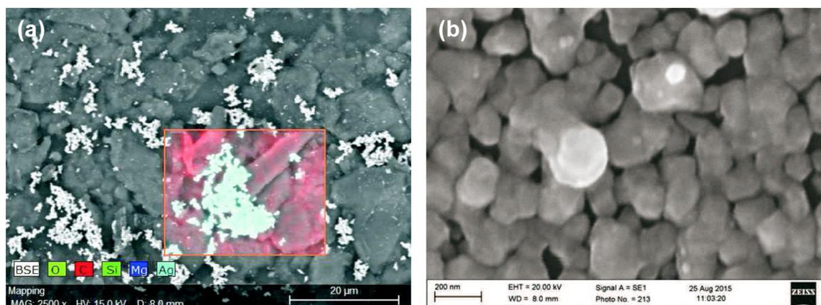
**Figure 15:** (a) The low-resolution SEM micrograph of silver on a rough polysilicone surface shows disconnected spots of silver (10 min deposition time, disaccharide: maltose). (b) The high-resolution SEM micrograph reveals a typical grain size of 50–200 nm. Reprinted with permission from [19], copyright 2016 American Vacuum Society.
