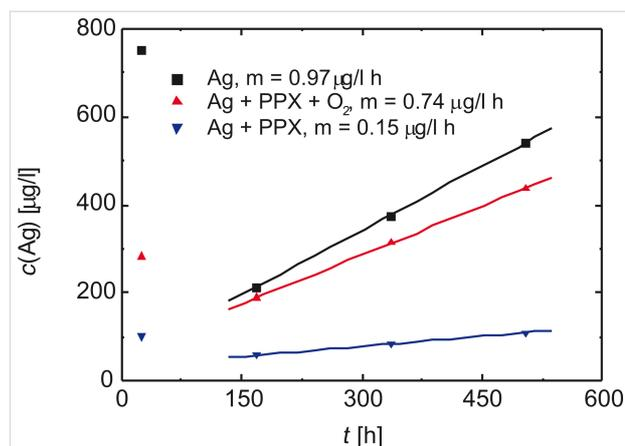
**Figure 24:** After 24 h, the released amount of  $\text{Ag}^+$  ions from the PPX layer does not depend on time and is almost constant. Reprinted with permission from [19], copyright 2016 American Vacuum Society.
