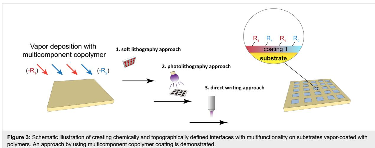
**Figure 3:** Schematic illustration of creating chemically and topographically defined interfaces with multifunctionality on substrates vapor-coated with polymers. An approach by using multicomponent copolymer coating is demonstrated.
