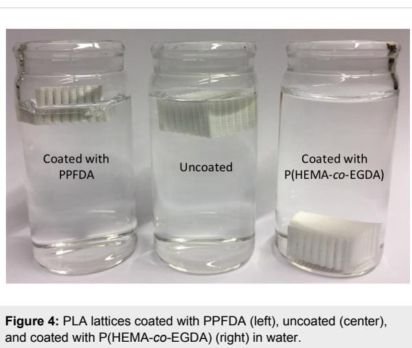
**Figure 4:** PLA lattices coated with PPFDA (left), uncoated (center), and coated with P(HEMA-co-EGDA) (right) in water.
