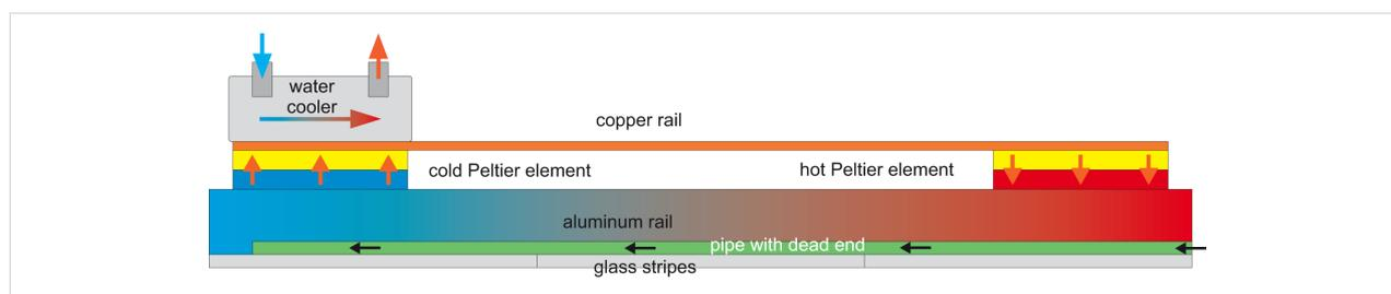
**Figure 7:** A “temperature seesaw” with several heating or cooling elements can equalize the density gradient that will develop as consequence of diffusion and simultaneous loss of diffusing molecules. Reprinted with permission from [35], copyright 2017 American Institute of Physics.
