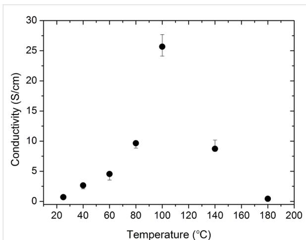
**Figure 5:** Electrical conductivity of PANI thin films at different annealing temperatures. The conductivity of the films increases with increasing annealing temperatures up to 100 °C because of the increase in crystallinity. Above 100 °C the crystalline structure is damaged leading to the reduction of conductivity.
