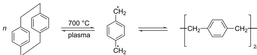
**Figure 4:** CVD process: The dimeric species di(*p*-xylylene) (DPX, left), which contains two ethyl bridges in each *para*-position, is cracked to form the *p*-xylylene diradical (PX, middle), which forms polymeric chains of poly(*p*-xylylene) (PPX, right) [27]. This reaction can occur either in the gas phase (volume polymerization) or on a cold surface (surface polymerization).
