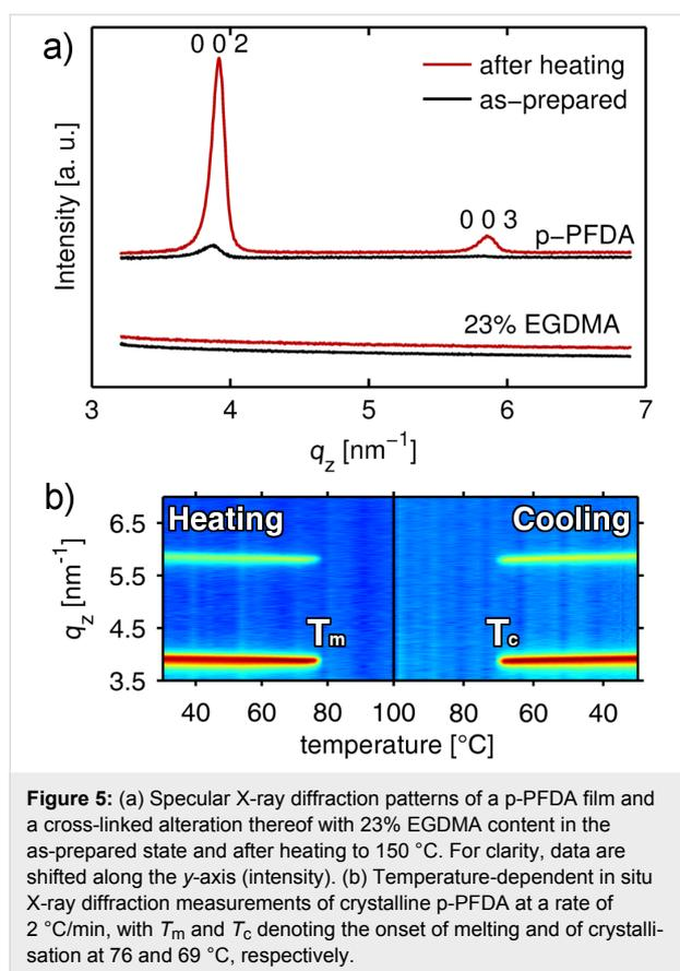
**Figure 5:** (a) Specular X-ray diffraction patterns of a p-PFDA film and a cross-linked alteration thereof with 23% EGDMA content in the as-prepared state and after heating to 150 °C. For clarity, data are shifted along the  $y$ -axis (intensity). (b) Temperature-dependent in situ X-ray diffraction measurements of crystalline p-PFDA at a rate of 2 °C/min, with  $T_m$  and  $T_c$  denoting the onset of melting and of crystallization at 76 and 69 °C, respectively.
