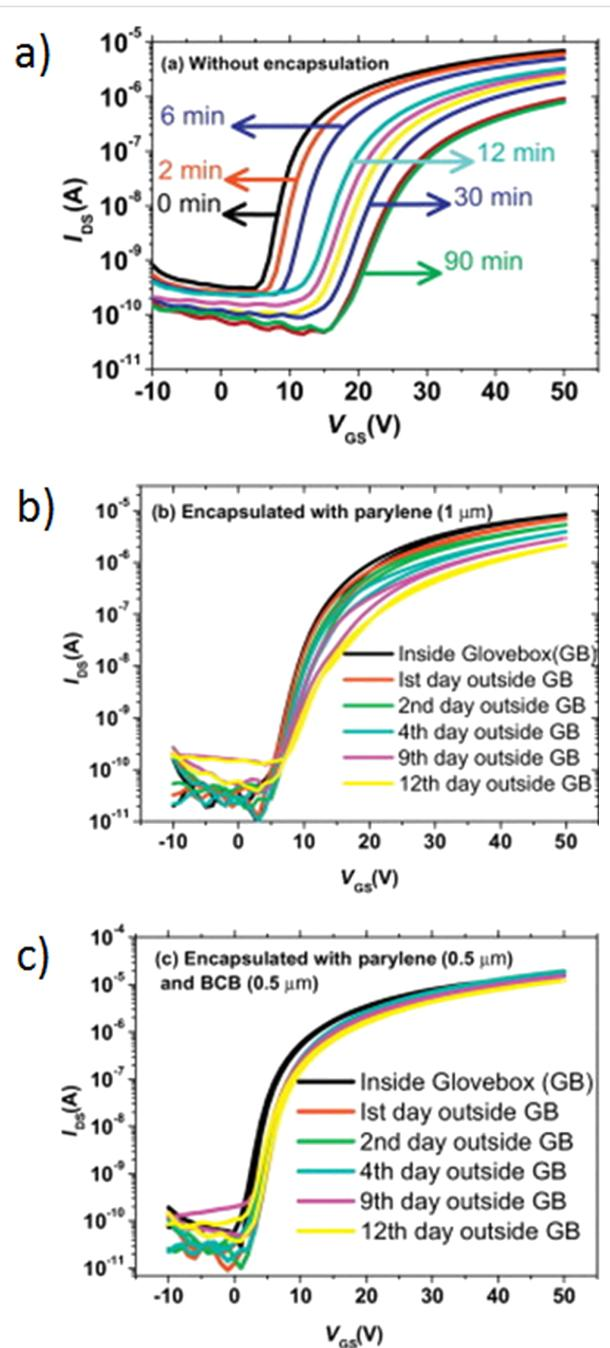
**Figure 13:** Transfer characteristics recorded under ambient conditions of a fullerene transistor without encapsulation (a), encapsulated with 1  $\mu\text{m}$  thick layer of Parylene C (b) and encapsulated with 0.5  $\mu\text{m}$  thick layer of Parylene C followed by 0.5  $\mu\text{m}$  layer of benzocyclobutene (c). Reprinted with the permission from [69], copyright 2014 Elsevier.
