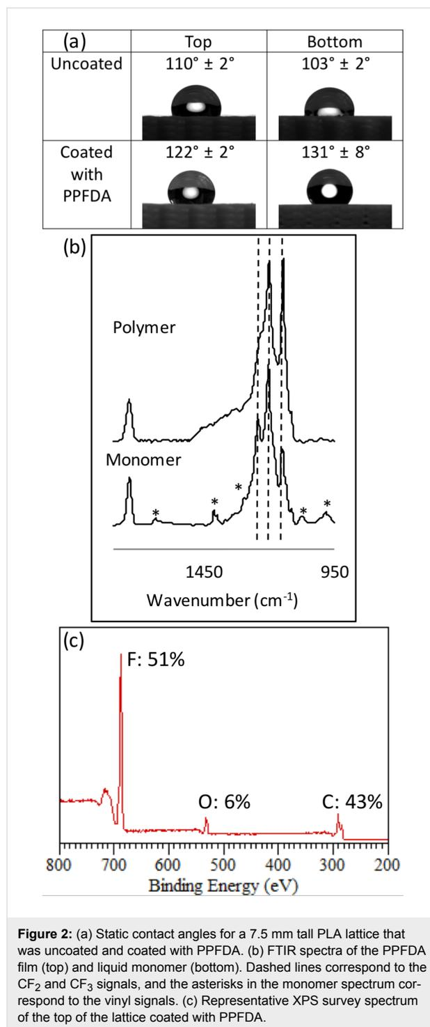
**Figure 2:** (a) Static contact angles for a 7.5 mm tall PLA lattice that was uncoated and coated with PPFDA. (b) FTIR spectra of the PPFDA film (top) and liquid monomer (bottom). Dashed lines correspond to the  $\text{CF}_2$  and  $\text{CF}_3$  signals, and the asterisks in the monomer spectrum correspond to the vinyl signals. (c) Representative XPS survey spectrum of the top of the lattice coated with PPFDA.
