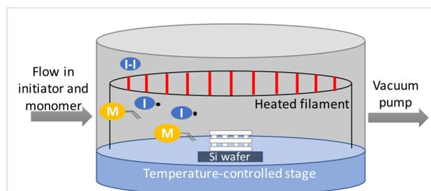
**Figure 1:** Schematic of the iCVD process. The 3D-printed substrate (white lattice) is placed on a silicon wafer piece on a temperature-controlled stage. Initiator (I-I) and monomer (M) in vapor phase are introduced into the reactor and the filament array is heated to thermally cleave the initiator.
