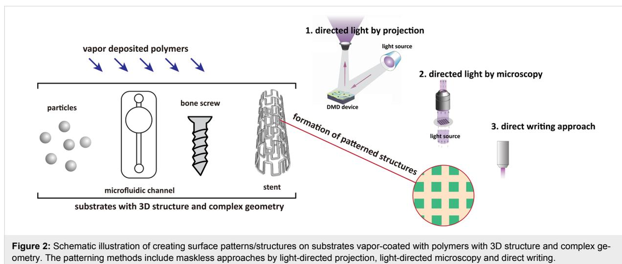
**Figure 2:** Schematic illustration of creating surface patterns/structures on substrates vapor-coated with polymers with 3D structure and complex geometry. The patterning methods include maskless approaches by light-directed projection, light-directed microscopy and direct writing.
