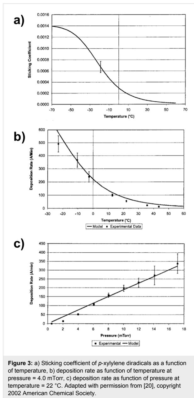
**Figure 3:** a) Sticking coefficient of *p*-xylylene diradicals as a function of temperature, b) deposition rate as function of temperature at pressure = 4.0 mTorr, c) deposition rate as function of pressure at temperature = 22 °C. Adapted with permission from [20], copyright 2002 American Chemical Society.
