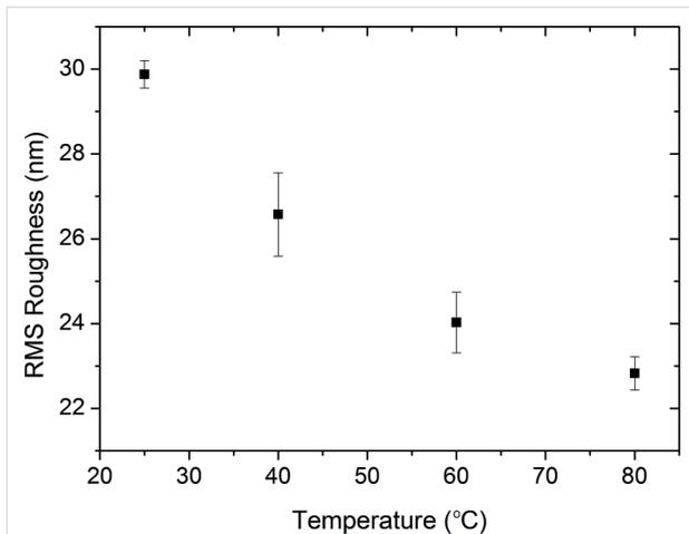
**Figure 4:** Surface roughness of PANI thin films annealed at 25, 40, 60 and 80 °C. The surface roughness of the polymer thin films decreases as a result of the increased crystallinity as the annealing temperature increases.
