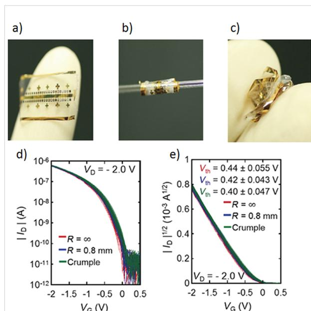
**Figure 5:** Transfer characteristics of 10 OTFTs after bending and crumpling tests: (a) Photograph of a device before mechanical tests. (b) Photograph of a device rolled onto a cylinder of 0.8 mm radius. (c) Photograph of a crumpled device. (d) and (e) Transfer characteristics of 10 OTFTs before and after bending and crumpling tests. Reprinted with permission from [33] copyright 2016 IOP Publishing Ltd.
