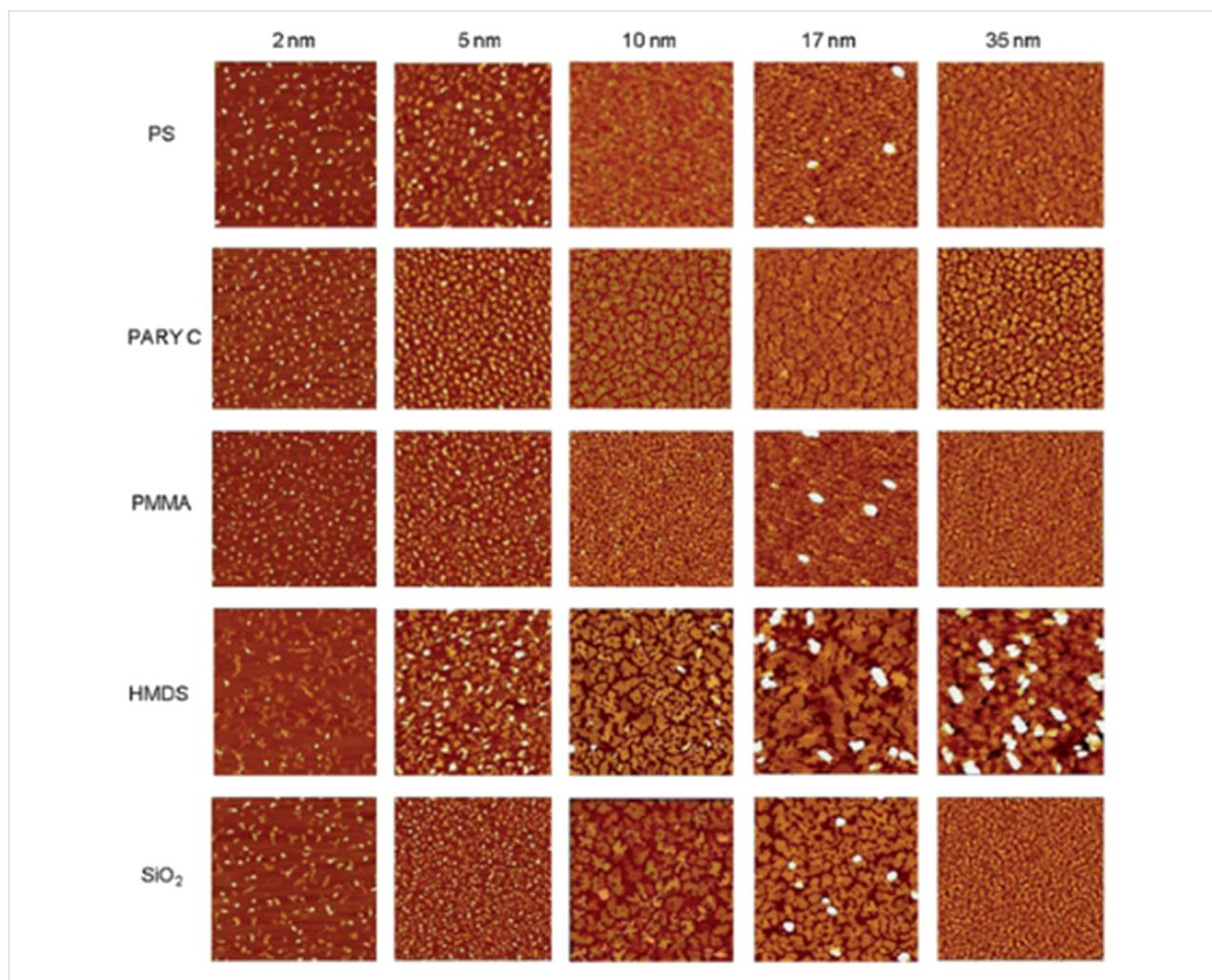
**Figure 8:**  $10\ \mu\text{m} \times 10\ \mu\text{m}$  AFM images of tetracene thin films on different dielectric surfaces at different nominal thickness. Z-scale: 50 nm. Reprinted with permission from [50], copyright 2013 Royal Society of Chemistry.
