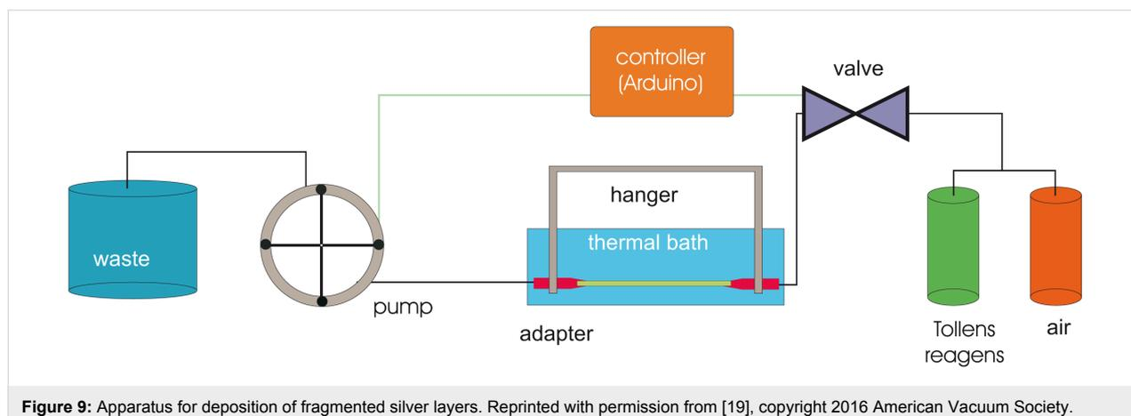
**Figure 9:** Apparatus for deposition of fragmented silver layers. Reprinted with permission from [19], copyright 2016 American Vacuum Society.
