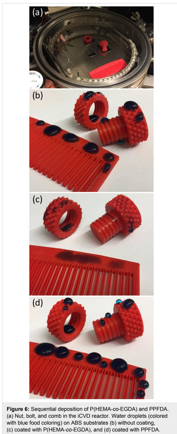
**Figure 6:** Sequential deposition of P(HEMA-co-EGDA) and PPFDA. (a) Nut, bolt, and comb in the iCVD reactor. Water droplets (colored with blue food coloring) on ABS substrates (b) without coating, (c) coated with P(HEMA-co-EGDA), and (d) coated with PPFDA.
