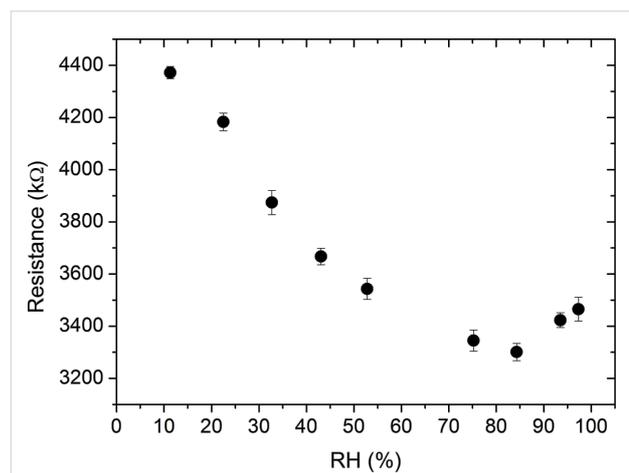
**Figure 7:** Resistance of PANI thin films as a function of the relative humidity measured using a two-point probe. The parabolic dependency is the result of the competitive effects of doping and swelling of the polymer.
