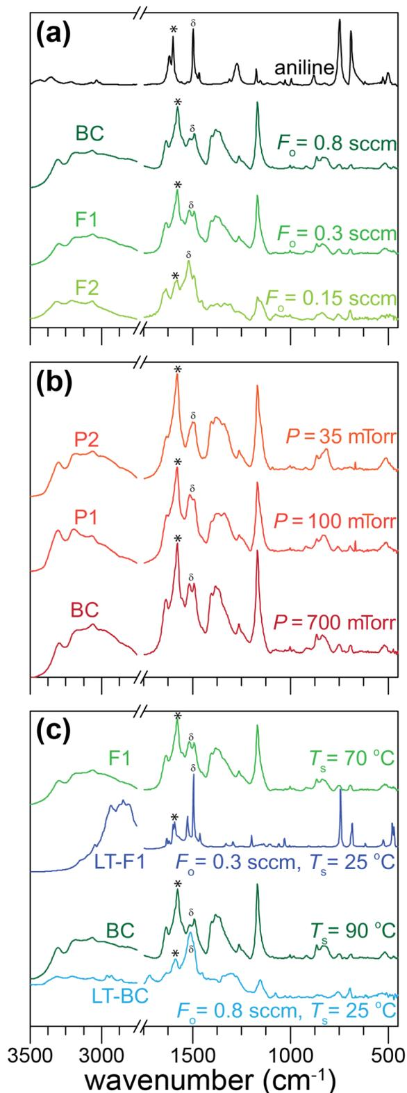
**Figure 3:** FTIR of as-deposited oCVD PANI films based on the experimental conditions in Table 1. Effect of (a) reactor pressure, (b) oxidant flow rate, and (c) substrate temperature on oCVD PANI chemistry. The quinoid and benzenoid groups are labeled by \* and  $\delta$ , respectively.
