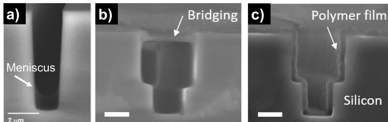
**Figure 1:** Micro-trenches with polymer coatings by a) solution with low substrate–interface energy, b) solution with high substrate–interface energy and c) iCVD (scale bar 2  $\mu\text{m}$ ). a) Reproduced with permission from [8]. Copyright 2008 John Wiley and Sons. b),c) Reproduced with permission from [9]. Copyright 2016 Massachusetts Institute of Technology.
