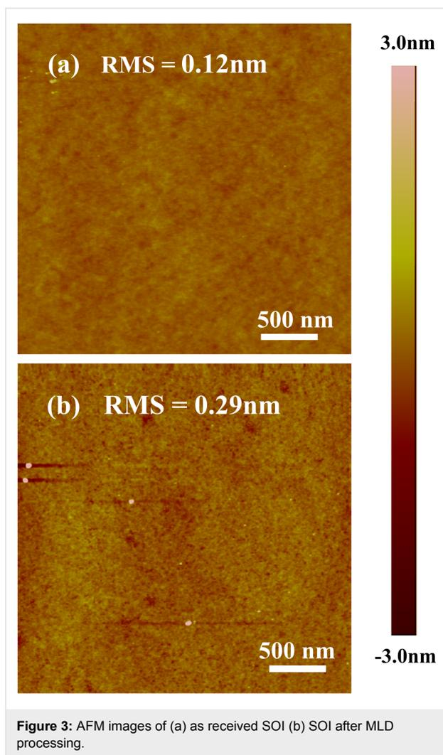
Figure 3: AFM images of (a) as received SOI (b) SOI after MLD processing.
