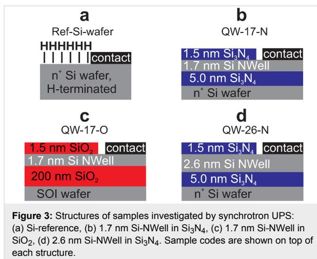
**Figure 3:** Structures of samples investigated by synchrotron UPS: (a) Si-reference, (b) 1.7 nm Si-NWell in  $\text{Si}_3\text{N}_4$ , (c) 1.7 nm Si-NWell in  $\text{SiO}_2$ , (d) 2.6 nm Si-NWell in  $\text{Si}_3\text{N}_4$ . Sample codes are shown on top of each structure.
