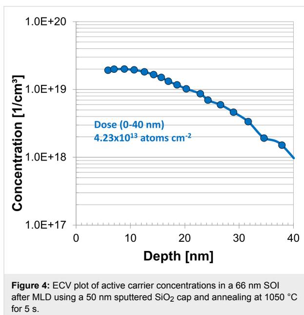
Figure 4: ECV plot of active carrier concentrations in a 66 nm SOI after MLD using a 50 nm sputtered SiO<sub>2</sub> cap and annealing at 1050 °C for 5 s.
