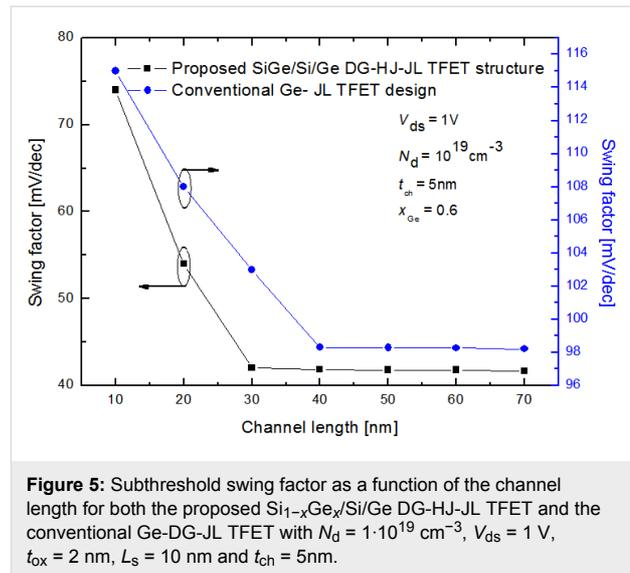
**Figure 5:** Subthreshold swing factor as a function of the channel length for both the proposed  $Si_{1-x}Ge_x/Si/Ge$  DG-HJ-JL TFET and the conventional Ge-DG-JL TFET with  $N_d = 1 \cdot 10^{19} cm^{-3}$ ,  $V_{ds} = 1 V$ ,  $t_{ox} = 2 nm$ ,  $L_s = 10 nm$  and  $t_{ch} = 5 nm$ .
