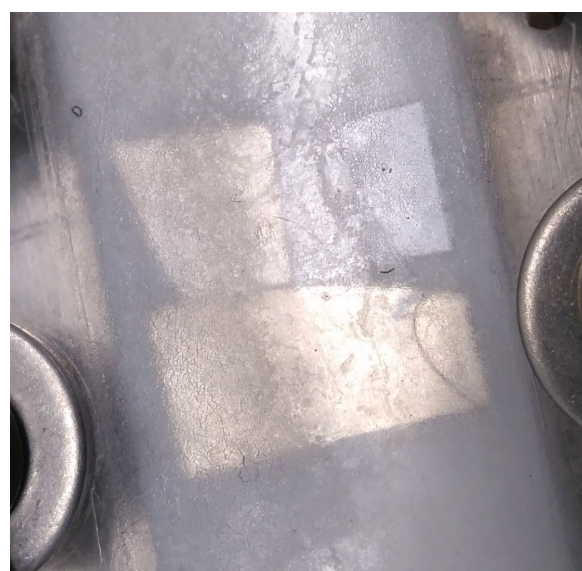
Figure 3: Samples in chamber during deposition, immediately before being taken out of the chamber. The glass slide was held in place by an acrylic block, immediately upon removal of the block the chamber unsealed and the films started reacting with air.
