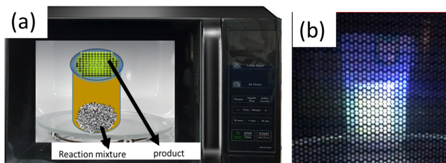
Figure 2: (a) Schematic of the synthesis in a microwave reactor, (b) plasma generated with metal particles under microwave irradiation.
