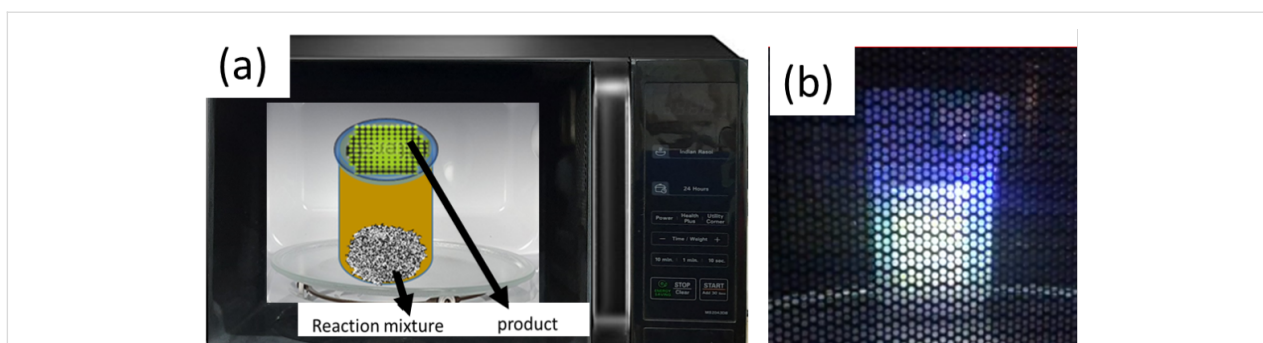
Figure 2: (a) Schematic of the synthesis in a microwave reactor, (b) plasma generated with metal particles under microwave irradiation.
