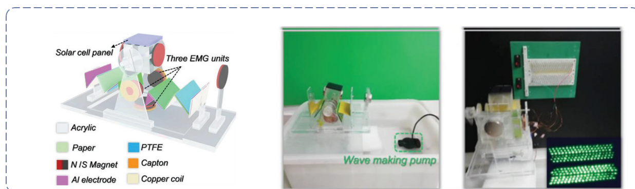
Figure 12: Harvesting water wave energy with a hybrid generator [163] Copyright © 2019 WILEY-VCH Verlag GmbH & Co. KGaA, Weinheim. Adapted with permission from Hongmei Yang et al., "A Nonencapsulated Pendulum-Like Paper-Based Hybrid Nanogenerator for Energy Harvesting", Advanced Energy Materials, John Wiley and Sons.
