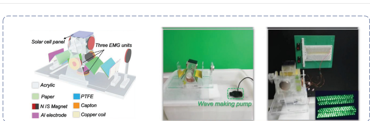
Figure 12: Harvesting water wave energy with a hybrid generator [163] Copyright © 2019 WILEY-VCH Verlag GmbH & Co. KGaA, Weinheim. Adapted with permission from Hongmei Yang et al., “A Nonencapsulative Pendulum-Like Paper-Based Hybrid Nanogenerator for Energy Harvesting”, Advanced Energy Materials, John Wiley and Sons.
