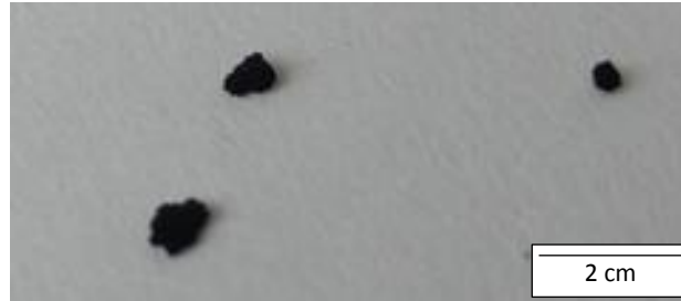
Figure S4: Agglomerates of decorated carbon nanotubes resulting from using the first decoration approach.
