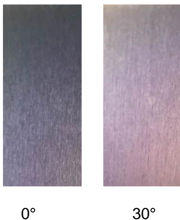
Figure S1: The color variation of the S3 sample under incident light at different angles (the sunlight perpendicular to the sample surface is designated to the incident light angle equal to 0^\circ ).
