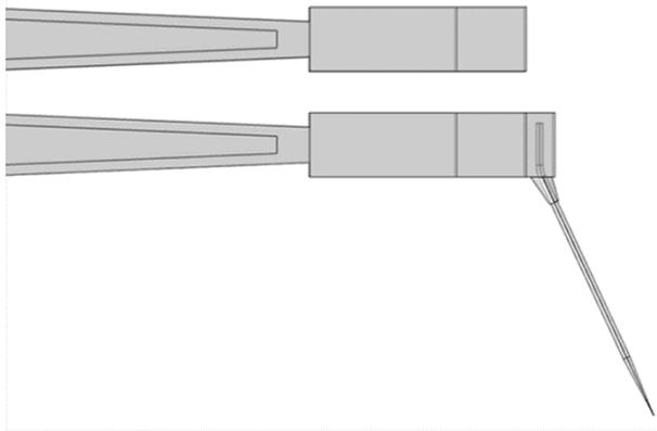
**Figure S1:** Schematic diagram of the simulation model with an added cone of glue around the tip.
