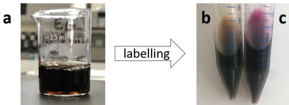
Figure S3: Pictures of FITC- and RhBITC-BSA/PDA NPs suspensions after dialysis with a 8–10 kDa cut-off membrane. (a) FITC-BSA/PDA NPs. (b) RhBITC-BSA/PDA NPs (c).
