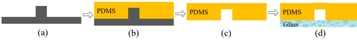
Scheme S1: Four steps of the fabrication process of a microfluidic device: (a) 3D printing of the mold; (b) PDMS casting; (c) PDMS peel-off; and (d) PDMS-glass bonding.
