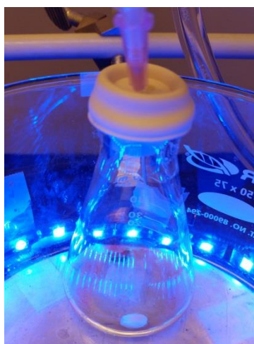
Figure S6: Thin film deposition experiment in progress. This setup was used for particle lithography experiments. Note that the stirbar (at bottom of the image) has been physically separated from the Au substrate (near the LED strip on the other side of the Erlenmeyer flask) to prevent perturbation of the substrate.
