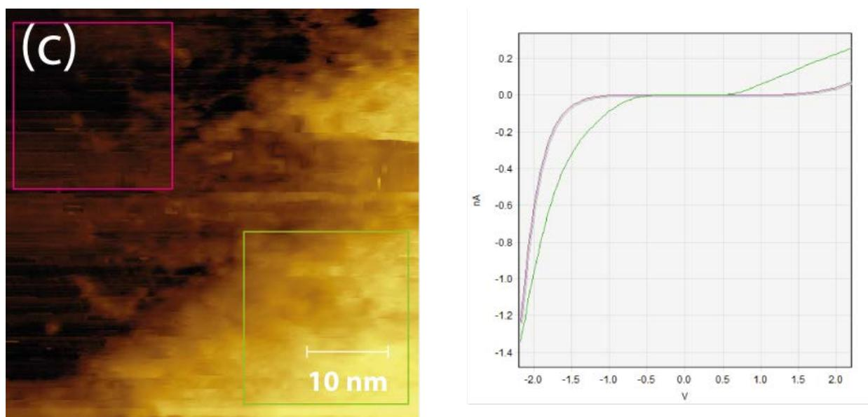
**Figure S2:** (a) silicon clusters on top of MoS<sub>2</sub> after deposition of 1.4 monolayers of silicon. The purple and green boxes indicate the locations where a grid scan is performed. Each grid did consist of 100 curves. (b) The average of the recorded  $I(V)$  curves on top of the cluster (green) is significantly different from the average of the curves recorded on MoS<sub>2</sub> (purple).
