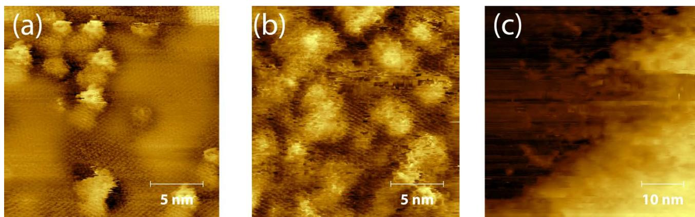
**Figure S1:** Topography of the MoS<sub>2</sub> surface as a function of the amount of deposited silicon. (a) 0.2 monolayers. Here transitions between hills and valleys are visible. The recurring feature is a tip image. (b) 0.8 monolayers. The sample becomes rougher and more difficult to image. (c) 1.4 monolayers. Silicon clusters are visible on top of the MoS<sub>2</sub>.
