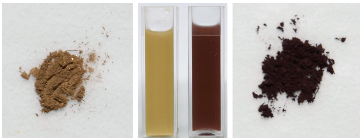
Figure S2: Images of Ag@TiO 2 (left) and Au@TiO 2 (right) core-shell nanostructures in form of powders and water suspensions.
