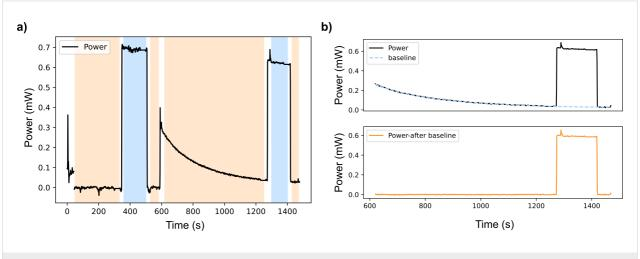
Figure 3: A visual example of the power determination. a) Power without any elements (left) and with insulated jacket and cuvette (right side, the change in baseline is noticeable), b) power with insulated jacket and cuvette after baseline subtraction.
