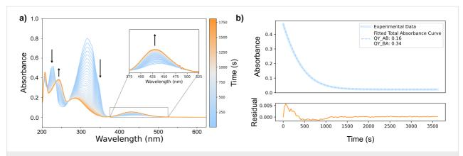
Figure 4: UV–vis absorption spectra of azobenzene upon irradiation at 340 nm (methanol solution, 20 °C). a) Evolution of spectra over time under irradiation and b) absorption at 340 nm over time, with fitted total absorbance curve obtained from Equation 5. The curve was obtained from entry 5 of Table S2 (Supporting Information File 1).
