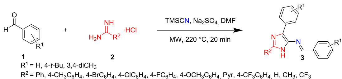
Scheme 1: General scheme for the synthesis of imidazoles with various amidines.
