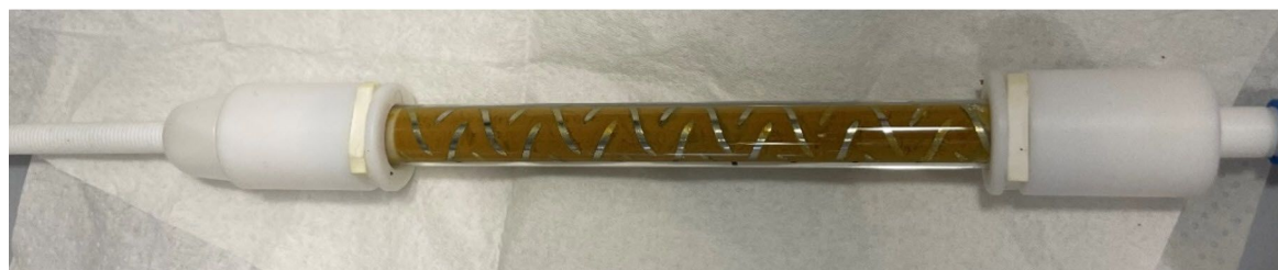
Figure 6: Photo of the packed column with a helical static mixer (polished SS316, 10 cm length, 15 mixing elements L/D = 1.04 from Stamixco AG).
