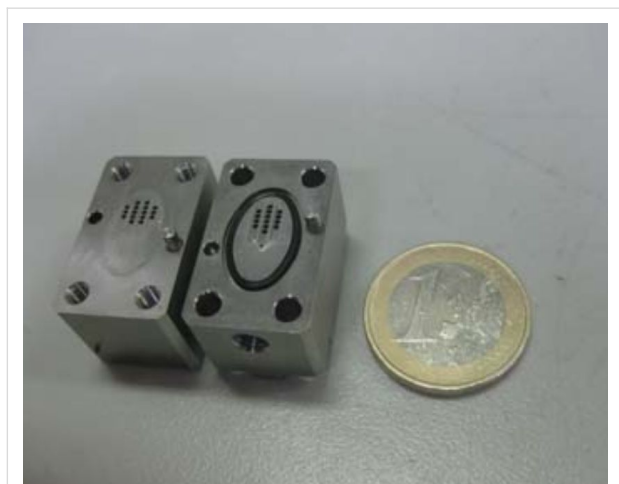
Figure 1: Hastelloy-made micromixer (MiChS \beta -150H).
