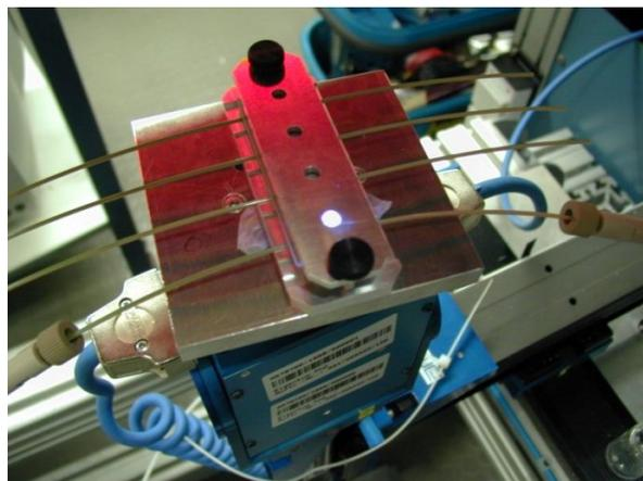
**Figure 6:** The miniaturized photoreactor (PEEK) during photolysis.
