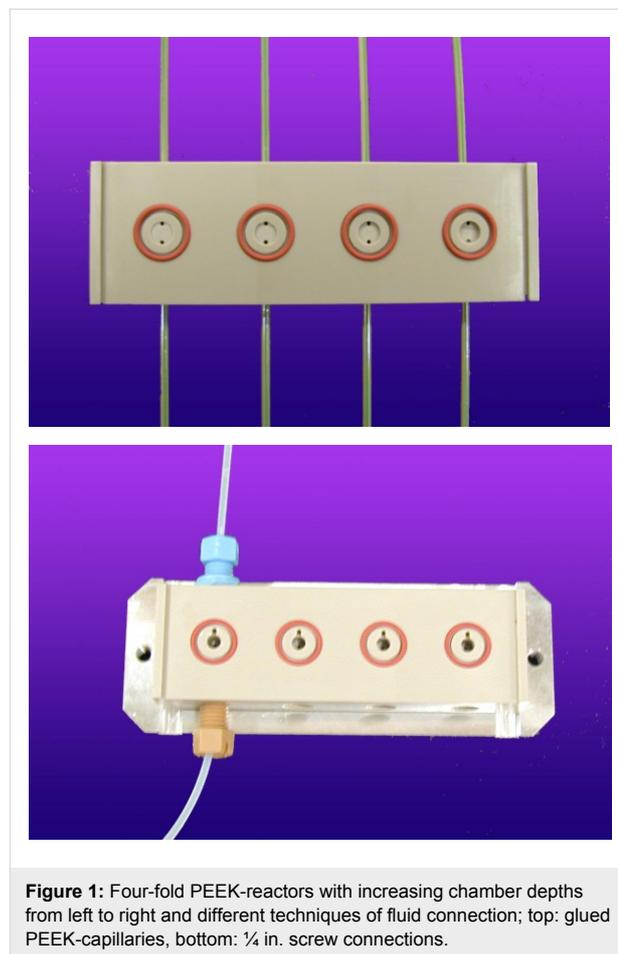
**Figure 1:** Four-fold PEEK-reactors with increasing chamber depths from left to right and different techniques of fluid connection; top: glued PEEK-capillaries, bottom:  $\frac{1}{4}$  in. screw connections.
