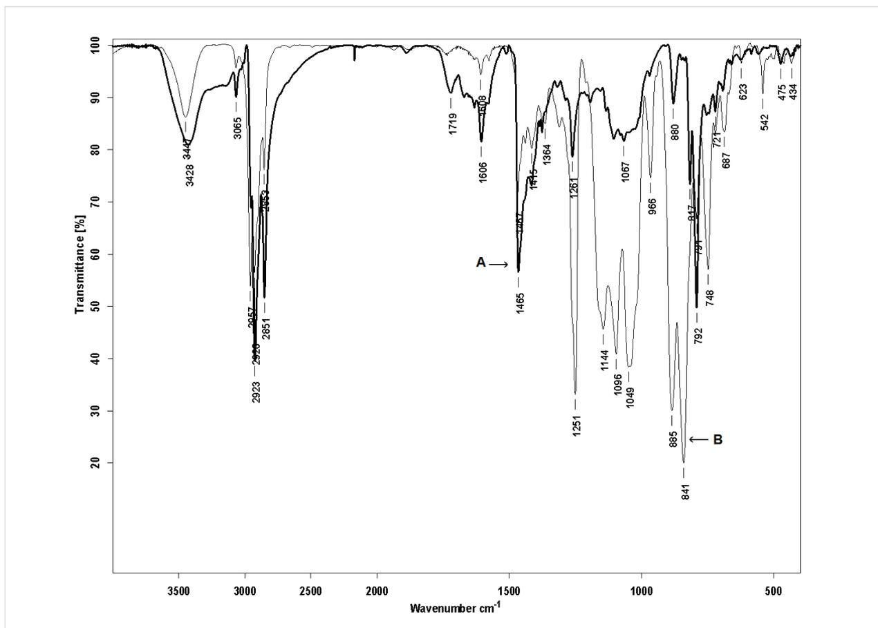
Figure 2: FTIR spectra (KBr pellet) of PDOF-BT (A) and PDOF-BTc (B) copolymers.
