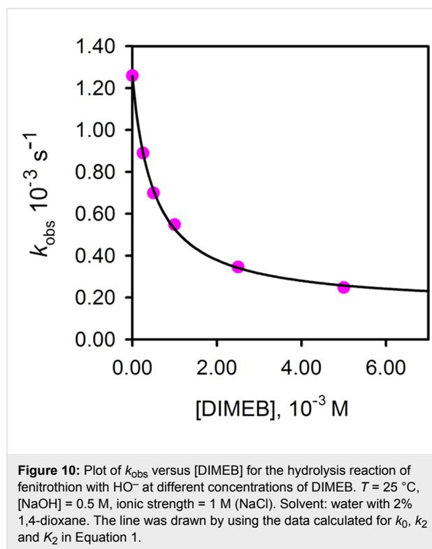
**Figure 10:** Plot of  $k_{\text{obs}}$  versus [DIMEB] for the hydrolysis reaction of fenitrothion with  $\text{HO}^-$  at different concentrations of DIMEB.  $T = 25^\circ\text{C}$ ,  $[\text{NaOH}] = 0.5 \text{ M}$ , ionic strength = 1 M (NaCl). Solvent: water with 2% 1,4-dioxane. The line was drawn by using the data calculated for  $k_0$ ,  $k_2$  and  $K_2$  in Equation 1.
