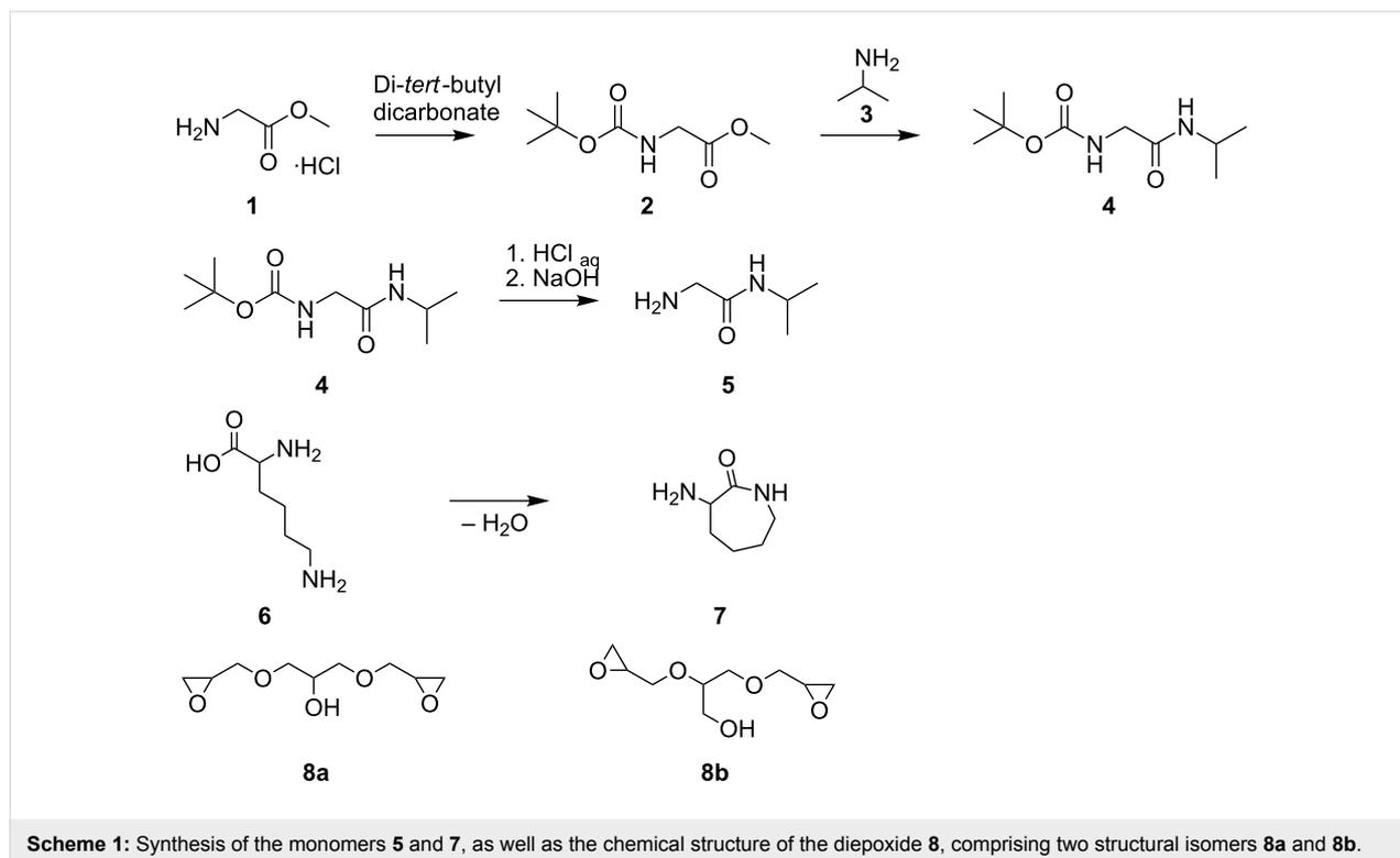
**Scheme 1:** Synthesis of the monomers **5** and **7**, as well as the chemical structure of the diepoxide **8**, comprising two structural isomers **8a** and **8b**.
