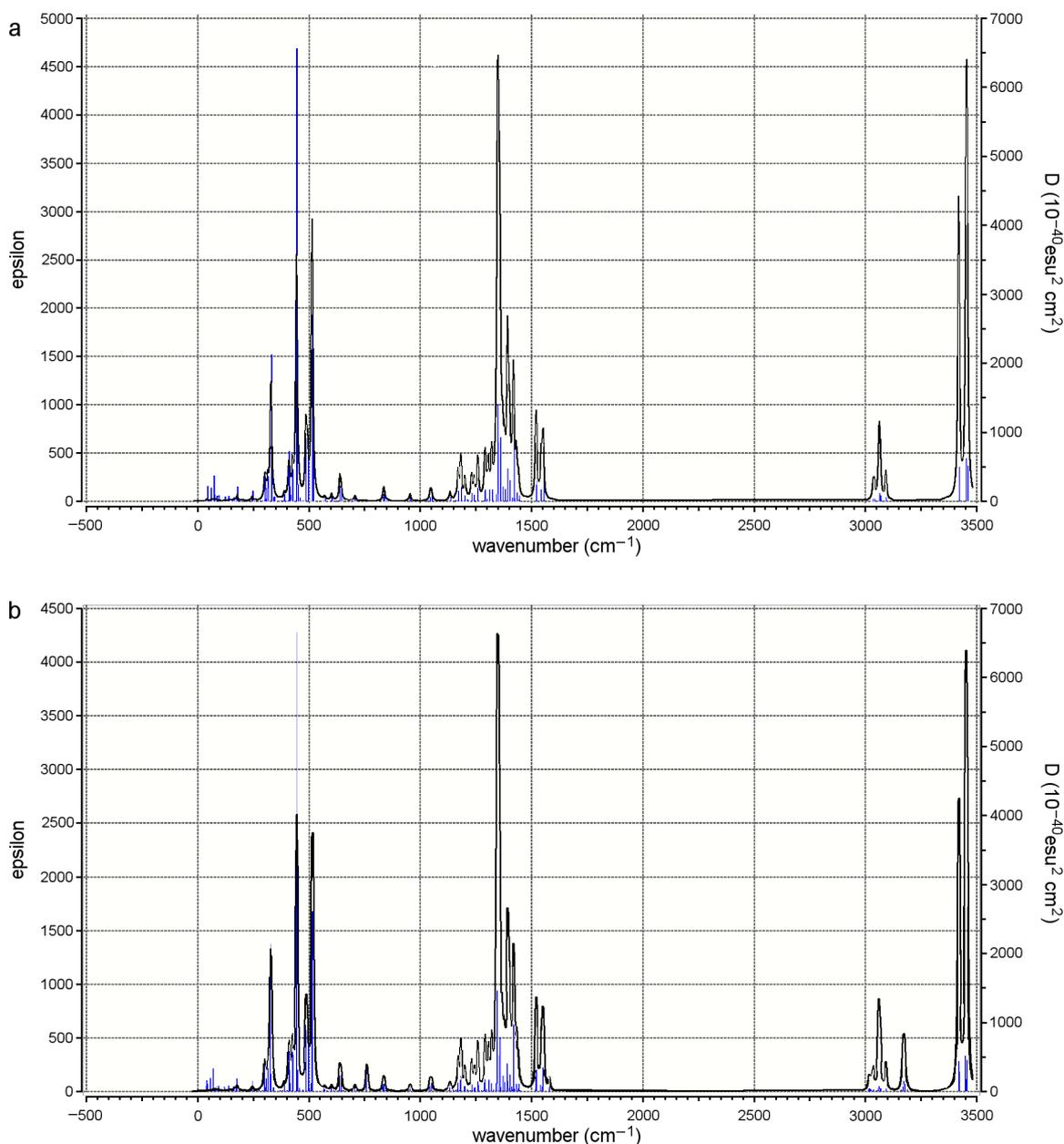
**Figure 3:** (a) AM1 calculated IR spectra of BCDO23rO6l empty and (b) the BCDO23rO6l/benzene inclusion complex with benzene in a parallel orientation.
