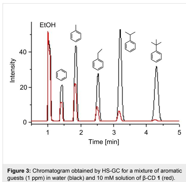
**Figure 3:** Chromatogram obtained by HS-GC for a mixture of aromatic guests (1 ppm) in water (black) and 10 mM solution of  $\beta$ -CD **1** (red).
