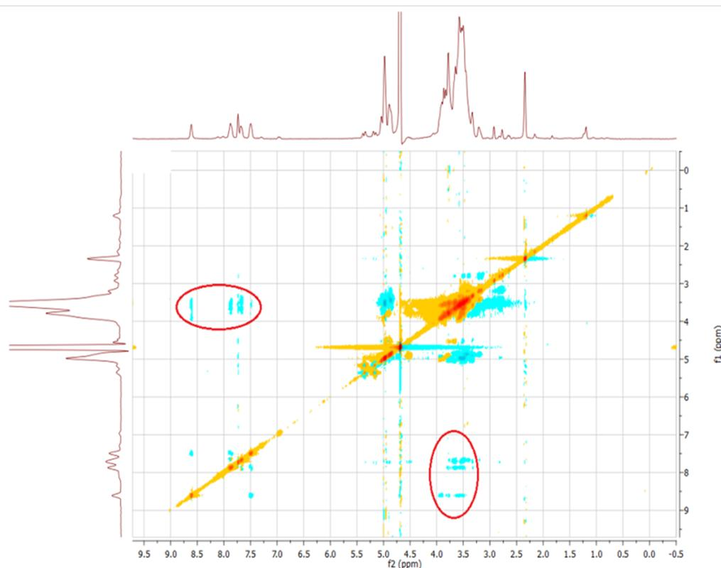
**Figure 1:**  $^1\text{H}$  NMR-ROESY spectrum of the modified CD **3**.
