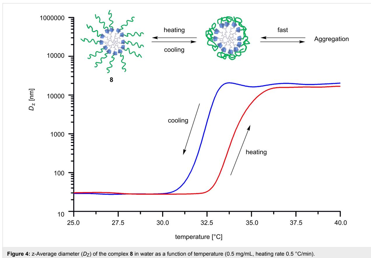
**Figure 4:** z-Average diameter ( $D_z$ ) of the complex **8** in water as a function of temperature (0.5 mg/mL, heating rate 0.5 °C/min).
