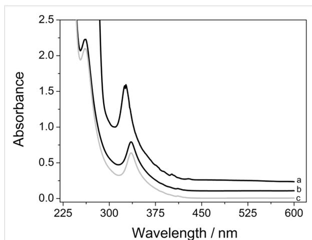
**Figure 2:** UV-vis spectra of (a)  $C_{60}$  solution in THF, (b) aqueous solutions of  $C_{60}$  with 6 mM  $\gamma$ -CD thioether **5** before centrifugation, and (c) after centrifugation (13,000 rpm) for 60 min. The absorbance intensities of (a) and (b) are shifted by 0.2 and 0.1 AU, respectively.
