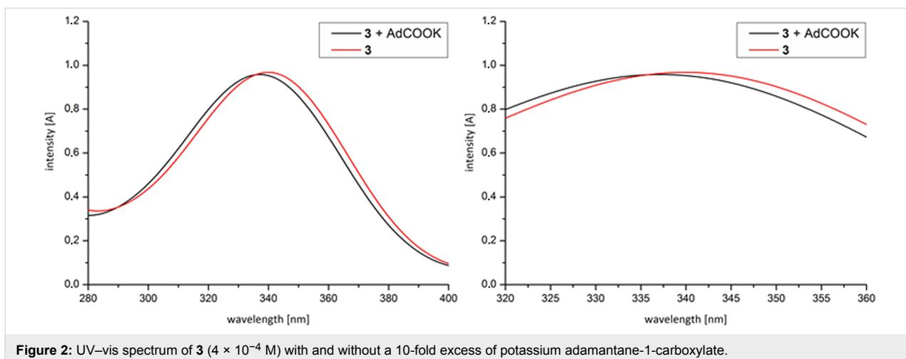
**Figure 2:** UV-vis spectrum of **3** ( $4 \times 10^{-4}$  M) with and without a 10-fold excess of potassium adamantane-1-carboxylate.
