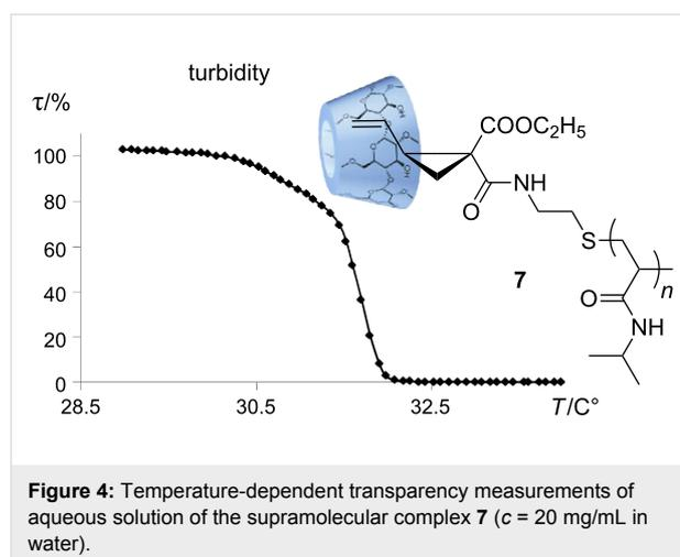
**Figure 4:** Temperature-dependent transparency measurements of aqueous solution of the supramolecular complex **7** ( $c = 20$  mg/mL in water).
