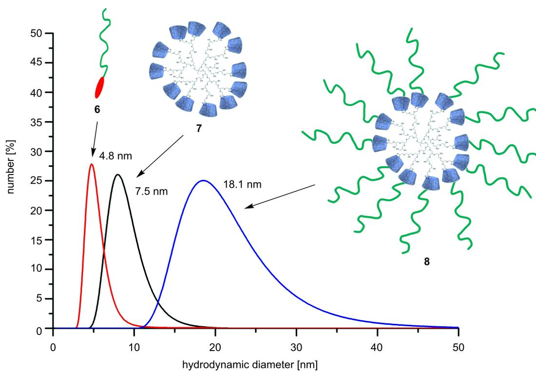
**Figure 3:** Hydrodynamic diameters of **6**, **7** and **8** (1 mg/mL) at 20 °C.
