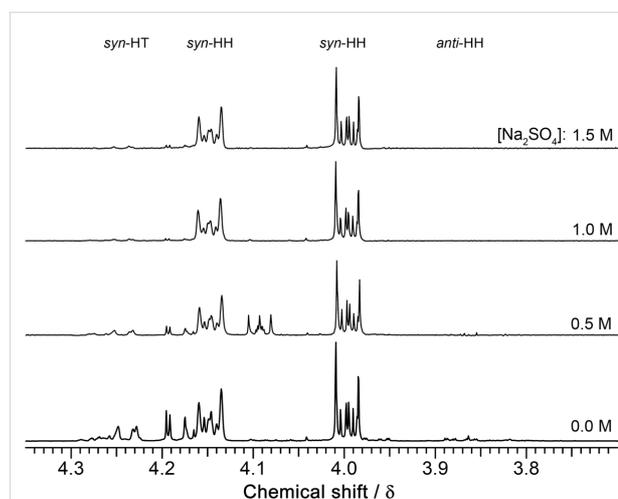
**Figure 6:** Partial <sup>1</sup>H NMR of the photodimers formed after irradiation of **COU** at various concentrations of Na<sub>2</sub>SO<sub>4</sub> in the presence of 6 mM  $\gamma$ -CD thioether **2**.
