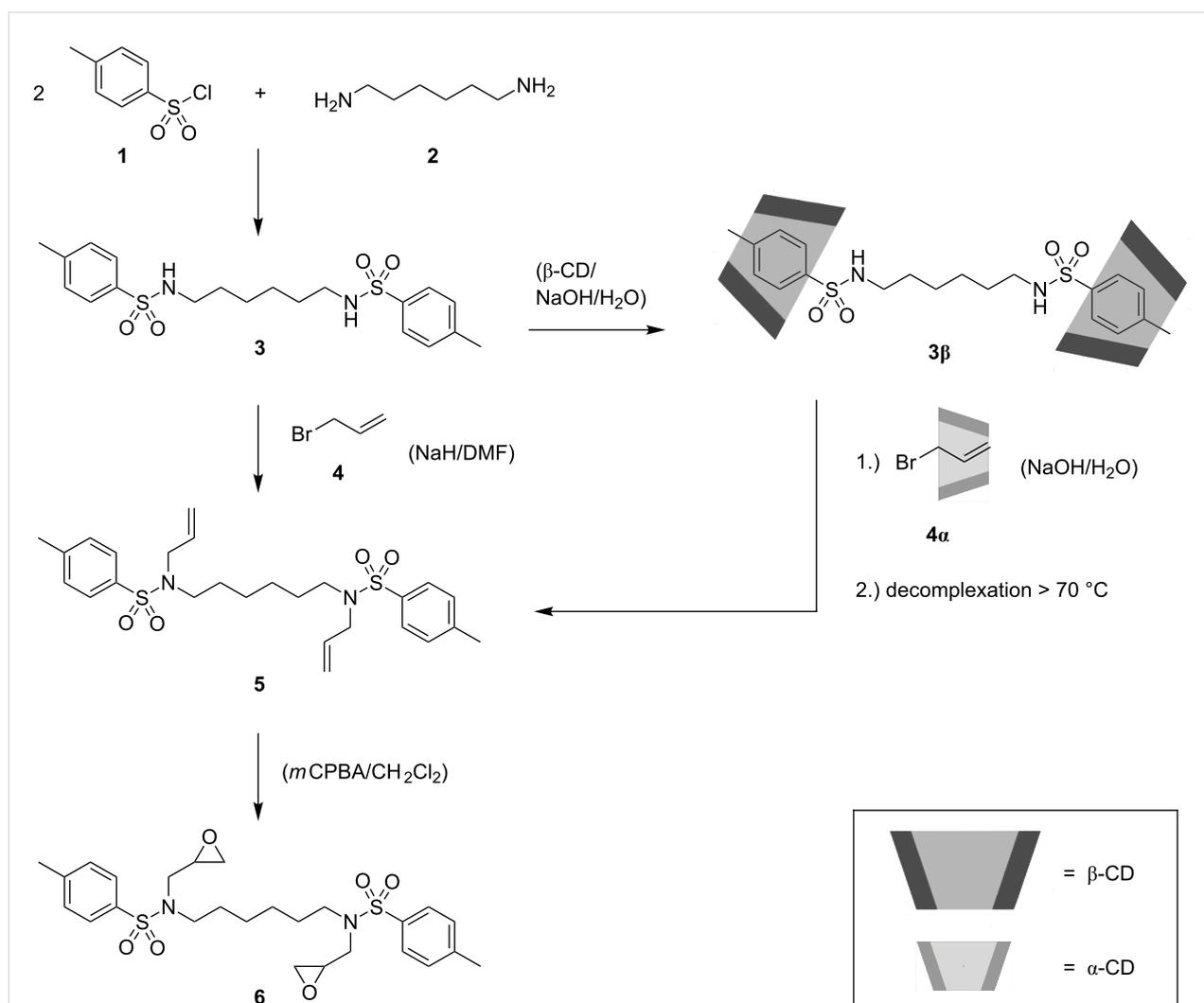
**Scheme 1:** Synthesis of sulfonamide **3**, *N*-alkylation of **3** in organic solution and of CD-complex (**3 $\beta$** ) in aqueous phase to obtain **5** and the subsequent epoxidation with *m*-chloroperbenzoic acid (*m*CPBA) to yield product **6**.
