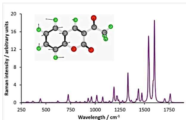
**Figure 2:** The Raman spectrum of 3-acetylcoumarin (**1**) generated using Gaussian 09 [40] at the B3LYP/6-31g(d) level of theory. The inset molecule illustrates the stretching mode responsible for the signal calculated at  $1602\text{ cm}^{-1}$  (actual:  $1608\text{ cm}^{-1}$ ).
