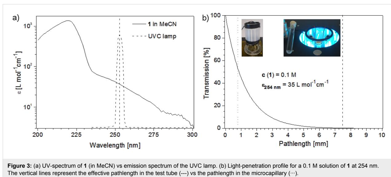
**Figure 3:** (a) UV-spectrum of **1** (in MeCN) vs emission spectrum of the UVC lamp. (b) Light-penetration profile for a 0.1 M solution of **1** at 254 nm. The vertical lines represent the effective pathlength in the test tube (---) vs the pathlength in the microcapillary (···).
