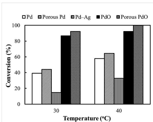
**Figure 3:** Influence of temperature on the conversion of 0.01 M *p*-nitrophenol with 0.1 M formic acid at 30 °C and 40 °C. Tubular reactors coated with Pd, PdO, Pd-Ag, porous Pd or porous PdO were applied for demonstration of the catalytic activity. All experiments were conducted with 14.7 s residence time.
