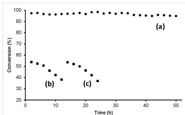
**Figure 3:** Conversion of cinnamaldehyde oxime ( $1, 25 \mu\text{M}$  in acetonitrile) by continuously running the catalytic microreactor: (a) for 50 h with 13 min residence time, (b) for 12 h with 78 s residence time, (c) also for 12 h with 78 s residence time but after reactivating the microreactor with  $\text{GaCl}_3$ .
