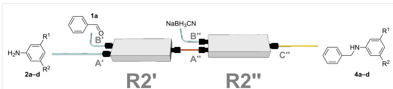
**Figure 7:** Representation of the setup for the two-step flow reaction employed in this work. The first reactor (R2') is used to synthesize the imines under previously optimized conditions. The product is then directly introduced into the next reactor (R2'') and mixed with the reducing agent to produce the secondary amine.
