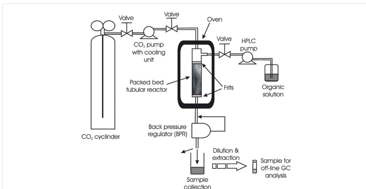
**Figure 2:** Schematic diagram of the continuous flow system. The reactor shown is the 3.9 mm i.d. PFR. For the 1 mm i.d. reactor this was a coil of the 300 cm or 100 cm tube according to the specific reaction.
