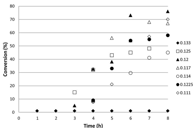
**Figure 4:** Total conversion of 4-iodoanisole at 155 °C and 200 bar as a function of reactor run time for different combined flow rates and therefore residence times. The values of the total flow rates given in the legend are mL min<sup>-1</sup>.
