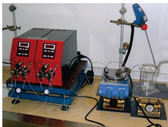
Figure 4: Photograph of the experimental setup for the synthesis of alkyl-nitropyrazoles. IMM's SIMM-V2 micromixer was used to ensure better mixing at the cost of pressure drop. Reproduced with permission from [31]. Copyright 2009 The American Chemical Society.
