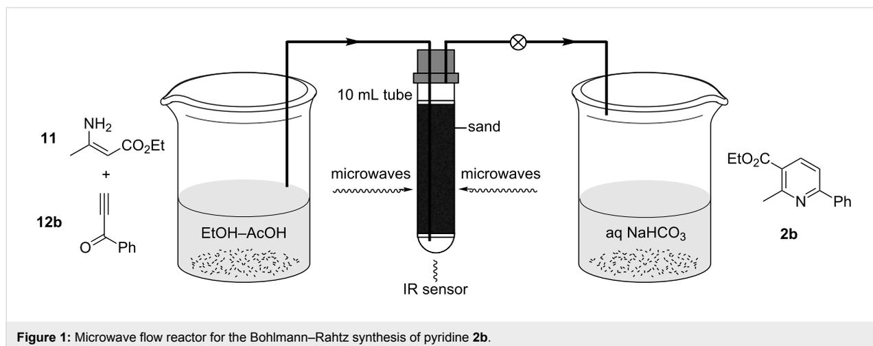
Figure 1: Microwave flow reactor for the Bohlmann–Rahtz synthesis of pyridine **2b**.
