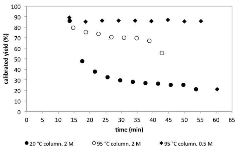
**Figure 3:** Comparing the long-term stability of the  $\text{Al}_2\text{O}_3$  and 3 Å MS columns when the  $\text{Al}_2\text{O}_3$  column temperature (20 °C and 95 °C) and Knoevenagel reaction concentration (2.0 M and 0.50 M) are varied. The time between 0 and 13 min was the equilibration period.
