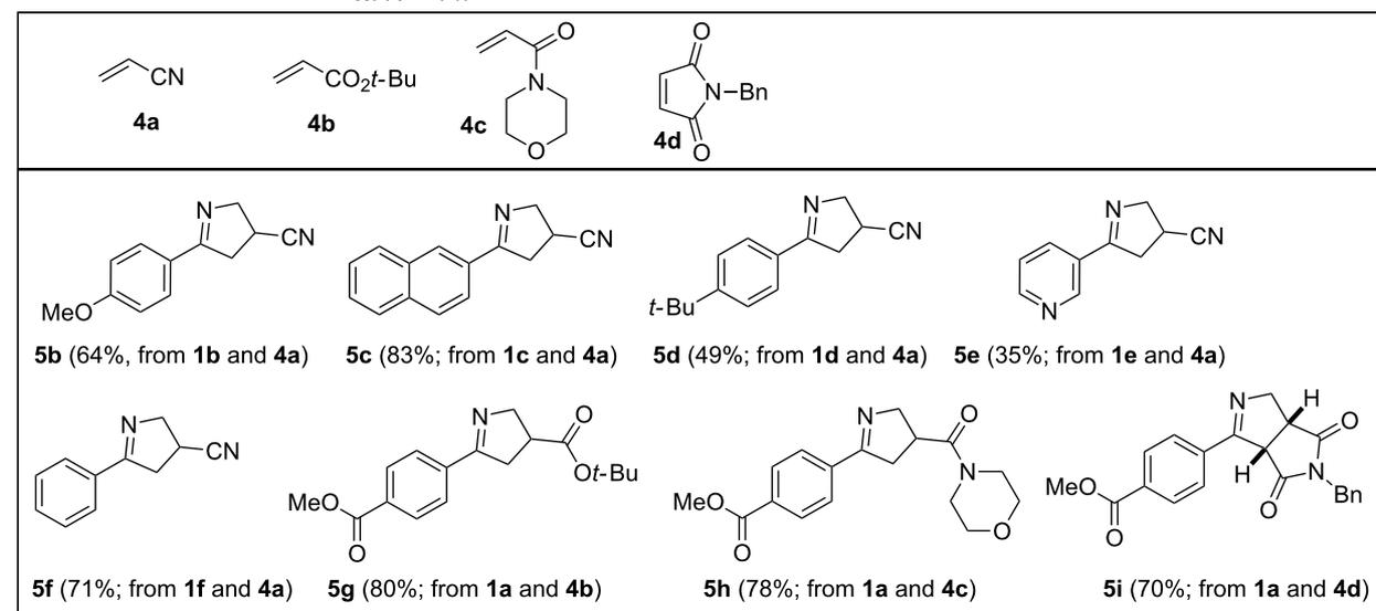
**Scheme 4:** Photoinduced cycloadditions of vinyl azides **1a–f** and electron-deficient alkenes **4a–d**. All experiments were conducted at room temperature in a photochemical flow-reactor (see above) using Teflon (FEP) tubing (volume: 5.5 mL, inner diameter = 0.75 mm) at a concentration of 0.05 M in CH<sub>3</sub>CN; isolated yields are given.
