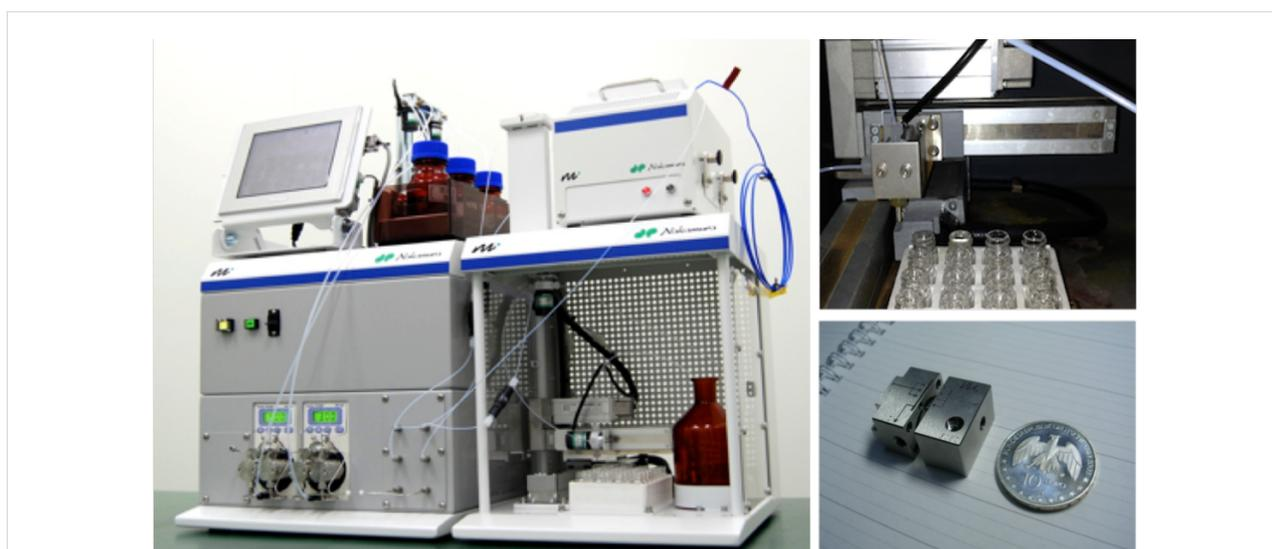
**Figure 1:** Pictures of the flow microreactor system (MiChS® System X-1), a micromixer (MiChS β-150, channel width: 150 μm), and a fraction collector used for this study.
