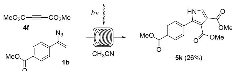
**Scheme 6:** Photoinduced cycloaddition of vinyl azide **1b** and alkyne **4f**. The experiment was conducted at room temperature in a photochemical flow-reactor (see above) using Teflon (FEP) tubing (volume: 5.5 mL, inner diameter = 0.75 mm) at a concentration of 0.05 M in CH<sub>3</sub>CN.
