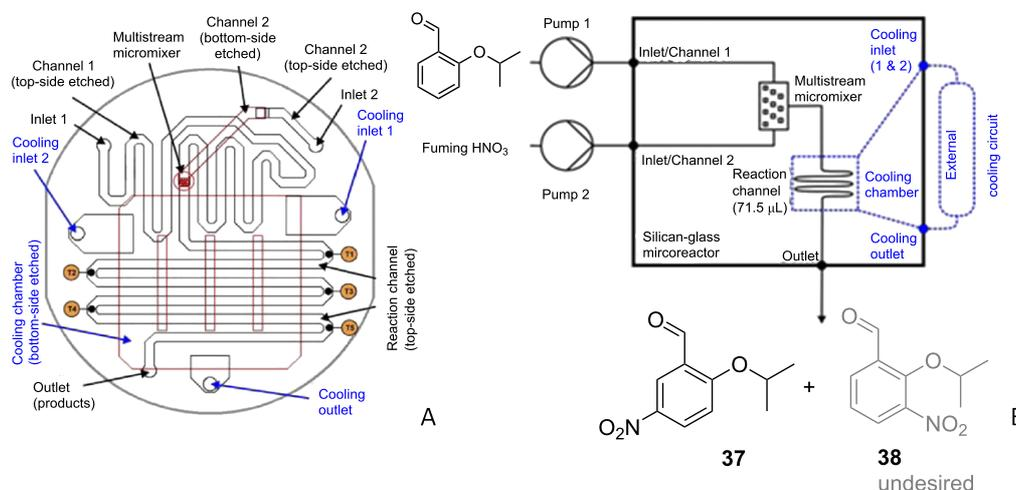
**Figure 6:** Silicon-glass microreactor by Knapkiewicz et al. [37]. (A) Layout of the microreactor with a built-in micromixer, (B) schematic of the experimental setup. Reproduced with permission from [37] Copyright 2012 The American Chemical Society.
