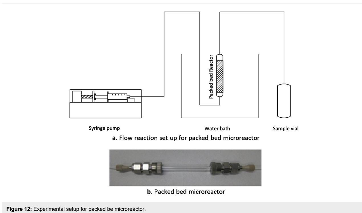
Figure 12: Experimental setup for packed be microreactor.
