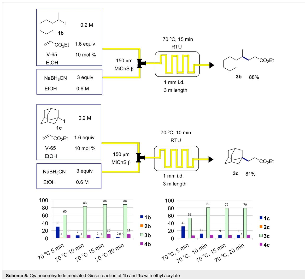
**Scheme 5:** Cyanoborohydride mediated Giese reaction of **1b** and **1c** with ethyl acrylate.
