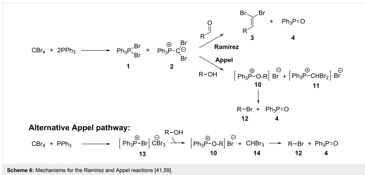
**Scheme 6:** Mechanisms for the Ramirez and Appel reactions [41,59].
