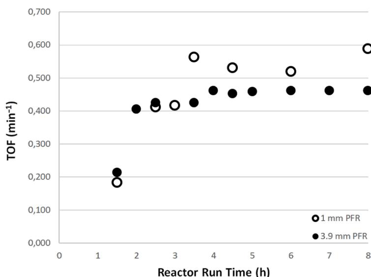
**Figure 8:** TOF values for the 1 mm (o) and 3.9 mm (●) PFRs at a total flow rate of 0.12 mL min<sup>-1</sup>, 155 °C and 200 bar for the reaction of 4-iodoanisole with methyl acrylate.
