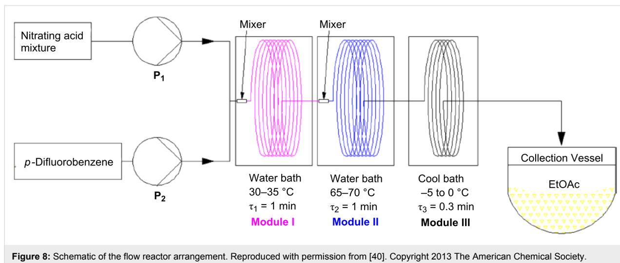
**Figure 8:** Schematic of the flow reactor arrangement. Reproduced with permission from [40]. Copyright 2013 The American Chemical Society.
