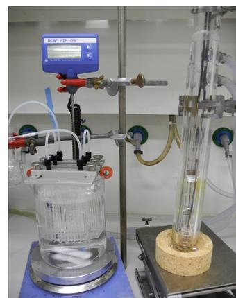
**Scheme 2:** Experimental setup of continuous-flow photocyclization–reduction cascade.
