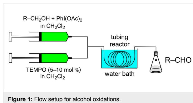
Figure 1: Flow setup for alcohol oxidations.
