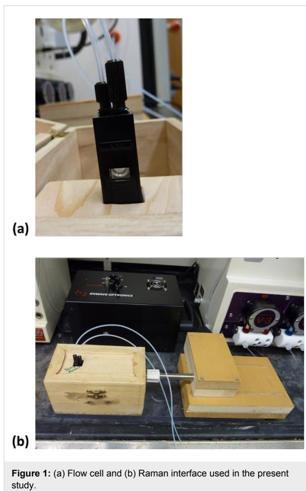
**Figure 1:** (a) Flow cell and (b) Raman interface used in the present study.
