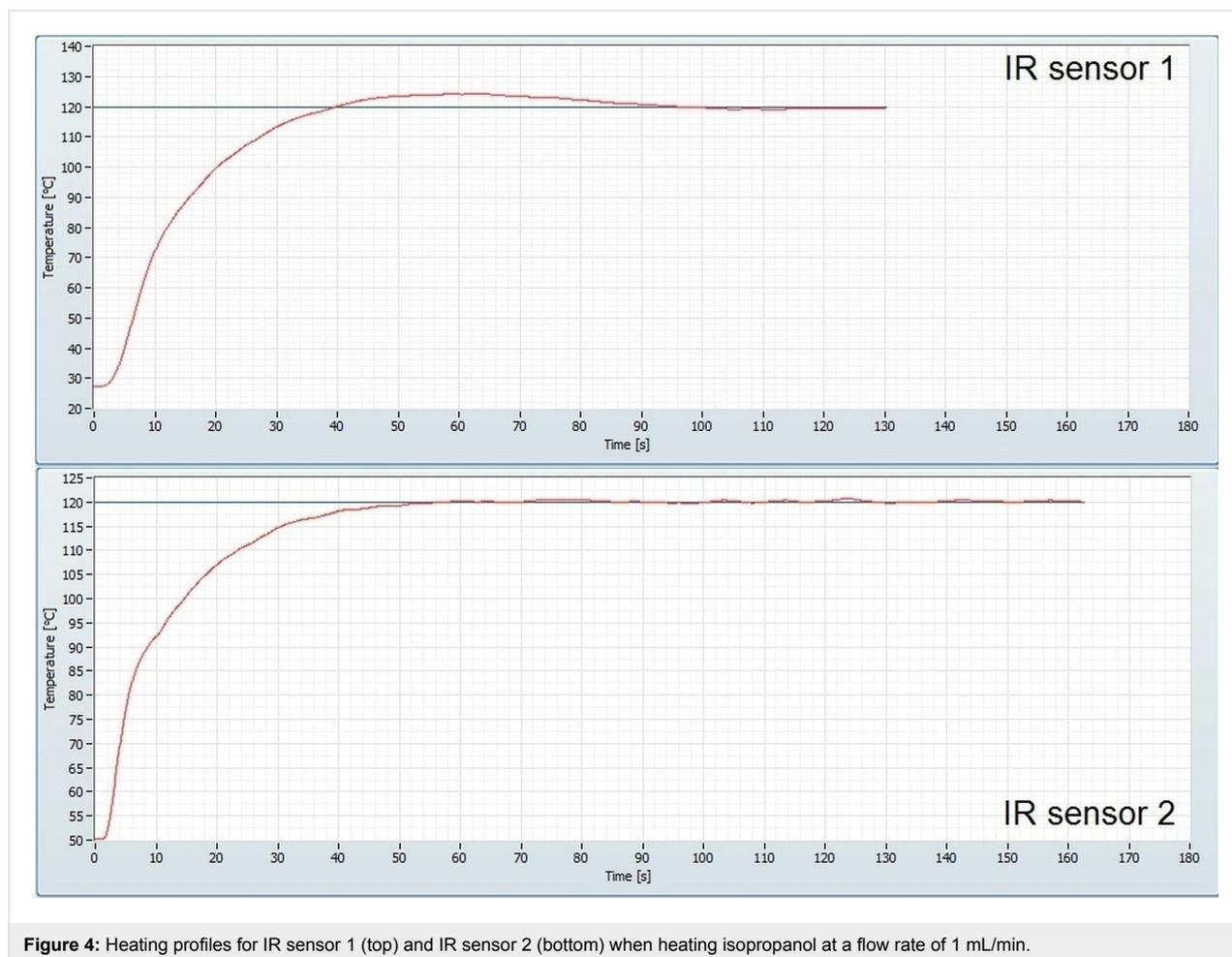
**Figure 4:** Heating profiles for IR sensor 1 (top) and IR sensor 2 (bottom) when heating isopropanol at a flow rate of 1 mL/min.
