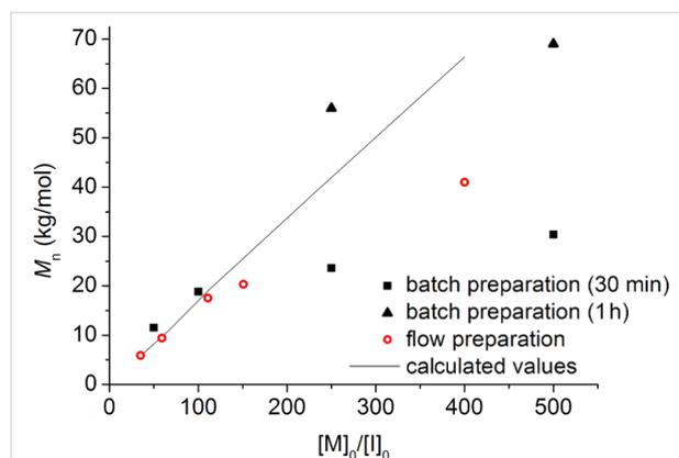
**Figure 3:** Plot of number-average molecular weight, *M*<sub>n</sub>, versus monomer-catalyst ratio [M]<sub>0</sub>/[I]<sub>0</sub> for batch and flow samples prepared with Ni(dppp)Cl<sub>2</sub> catalyst dissolved in *o*-DCB (see Table 2 for experimental data).
