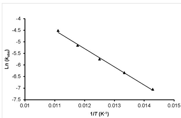
**Figure 2:** Arrhenius plot for the dehydration of cinnamaldehyde oxime (**1**).
