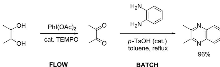
**Scheme 1:** Oxidation–condensation sequence in the synthesis of 2,3-dimethylquinoxaline.
