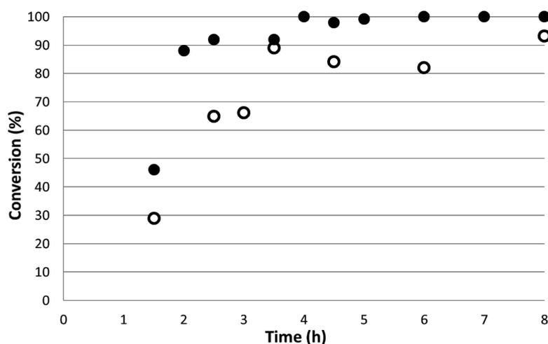
**Figure 7:** Comparison of conversion as a function of reactor run time for the reaction of methyl acrylate in the 1 mm × 300 cm (o) and 3.9 mm × 9 cm (●) plug flow reactors over the Pd-SiO<sub>2</sub> catalyst.
