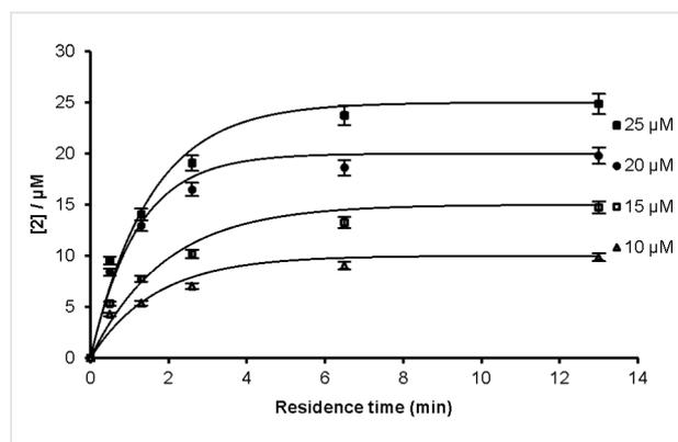
**Figure 1:** Gallium-catalyzed formation of nitrile **2** at 90 °C and 5 atm pressure.
