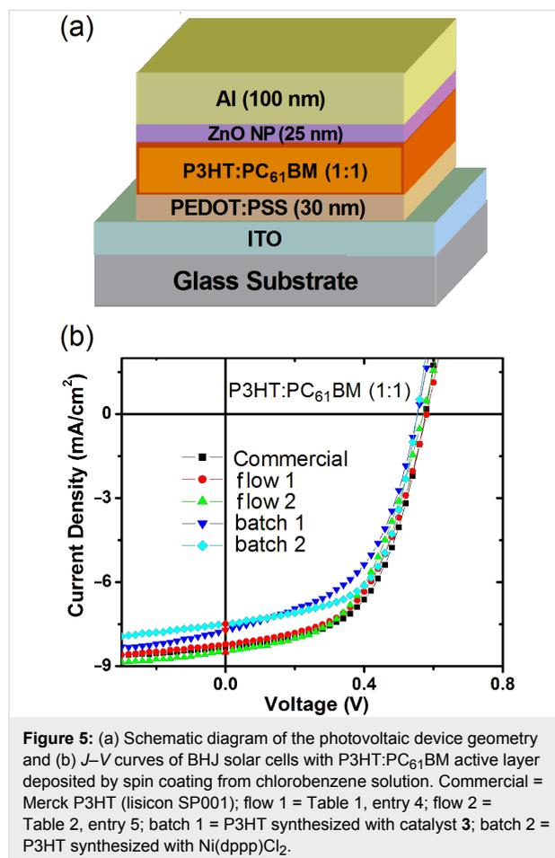
**Figure 5:** (a) Schematic diagram of the photovoltaic device geometry and (b)  $J$ – $V$  curves of BHJ solar cells with P3HT:PC<sub>61</sub>BM active layer deposited by spin coating from chlorobenzene solution. Commercial = Merck P3HT (lisicon SP001); flow 1 = Table 1, entry 4; flow 2 = Table 2, entry 5; batch 1 = P3HT synthesized with catalyst **3**; batch 2 = P3HT synthesized with Ni(dppp)Cl<sub>2</sub>.
