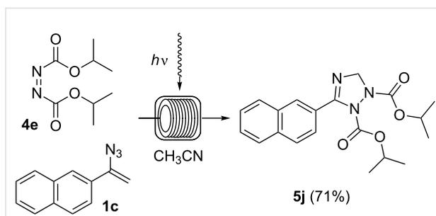
**Scheme 5:** Photoinduced cycloaddition of vinyl azide **1c** and diisopropyl azodicarboxylate (**4e**). The experiment was conducted at room temperature in a photochemical flow-reactor (see above) using Teflon (FEP) tubing (volume: 5.5 mL, inner diameter = 0.75 mm) at a concentration of 0.05 M in CH<sub>3</sub>CN.
