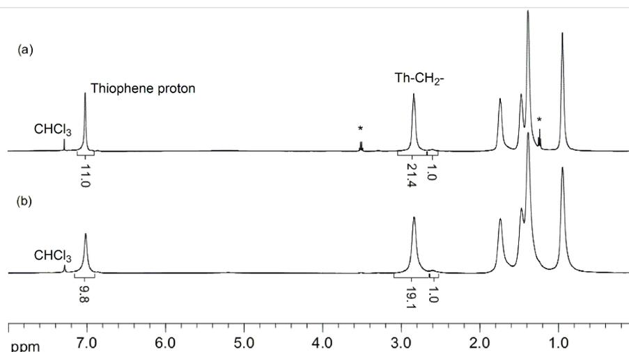
**Figure 4:** <sup>1</sup>H NMR (CDCl<sub>3</sub>, 500 MHz) spectra of P3HT samples prepared in (a) flow and (b) batch show comparable regioregularity of approximately 95% for both processes. P3HT prepared in flow ( $M_n$  = 20 kg/mol) and in batch ( $M_n$  = 17 kg/mol) (\* designates residual solvent).
