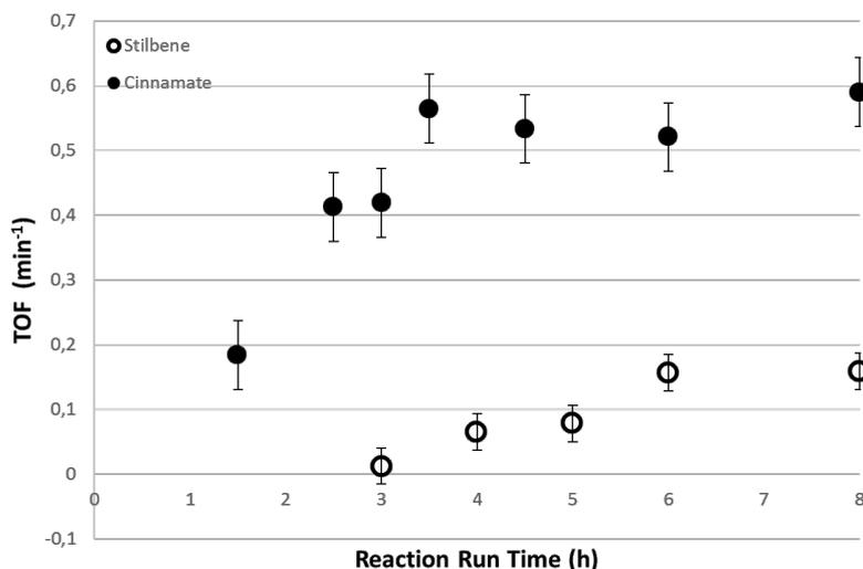
**Figure 9:** Turnover frequencies of the Heck reactions at 155 °C using styrene (o) as combined isomeric products, and methyl acrylate (●) as a function of reactor run time for the 1 mm internal diameter plug flow reactors.
