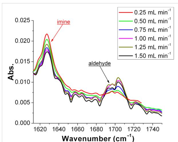
**Figure 6:** Comparison of the IR spectra of imine **3a**, derived from benzaldehyde (**1a**) and aniline (**2a**), synthesized at different flow rates. The conversion of **3a** at different flow rates was calculated using the equation of the calibration curve (see Figure 4), and for a flow rate of 0.25 mL min<sup>-1</sup> was 97% and at a flow rate of 1.5 mL min<sup>-1</sup>, 94%.
