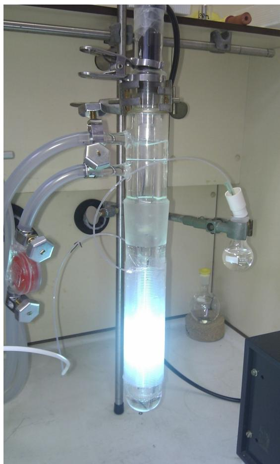
Figure 1: Flow-reactor setup used in the optimization study.
