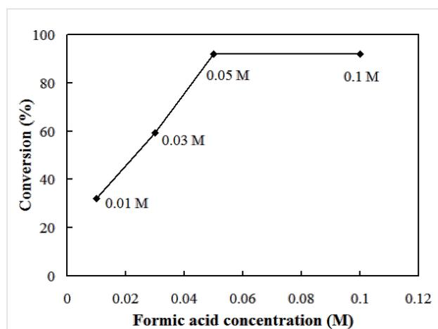
**Figure 5:** Effect of the concentration of formic acid on the conversion of 0.01 M *p*-nitrophenol. The formic acid concentration varied: 0.01 M, 0.03 M, 0.05 M and 0.1 M. Porous-PdO-coated reactor was used at 30 °C, with a residence time of 14.7 s.
