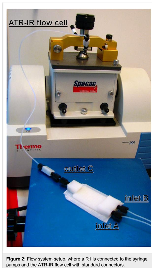
**Figure 2:** Flow system setup, where a R1 is connected to the syringe pumps and the ATR-IR flow cell with standard connectors.
