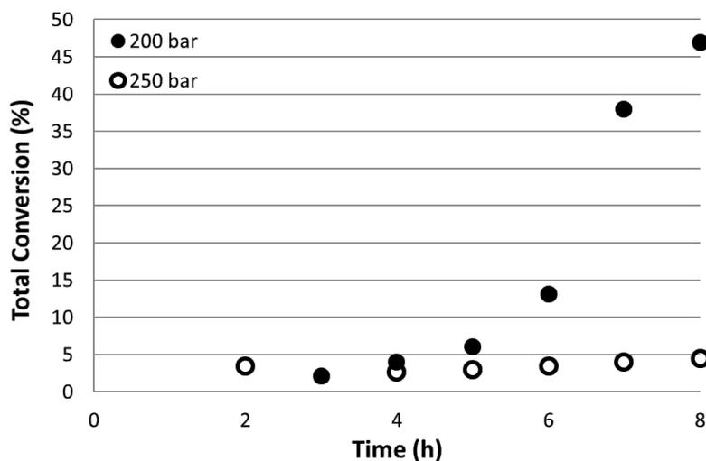
**Figure 5:** Total conversion of 4-iodoanisole as a function of reactor run time at 145 °C and at 200 (●) and 250 (○) bar CO<sub>2</sub> pressure.
