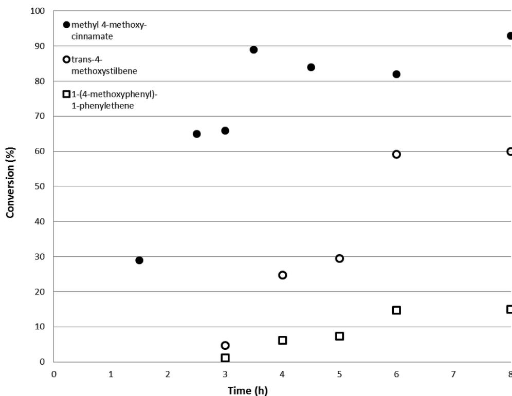
**Figure 6:** Conversion of 4-iodoanisole to methyl 4-methoxycinnamate (●) at 155 °C and 200 bar as a function of reactor run time. The open symbols are the conversions to the different isomeric products for the reaction of 4-iodoanisole with styrene for comparison.
