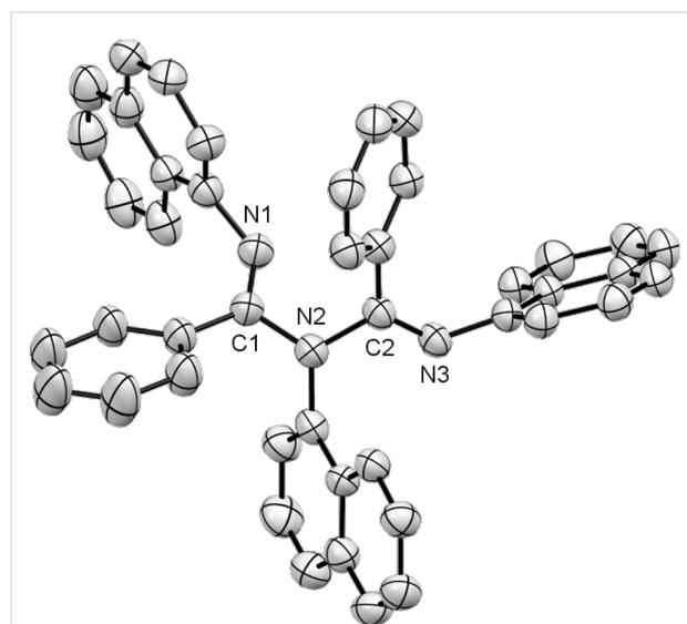
**Figure 3:** ORTEP drawing of **3b**. Thermal ellipsoids are set at 35% probability level. Hydrogen atoms are omitted for clarity. Selected bond lengths [Å] and angles [°] are as follows: C(1)–N(1) 1.273(4), C(1)–N(2) 1.420(4), C(2)–N(2) 1.421(4), C(2)–N(3) 1.278(4), N(1)–C(1)–N(2) 115.3(3), C(1)–N(2)–C(2) 117.0(3), N(2)–C(2)–N(3) 117.8(3).
