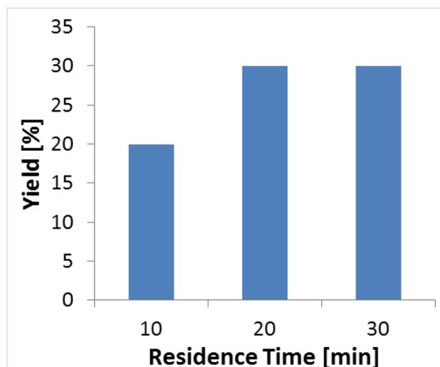
**Figure 6:** Effect of flow rates on yield for immobilized enzymes in a packed bed microreactor (70  $^{\circ}\text{C}$ ). Reaction conditions: Reaction volume (0.250 mL), TA (1.1 mg, specific activity – 0.052 U/mg), temperature (70  $^{\circ}\text{C}$ ).
