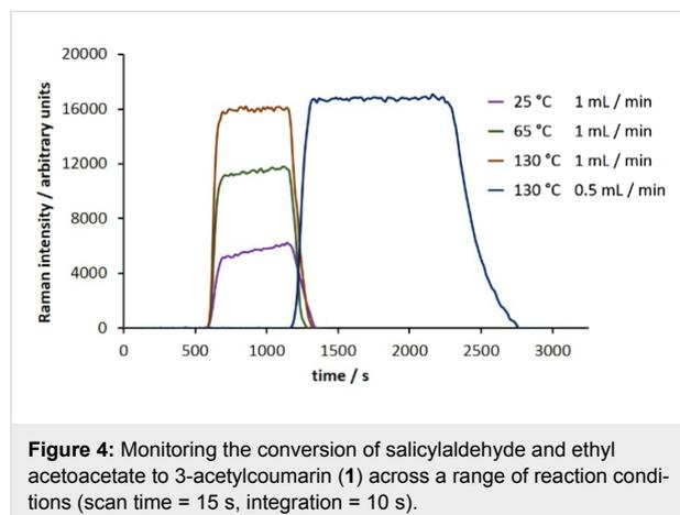
**Figure 4:** Monitoring the conversion of salicylaldehyde and ethyl acetoacetate to 3-acetylcoumarin (**1**) across a range of reaction conditions (scan time = 15 s, integration = 10 s).
