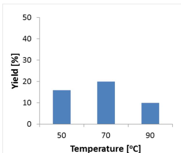
**Figure 5:** Effect of temperature on product yield. Reaction conditions: Reaction volume (0.250 mL), TA (1.1 mg, specific activity – 0.052 U/mg), flow rate (25  $\mu\text{L}/\text{min}$ ). Samples were taken after 30 minutes at the indicated temperature.
