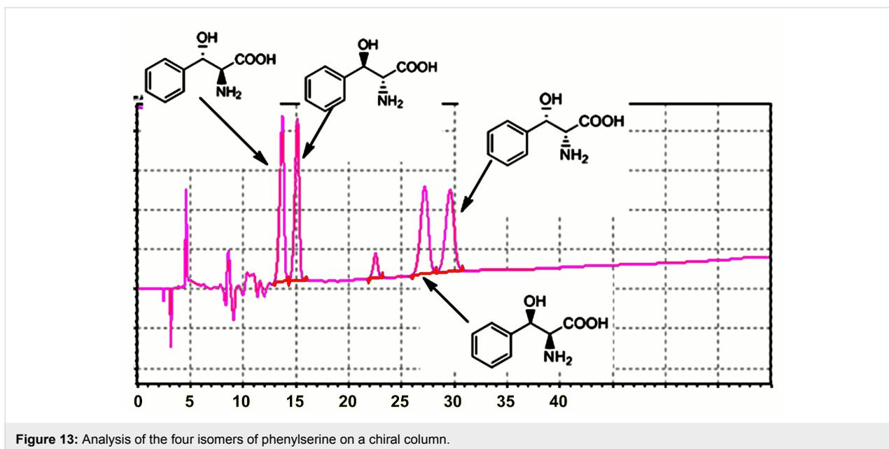
Figure 13: Analysis of the four isomers of phenylserine on a chiral column.
