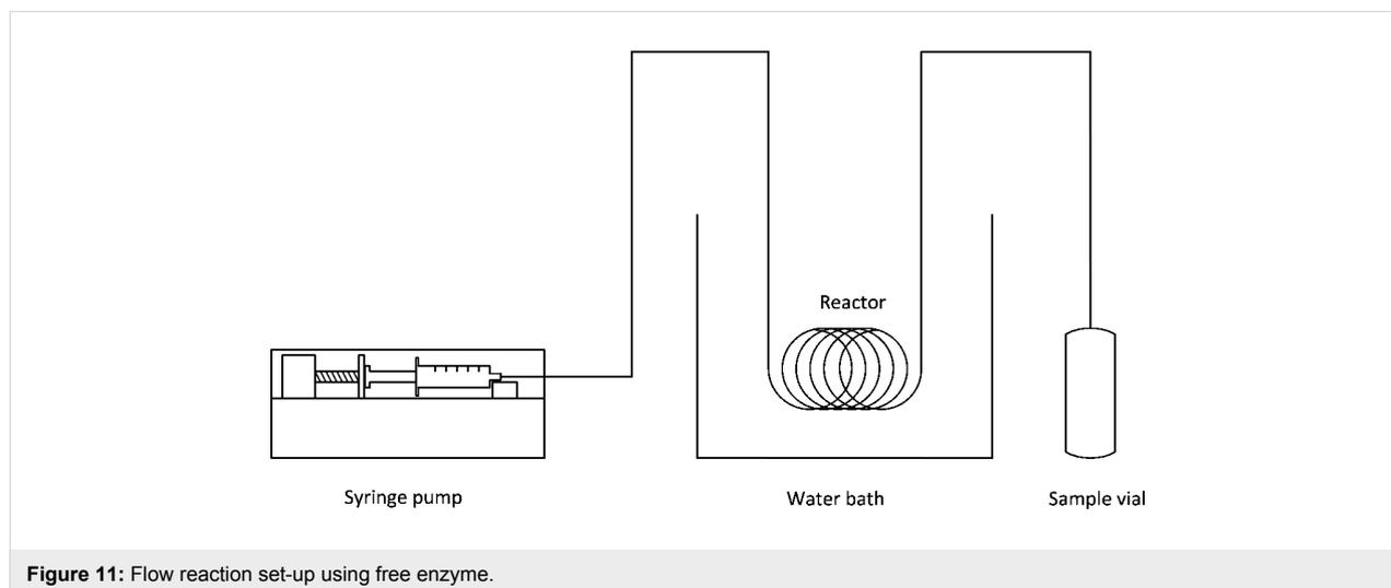
Figure 11: Flow reaction set-up using free enzyme.
