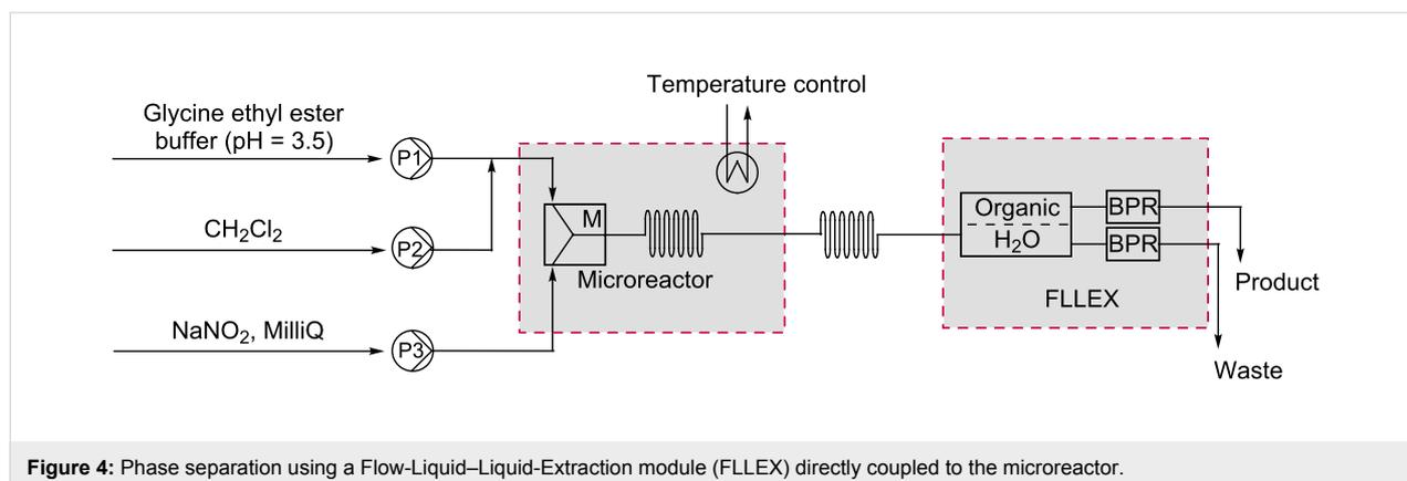
**Figure 4:** Phase separation using a Flow-Liquid-Liquid-Extraction module (FLLEX) directly coupled to the microreactor.
