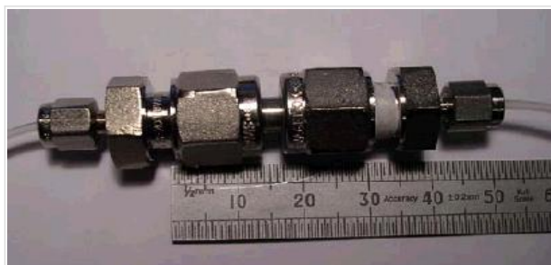
Figure 1: Stainless steel single column flow reactor for discovery scale synthesis.
