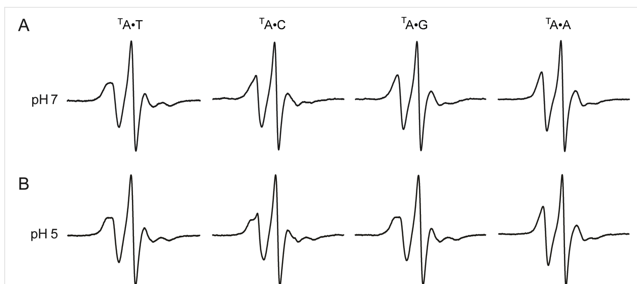
Figure 2: EPR spectra of 14-mer DNA duplexes 5'-d(GACCTCG ^T\text{A} ATCGTG)•5'-d(CACGATYCGAGGTC), (10 mM phosphate, 100 mM NaCl, 0.1 mM Na 2 EDTA, pH 7.0 (A) and 5.0 (B)) at 10 °C, where ^T\text{A} is paired with either Y = T, C, G or A.
