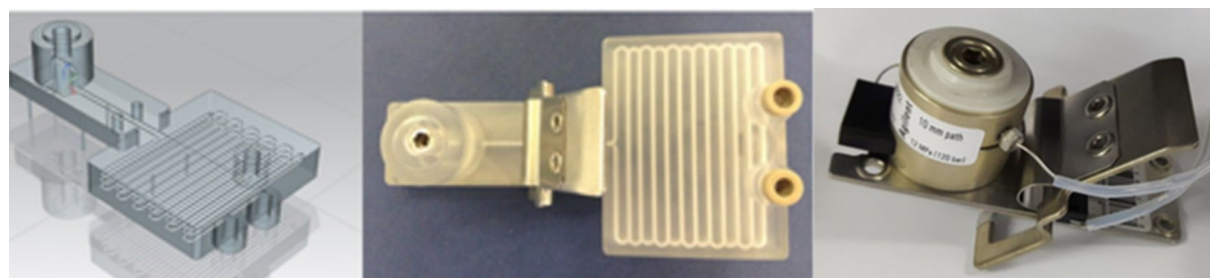
Figure 1: CAD model of SL reactor design RD1 (left), RD1 with attached sprung clip (centre), commercially available Agilent flow cell (right). External dimensions of RD1 are 123 (length) \times 67 (width) \times 42 mm (depth).
