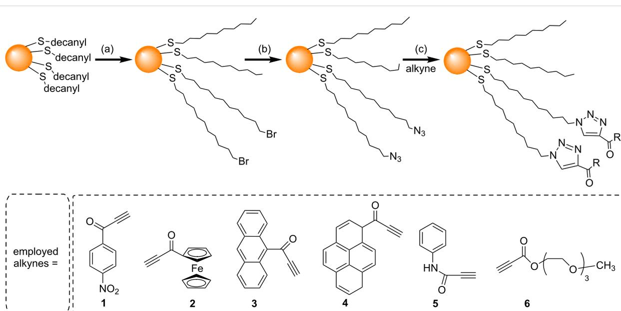
**Scheme 2:** Ligand exchange and NCAAC on an AuNP surface. Reagents and conditions: (a)  $\text{Br}(\text{CH}_2)_{11}\text{SH}$  in DCM, 60 h, rt; (b)  $\text{NaN}_3$ , DCM/DMSO, 48 h; (c) R = propyn-1-one derivatives, 24–96 h in dioxane, or 1:1 hexane/dioxane [45].
