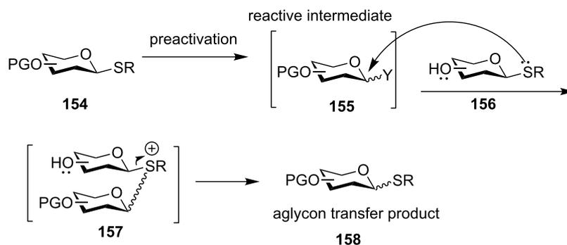
**Scheme 23:** Aglycon transfer from a thioglycosyl acceptor to an activated donor can occur during preactivation-based glycosylation reaction. This side reaction can be suppressed by tuning the reactivity of acceptor aglycon or manipulating the reaction temperature.
