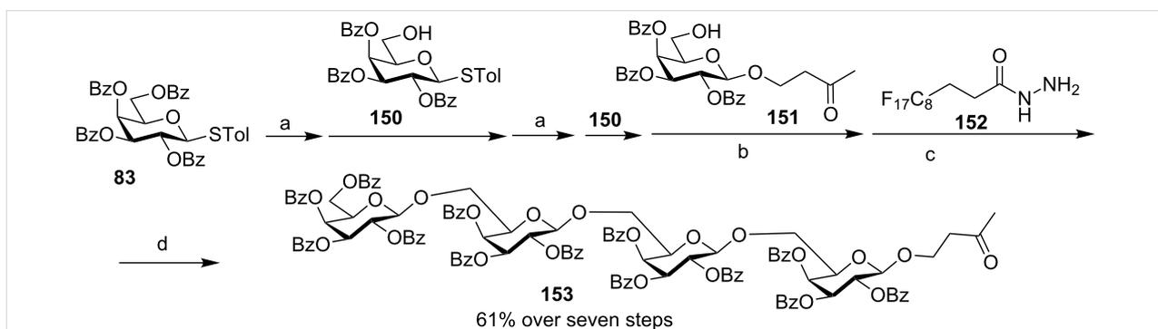
**Scheme 22:** Synthesis of tetrasaccharide **153**. Reagents and conditions: (a) AgOTf, *p*-TolSCL,  $\text{CH}_2\text{Cl}_2$ ,  $-78^\circ\text{C}$ ; then **150**; (b) AgOTf, *p*-TolSCL,  $\text{CH}_2\text{Cl}_2$ , **150**,  $-78^\circ\text{C}$  to rt; (c)  $\text{CH}_2\text{Cl}_2/\text{MeOH}$ , then F-SPE; (d) acetone/trifluoroacetic acid, then F-SPE.
