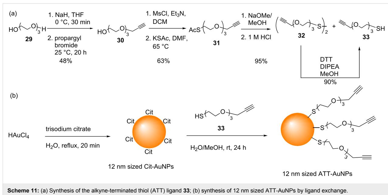
**Scheme 11:** (a) Synthesis of the alkyne-terminated thiol (ATT) ligand **33**; (b) synthesis of 12 nm sized ATT-AuNPs by ligand exchange.
