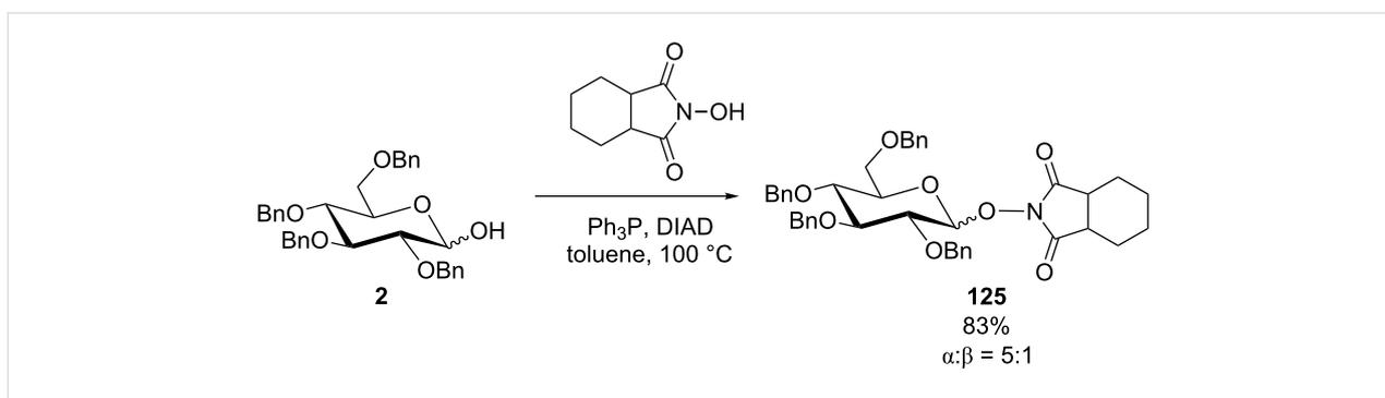
**Scheme 26:** Synthesis of carbohydrates with an alkoxyamine bond [114].
