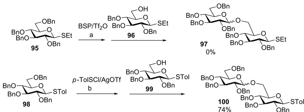
**Scheme 17:** Comparison of the BSP/Tf<sub>2</sub>O and *p*-TolSCl/AgOTf promoter systems in facilitating the preactivation-based thioglycoside glycosylation. Reagents and conditions: (a) BSP, Tf<sub>2</sub>O, CH<sub>2</sub>Cl<sub>2</sub>, TTBP, -60 °C; then **96**, and triethyl phosphite; (b) *p*-TolSCl/AgOTf, -60 °C; then **99**.
