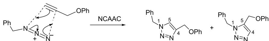
**Scheme 1:** The non-catalysed azide–alkyne Huisgen cycloaddition (NCAAC) between an organic azide (1,3-dipole) and an alkyne (dipolarophile) resulting in the formation of regioisomeric triazole products.
