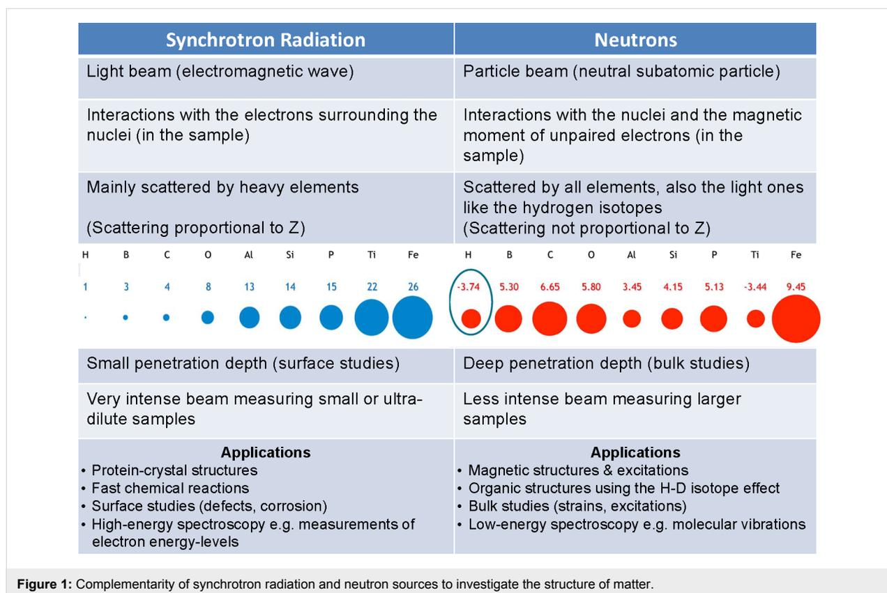
**Figure 1:** Complementarity of synchrotron radiation and neutron sources to investigate the structure of matter.
