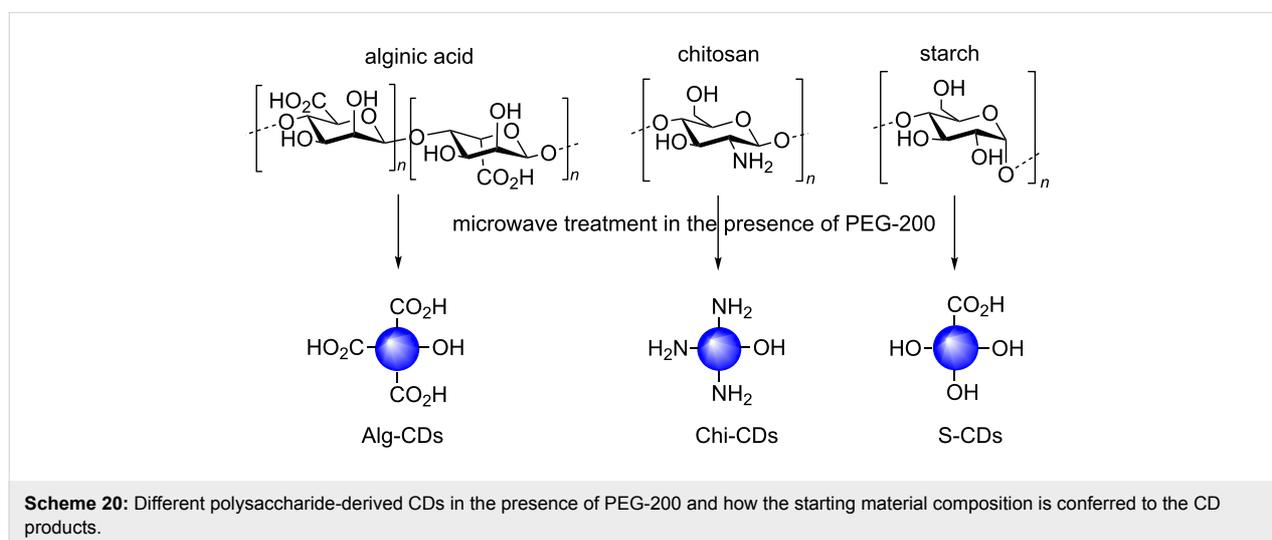
**Scheme 20:** Different polysaccharide-derived CDs in the presence of PEG-200 and how the starting material composition is conferred to the CD products.
