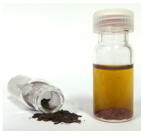
Figure 3: a) Custom-machined copper vessel and zirconia balls used to perform CuAAC reactions (showing: upper half of vessel with PTFE insert (front), pristine \text{ZrO}_2 ball, used \text{ZrO}_2 ball and lower half of vessel showing deformation of the metal). b) Crude solid ball mill click reaction mixture after removal from copper vessel (left) and during extraction of pure product with DMSO (right).
