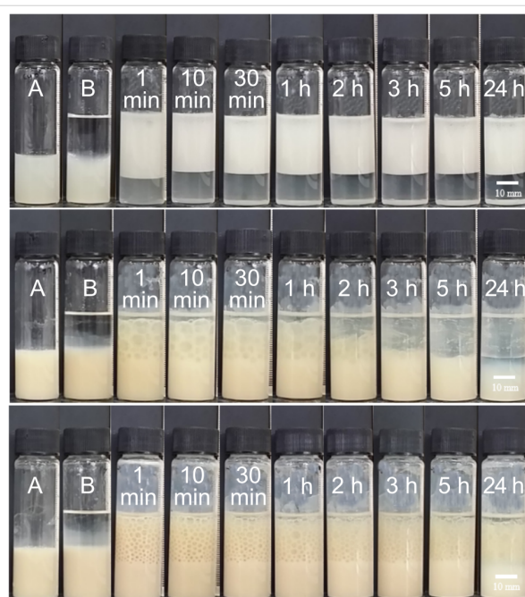
Figure 4: Photos of vessels containing cyclohexane-in-water emulsions stabilised by particles of \text{Ce}_{0.495}\text{Sn}_{0.495}\text{Pd}_{0.01}\text{O}_{2-\delta} at concentrations in water of 0.03 wt % (upper), 0.30 wt % (middle) and 1.0 wt % (lower) at different times since preparation. A is the aqueous dispersion of particles, B is after addition of oil but before emulsification.
