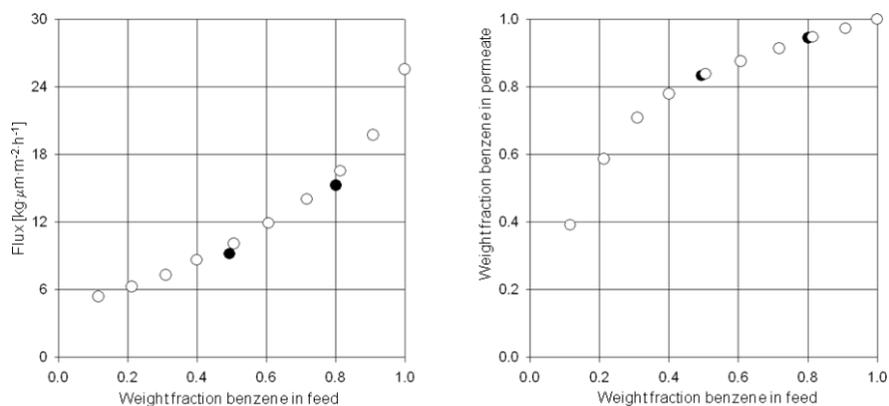
**Figure 10:** Pervaporation results for the 6FDA-6FpDA/6FDA-4MPD/6FDA-DABA 3:1:1 copolyimide cross-linked with ethylene glycol (first run (●) and second run (○) using benzene/cyclohexane mixtures at 60 °C and a permeate pressure of 10–20 mbar (data taken from [28]).
