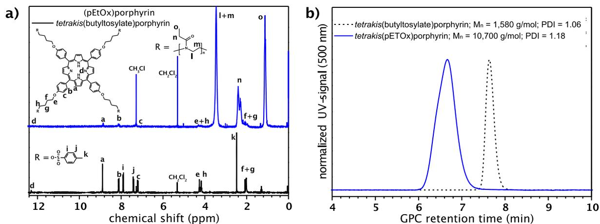
**Figure 9:** a)  $^1\text{H}$  NMR spectra (in  $\text{CDCl}_3$ ) of the porphyrin initiator TetraTos-B (bottom) and star-pETox (top). b) SEC traces of TetraTos-B and star-PETox (in  $\text{CHCl}_3\text{:NEt}_3\text{:2-PrOH}$ ; UV-detector at 500 nm).
