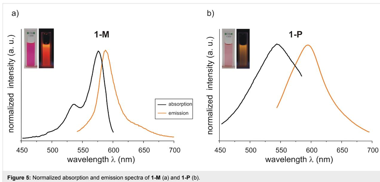
**Figure 5:** Normalized absorption and emission spectra of **1-M** (a) and **1-P** (b).
