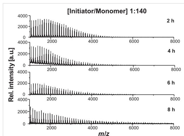
**Figure 4:** MALDI-TOF MS of P2VP obtained for polymerizations stopped after 2, 4, 6, and 8 h. The samples were prepared by the dried droplet method dissolving the polymer, DT, and KOTf in THF. To gain representative information, the spot was probed at several locations and 100 spectra were accumulated.
