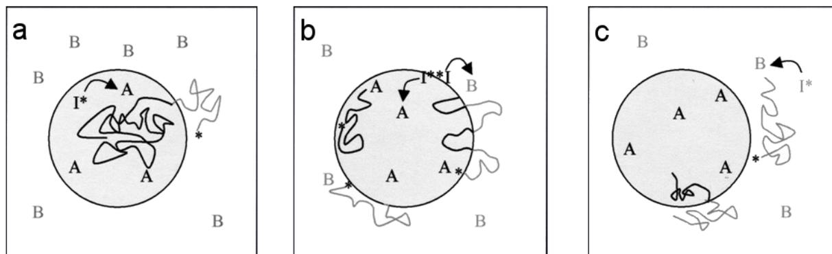
**Figure 1:** Copolymerization of 2 monomers A and B with different polarities in direct miniemulsions with the decomposed initiators  $I^*$  which are **a:** oil-soluble, **b:** surface active, **c:** water-soluble (reproduced with permission from [27]. Copyright (2002) Wiley-VCH Verlag GmbH & Co, KGaA).
