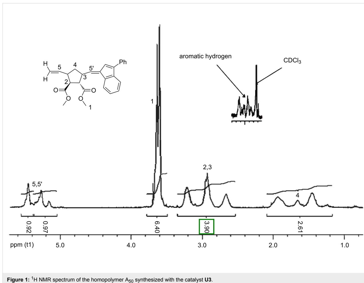
Figure 1:  $^1\text{H}$  NMR spectrum of the homopolymer  $\text{A}_{50}$  synthesized with the catalyst **U3**.
