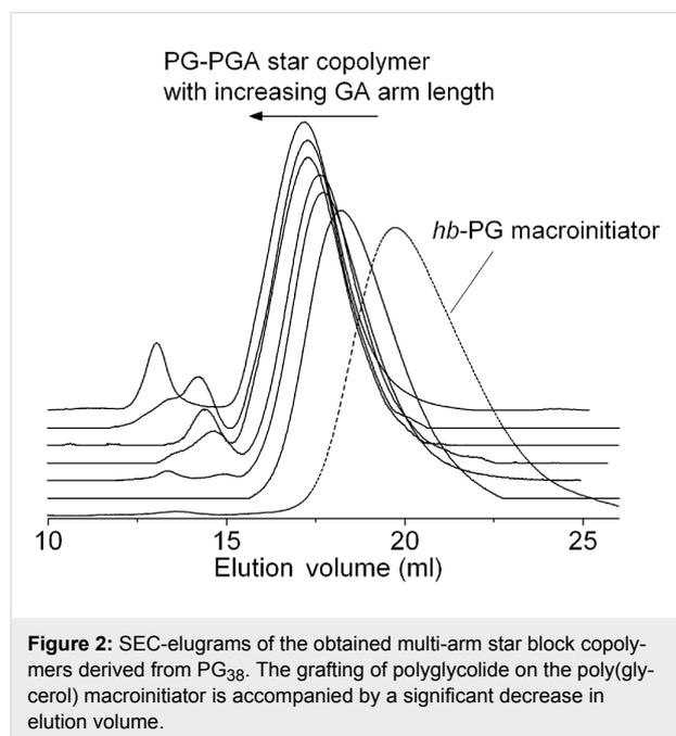
**Figure 2:** SEC-elugrams of the obtained multi-arm star block copolymers derived from  $\text{PG}_{38}$ . The grafting of polyglycolide on the poly(glycerol) macroinitiator is accompanied by a significant decrease in elution volume.
