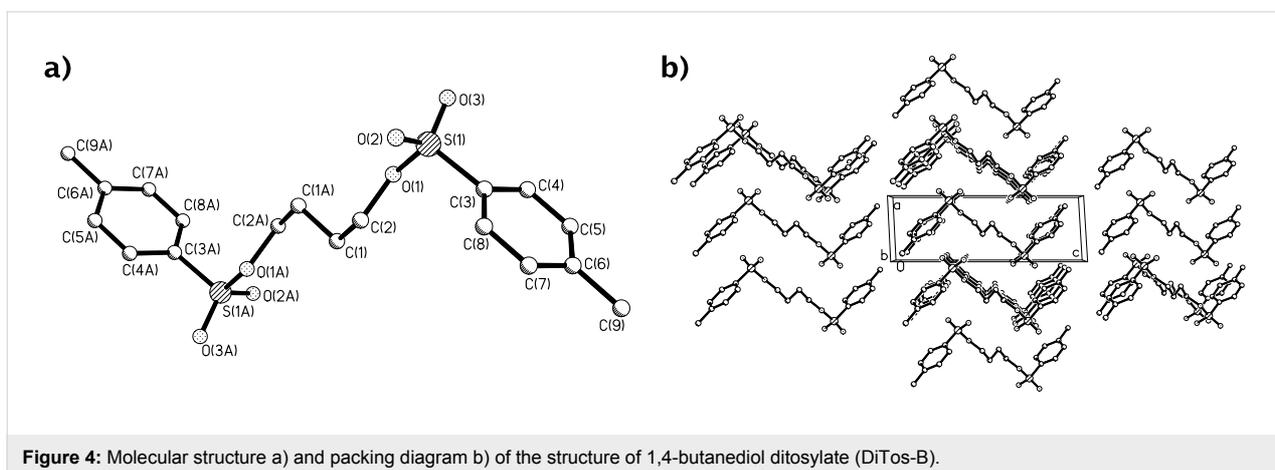
Figure 4: Molecular structure a) and packing diagram b) of the structure of 1,4-butanediol ditosylate (DiTos-B).
