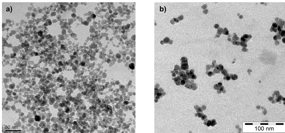
**Figure 2:** TEM images of a)  $\text{Fe}_3\text{O}_4$  nanoparticles electrostatically stabilized by citric acid; b)  $\text{Fe}_3\text{O}_4@P(\text{M}_{100})$  nanoparticles after surface-initiated ATRP.
