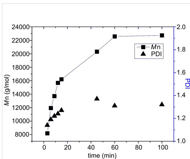
**Figure 6:**  $M_n$  vs. time ( $t$ ) kinetic plot and  $M_w/M_n$  (PDI) of the polymerization of monomer T 9 with catalyst U3;  $[9]/[U3] = 50/1$ .
