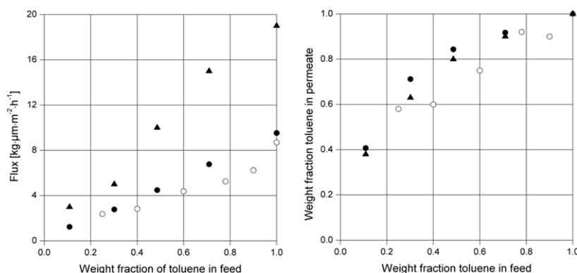
**Figure 12:** Pervaporation results for conditioned 6FDA-4MPD/6FDA-DABA 4:1 copolyimide membranes, 100% cross-linked with 1,4-butanediol (●) and 10% cross-linked with zircon(IV) acetylacetonate (○) and non cross-linked (▲) using a toluene/cyclohexane mixture at 60 °C. Permeate pressure was kept between 20 and 25 mbar.
