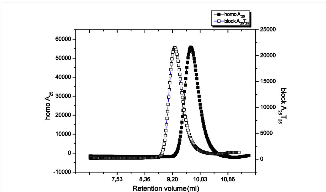
**Figure 7:** GPC trace of the block copolymer A<sub>25</sub>T<sub>25</sub> synthesized with catalyst U3.
