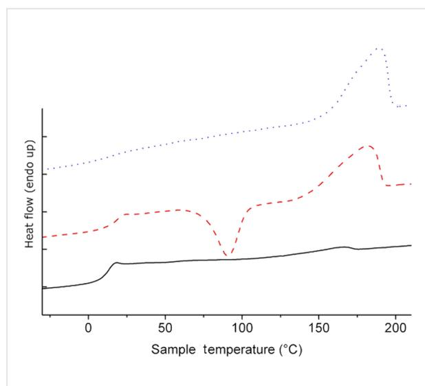
**Figure 6:** DSC heating traces (second heating run at 20 °C/min) for *hb*- $\text{PG}_{38}$ -*b*- $\text{GA}_4$  (bottom), *hb*- $\text{PG}_{38}$ -*b*- $\text{GA}_8$  (middle) and *hb*- $\text{PG}_{38}$ -*b*- $\text{GA}_{12}$  (top), reflecting the increasing influence of polyglycolide chain length.
