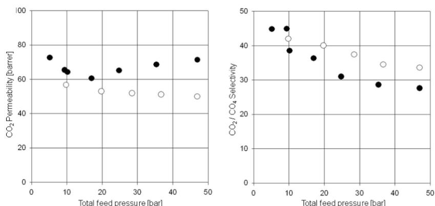
**Figure 15:** CO<sub>2</sub>/CH<sub>4</sub> separation characteristics for the 6FDA-4MPD/6FDA-DABA 4:1 copolyimide ionic cross-linked with aluminium acetylacetonate (●) and covalently cross-linked with ethylene glycol (○) at 35 °C using a 50:50 CO<sub>2</sub>/CH<sub>4</sub> feed gas mixture.
