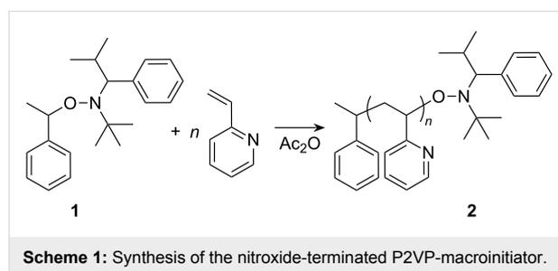
**Scheme 1:** Synthesis of the nitroxide-terminated P2VP-macroinitiator.
