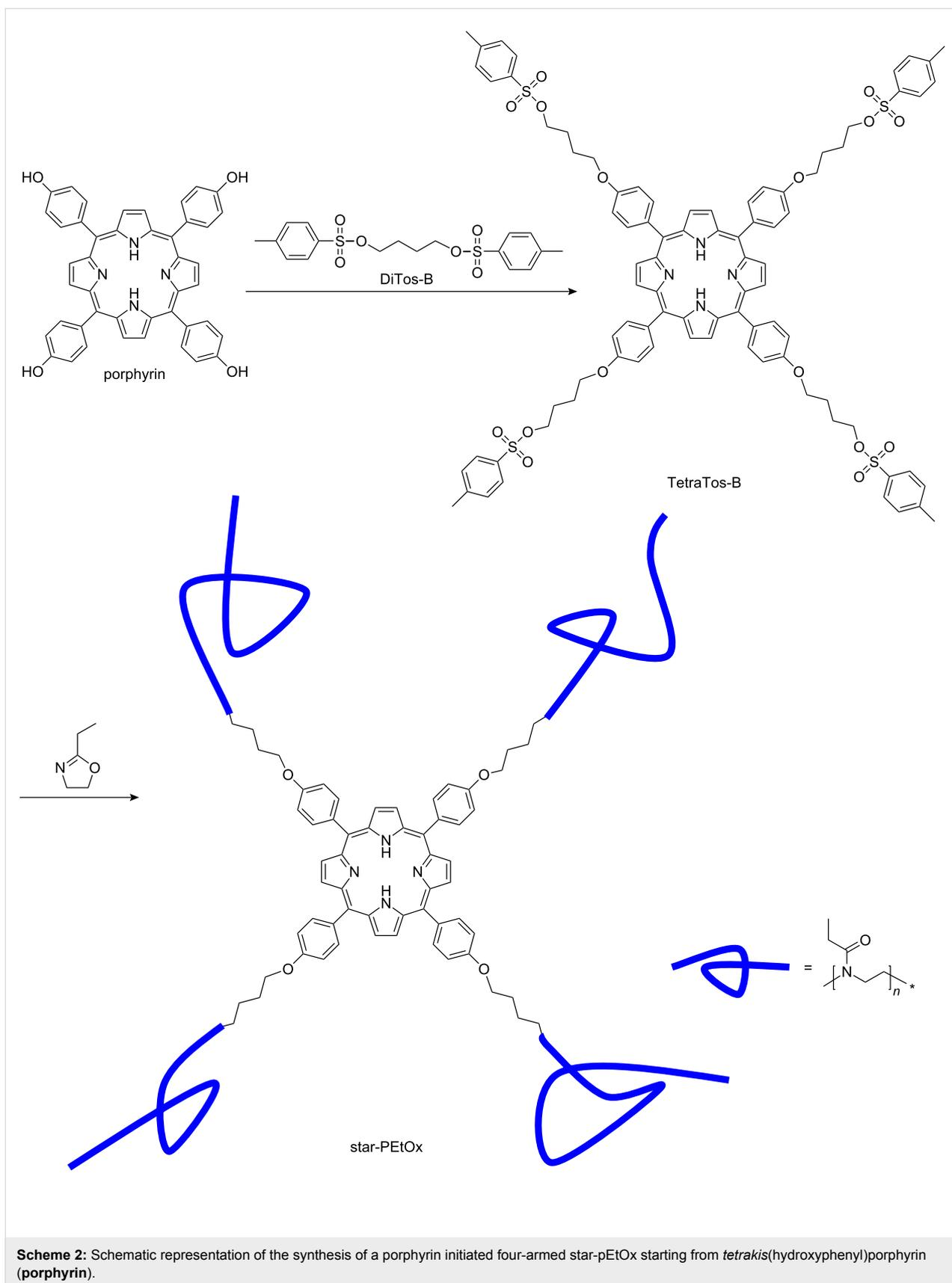
**Scheme 2:** Schematic representation of the synthesis of a porphyrin initiated four-armed star-pEtOx starting from *tetrakis*(hydroxyphenyl)porphyrin (**porphyrin**).
