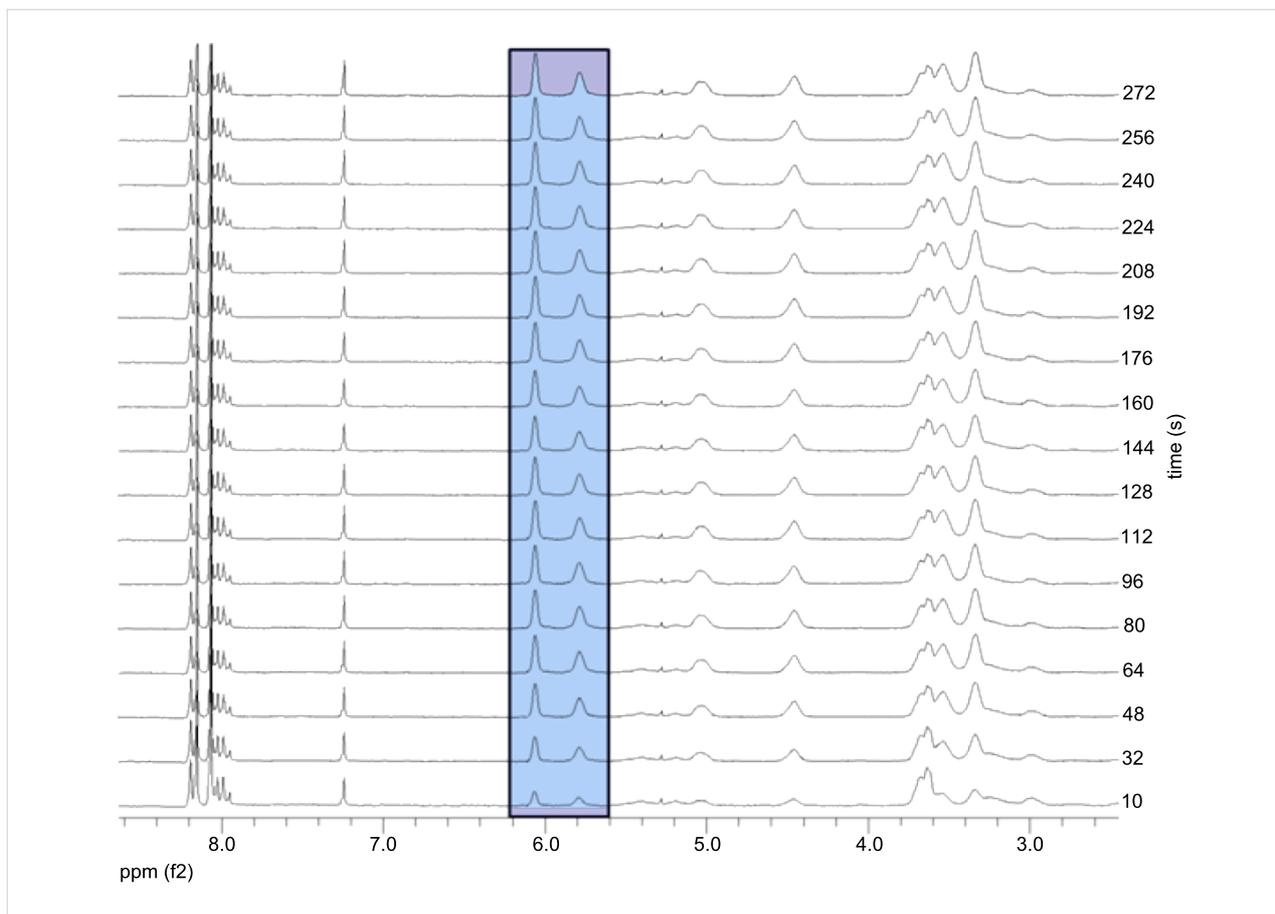
Figure 3: Kinetic progress monitored via  $^1\text{H}$  NMR spectroscopy of the polymerization of monomer **A 7** with catalyst **U1**;  $[\text{7}]/[\text{U1}] = 20/1$ .
