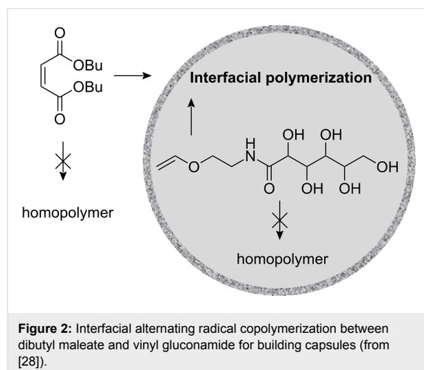
**Figure 2:** Interfacial alternating radical copolymerization between dibutyl maleate and vinyl gluconamide for building capsules (from [28]).
