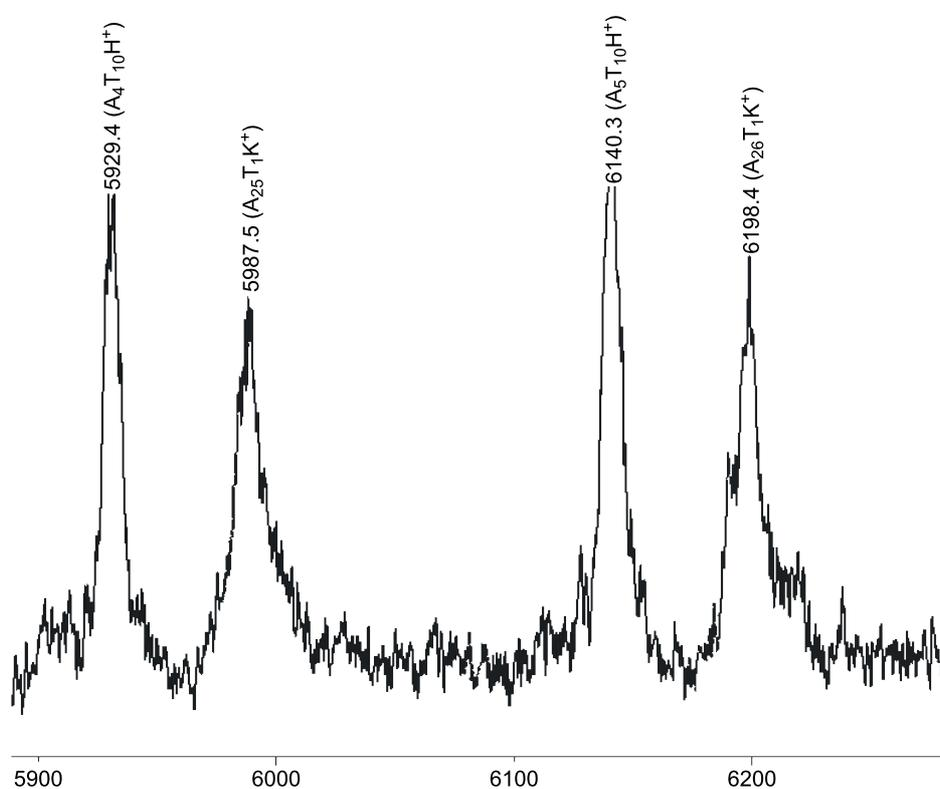
Figure 11: MALDI-TOF mass spectrum of BCP-A<sub>25</sub>T<sub>25</sub> synthesized with catalyst U3.
