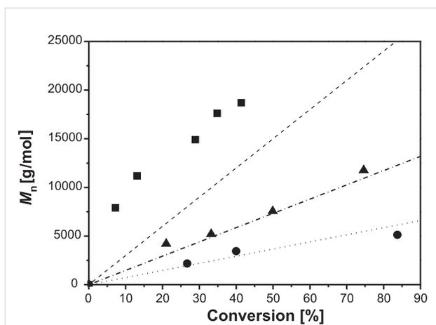
**Figure 3:** Plot of number average molecular weight vs conversion for the homopolymerization of 2VP at 110 °C with different molar ratios of [initiator]/[monomer] ■ 1:210, ▲ 1:140, ● 1:70. The dashed lines describe the theoretical behavior.
