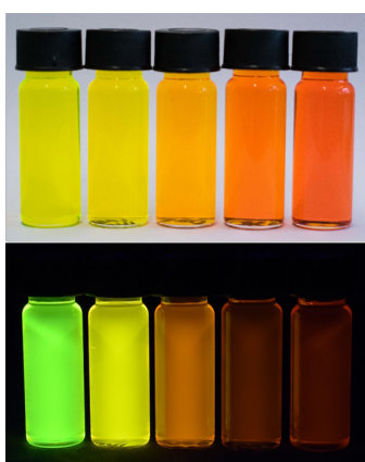
Figure 11: Absorption (top) and fluorescence (bottom) of compound 6c with variable solvent polarity (left to the right: toluene, ethyl acetate, acetone, DMF and DMSO, c(\mathbf{6c}) = 10^{-4} M; \lambda_{exc} = 365 nm, handheld UV lamp).
