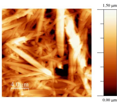
**Figure SI3.** AFM image of an OFET device fabricated with OTS/PFBT SAMs and compound **1** in *o*-dichlorobenzene.
