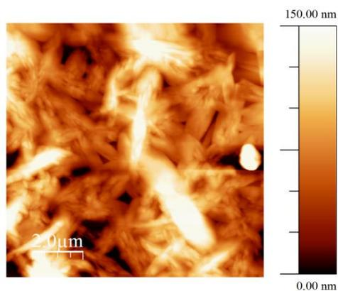
**Figure SI4.** AFM image of an OFET device fabricated with OTS/PFBT SAMs and compound **1** in chloroform.
