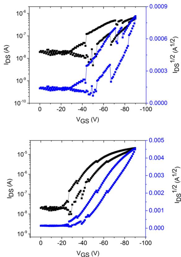
**Figure SI2.** Output characteristics of OFETs fabricated using compound **2** in  $\text{CHCl}_3$  with OTS (top) and PFBT/OTS (bottom) as self-assembled monolayers.
