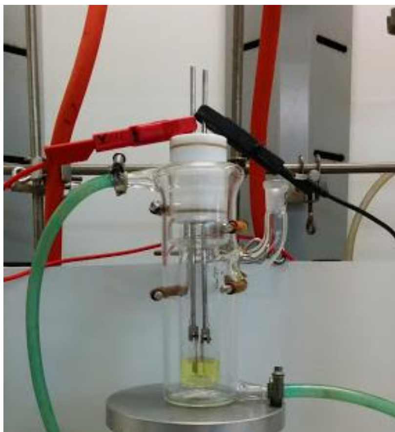
Figure 1: Schematic construction of the undivided electrolysis cell (top), photo of the undivided electrolysis cell (bottom).
