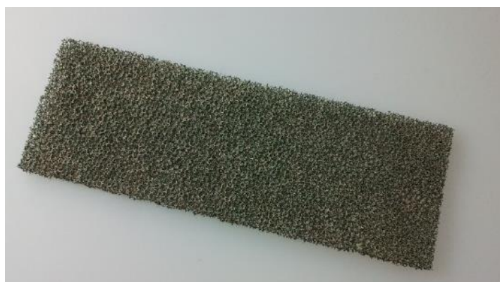
Figure S1: Ni foam electrode applied for the electrochemical degradation of lignin.
