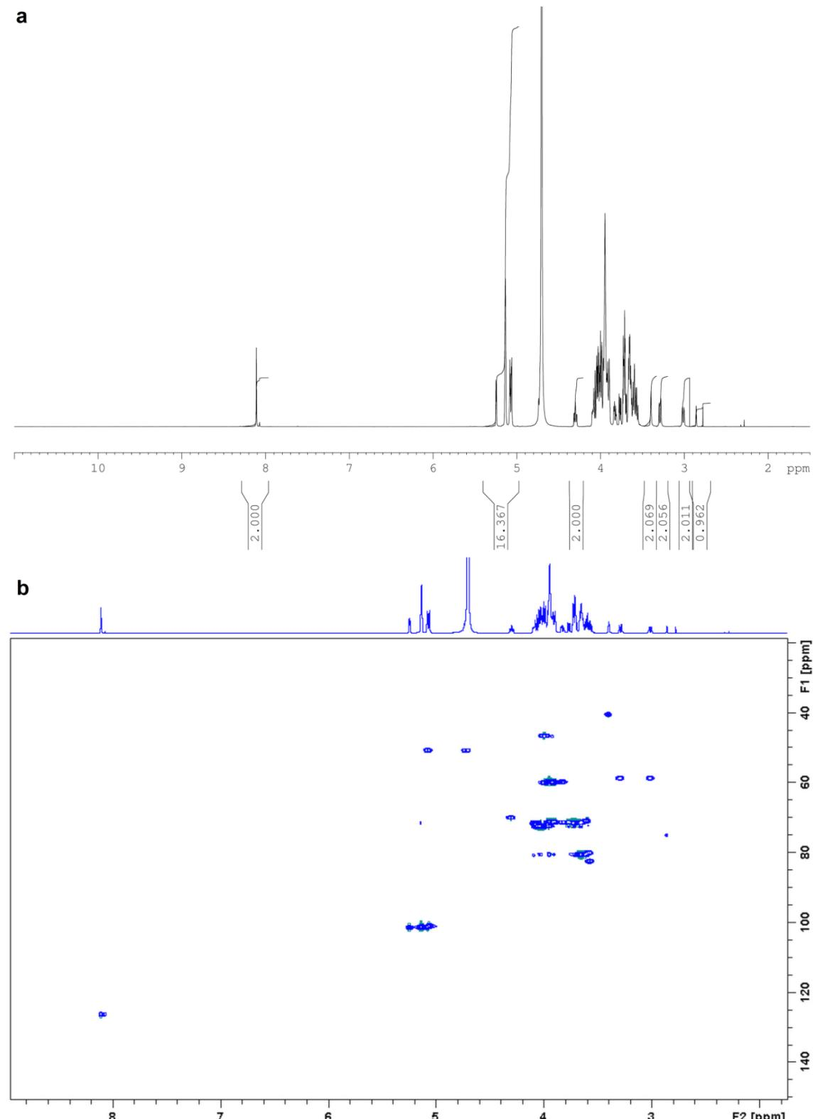
$^1\text{H}$  NMR (a) and  $^{13}\text{C}$  HSQC (b) spectra of the  $\beta$ -CD dimer. Successful CuAAC is evident from the signal resonating at 8.1 ppm (triazole). Furthermore, a signal from the terminal alkyne is present at 2.9 ppm.
