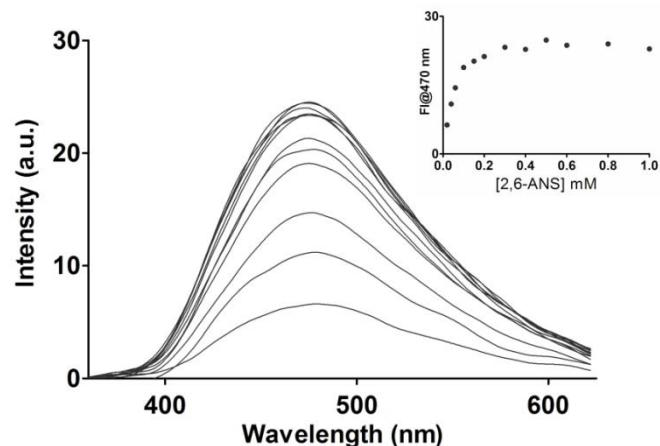
Titration series of 2,6-ANS (0.02–1 mM) recorded by TIRF spectroscopy on a clean and unmodified quartz slide.
