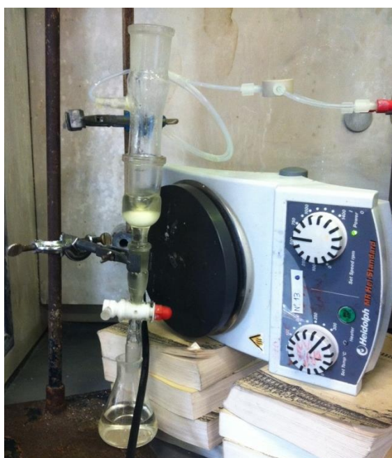
Figure S2: Set-up of continuous-flow apparatus for in-line extraction.
