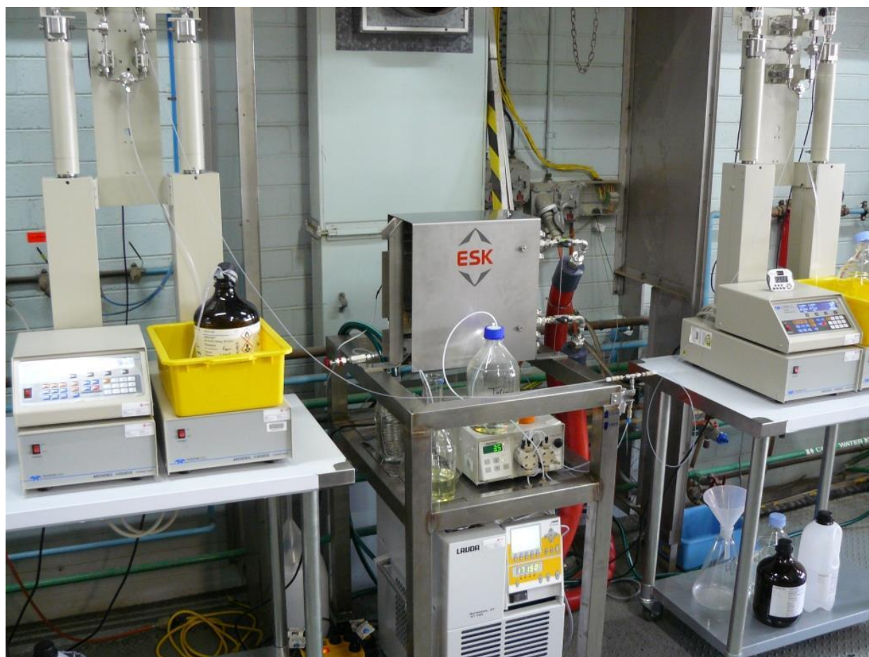
Figure S2: Experimental set-up for the Diels–Alder reaction of myrcene and acrylic acid in a Chemtrix Plantrix ® MR260 flow reactor.
