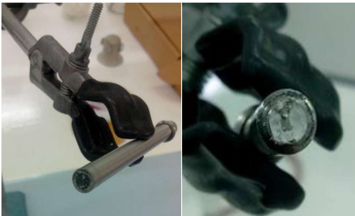
Figure S5: Images of a blocked 6 mm i.d. reactor tube of a tubular stainless steel reactor (with static mixer inserts); the white material is poly(acrylic acid-co-myrcene).
