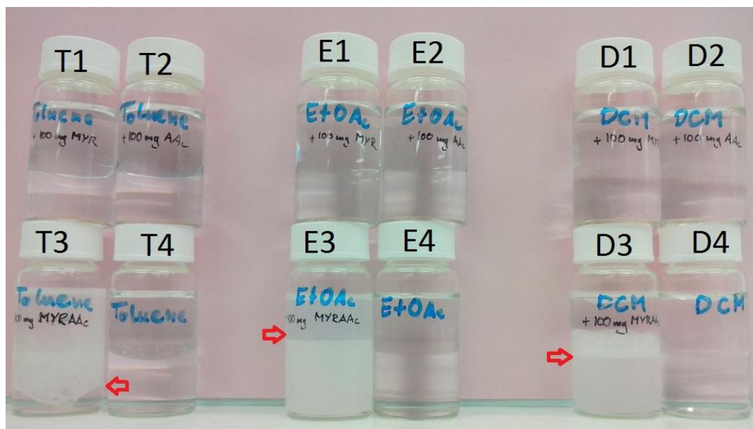
Figure S6: Image of a series of mixtures of water and an organic solvent, some containing starting material and others Diels–Alder adduct. The image was taken 18 min after agitation, the red arrows indicate the forming phase boundary between two emulsion layers for the samples containing Diels–Alder adduct
