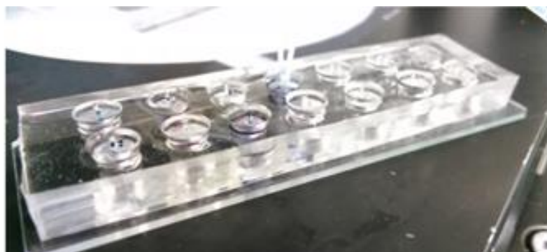
Figure S2.2.1: Off-Chip Droplet Incubation Reservoirs. Home-made inlet-outlet device fabricated by bonding two parts of PDMS and punching two 0.75 mm holes. 1/32'' OD PTFE tubing was used to connect the reservoir to the microfluidic chip.
