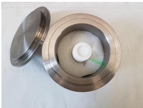
Figure S1: 25 mL glass jar milled in a planetary system using a 500 mL stainless steel jar as host cavity.
