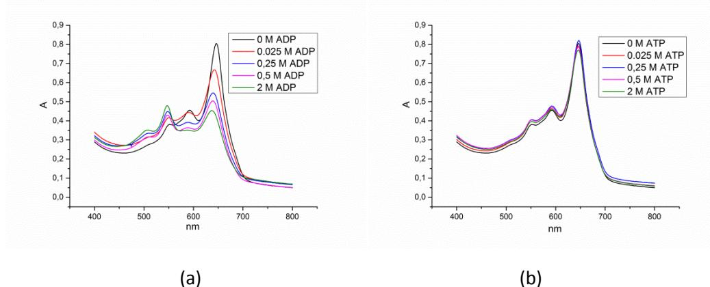
**Figure S4:** UV spectra of the AEPCDA-**10b** polydiacetylene vesicles in the absence or presence of ADP(a) or ATP (b); C(AEPCDA) = 0.2 mM, C (**10 b**)= 0.1 mM (a) C (nucleotide) = 0.025, 0.25, 0.5, 2 mM in 10 mM MES buffer, pH 6.5.
