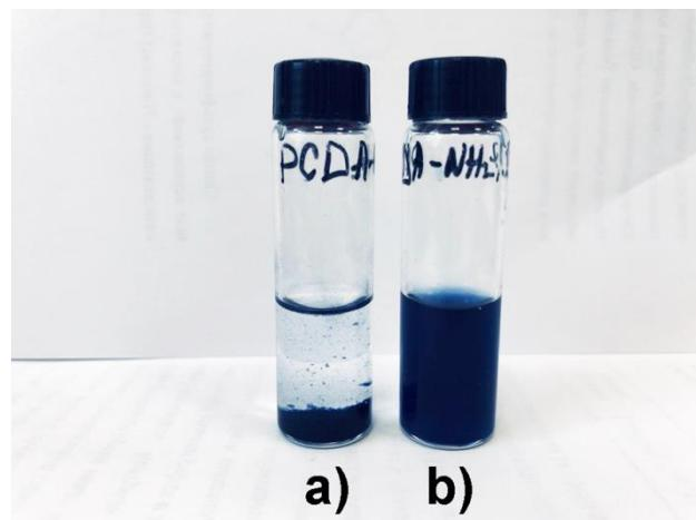
**Figure S3:** Photography of AEPCDA (a) and AEPCDA-**10b** (b) polydiacetylene vesicles after standing for 2 hours; C(AEPCDA) = 0.2 mM, C (**10b**)= 0.1 mM in 10 mM MES buffer, pH 6.5.
