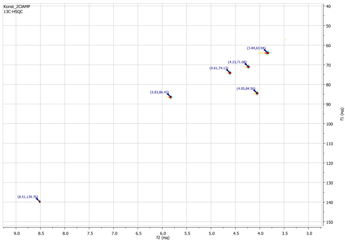
Figure S11. ^1\text{H} , ^{13}\text{C} -HSQC spectrum of 2-Cl-AMP
